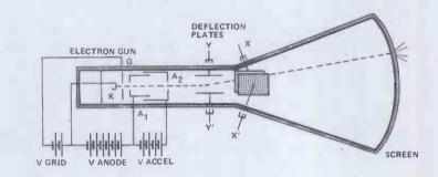
Figure 1. The internal structure of a typical cathode ray tube.
