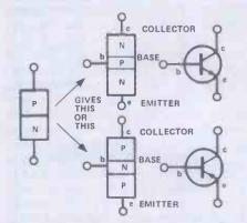
Figure 1. Three-layer device is either a pnp or npn transistor (with corresponding circuit symbol)
