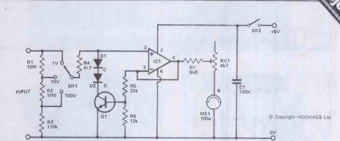
Figure 1. Circuit diagram of the High-Impedance Voltmeter
