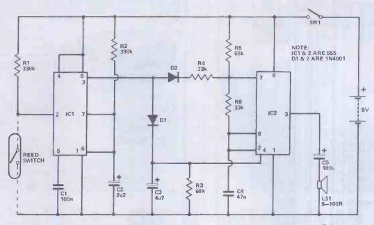
Figure 1. The HE Two-Tone Train Horn circuit diagram.
