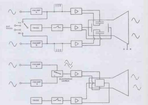
Figure 5. Dual-trace oscilloscopes can be implemented in two ways: using a dual beam cathode ray tube or using a single beam tube and electronic switching of the trace. The block diagram at the top is of a Philips model 3232 and is typical of dual-beam types. The block diagram at the bottom shows the electronic switching technique of obtaining dualtrace operation with a single beam cathode ray tube.
