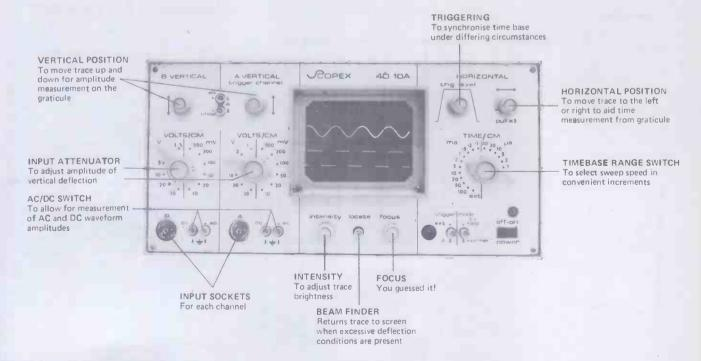
A typical oscilloscope front panel layout, showing the positions of the major controls.
