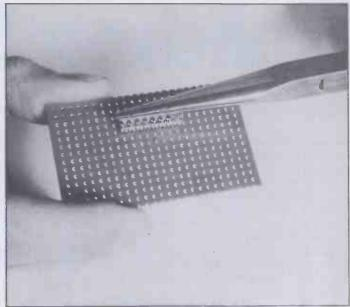
Figure 5. Break off the top common connector using your snipe-nosed pliers. This leaves one side of a ready-made IC socket.
