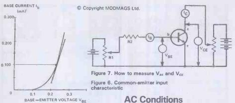
and so we say that the current gain is 50. This current gain is most properly referred to as  $h_{FE}$ . Thus:
