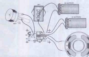
Figure 2. Overlay and connection details — use this if you build the circuit on PCB.
