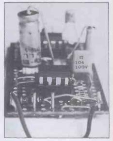
Figure 6. PCB pins are useful to make off-board connections.
