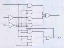
Figure 6.4 Circultry for a full adder. Inputs are the bits to be added, plus a carry from the previous stage: ouputs are the usual sum and carry bits
