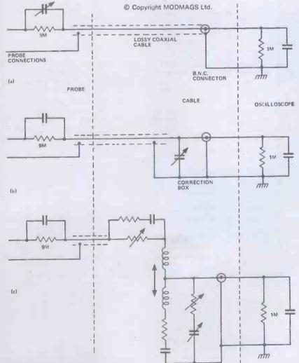
Figure 4. Schematic of attenuator probes (a) simplest concept (b) capacitive loading to extend bandwidth (c) inductive.
