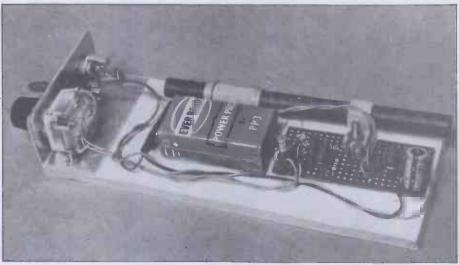
By mounting the project on a suitable board it can be carefully inserted into a case — such as the one we used for a Keystone camera
