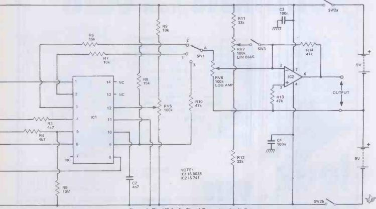
Figure 1. The HE Audio Signal Generator circuit diagram.
