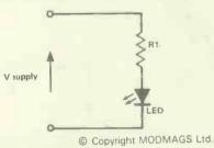
Figure 4. An LED in circuit
