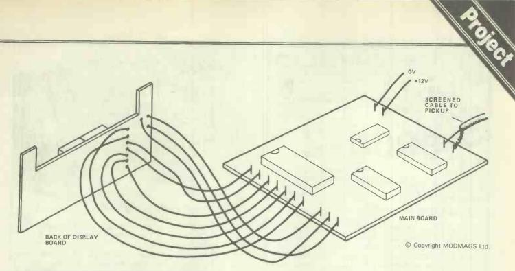
Figure 1. Connection details of the two boards of the Speedo
