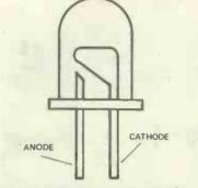
Figure 5. By holding the LED up to a bright light the junction can be seen
