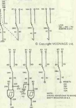
Fig. 5.14 The SIPO register connections. Once more, this shows the additions to the circuit in Fig. 5.9, with previous additions removed. This also restores the switches to normal operation for the next set of operations to be described next month
