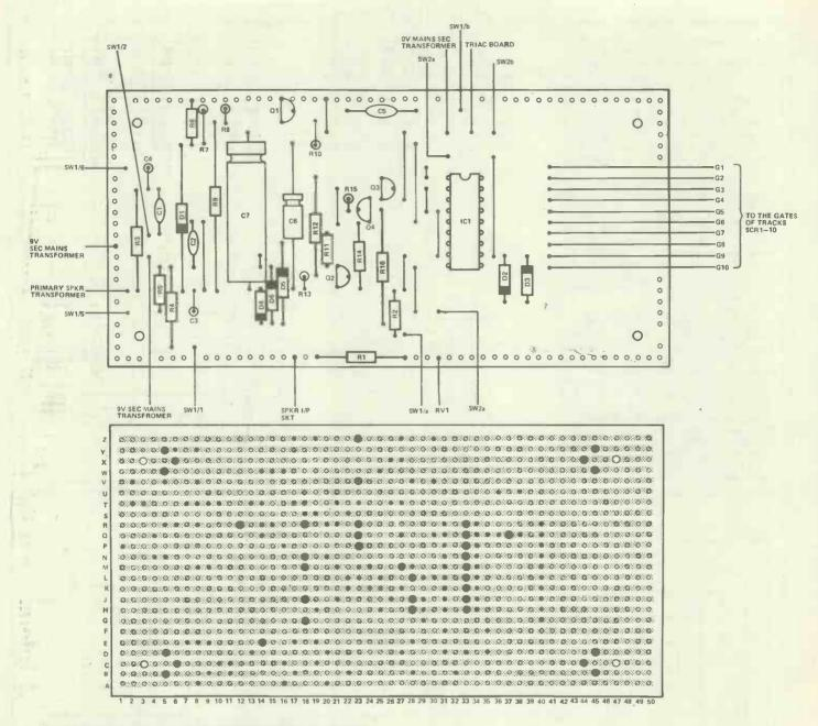
Figure 5. Veroboard layout and underside view showing track breaks
