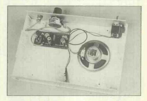
case also helps to avoid stray pick up of mains hum, etc, but a plastic one like we used is satisfactory for most purposes. The input leads and speaker leads should be kept reasonably well separated so that stray feedback is avoided.
