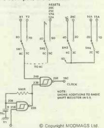
Figure 5.13 Connections for a PISO register. The connections shown in Fig. 5.11 are removed: the diagram shows the additions to the basic circuit in Fig. 5.9
