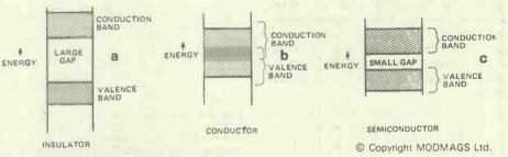
Figure 1. Conduction bands for a) insulators (well separated), b) metal (very close) and c) semiconductors (small gap)
