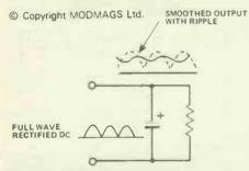
Figure 8. Action of a capacitor in smoothing full-wave rectified DC
