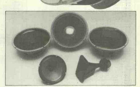
creating an alternating pattern of highand low-pressure waves. The idea has been refined and improved upon mechanically by exchanging the flat surface for a shallow cone supported in a circular metal frame. We all know this as our old friend the loudspeaker:
