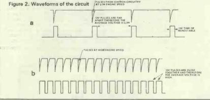
also be seen from this diagram that the average voltage at the output of IC1 will be at a maximum when the pulses are close together and at a minimum when the pulses are far apart. Consequently, as the RPM rate goes up so does the average output voltage. The resistor/ capacitor combination R3, 4 and C4 smooths out the voltage so that a steady DC voltage, which changes only with engine speed, is obtained across C4.
