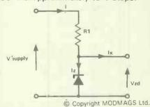
Figure 3. Typical circuit using a zener diode
