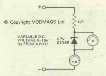
Figure 12. Circuit to demonstrate action of a zener diode
