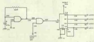
Figure 5.3 A clock-pulse oscillator driving the decade counter through a gate. The outputs of the counter are taken to LEDs © Copyright MODMAGS Ltd.
