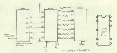
Figure 5.5 Counter-decoder-display circuit. Connections to the 74LS90 counter are the same as they were in Fig. 5.3, but the outputs Qa to Qd are connected to the decoder inputs, and the decoder outputs are connected through 470R resistors to the display
