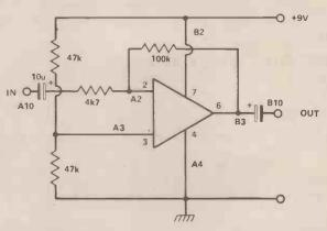
Fig. 3.16 Microphone booster circuits (a) dual supply, (b) single supply.
