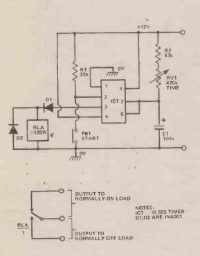
Fig. 1. A simple 6-second to 60-second timer circuit.
