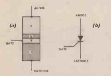
Fig. 1. Four-layer arrangement (a) and the thyristor symbol (b).
