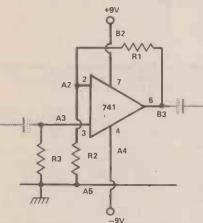
Fig. 3.7 The follower-with-gain. The (dotted) capacitors will be needed if the circuit is to be connected to any points which are not at earth voltage.
