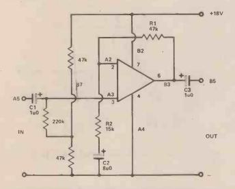
Fig. 3.8 Single-supply version of the follower-with-gain. C2 is needed to prevent the voltage at A2 from being reduced by the potential divider circuit, R1, R2.
