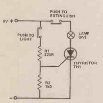
Fig. 6. Simple low-voltage light-switch circuit.
