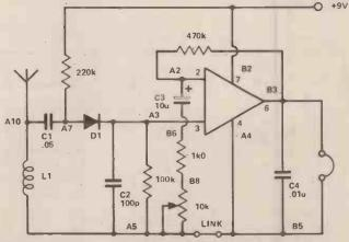
Fig. 3.19 A simple radio circuit using a single voltage supply.
