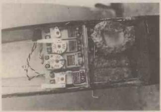
Installation of servos in a typical R/C aircraft. These operate rudder/steerable nose wheel, retractable nose wheel, elevator, and throttle. The main wheel retract servo and aileron servo are mounted in the detachable wing. Switch and foam packed receiver and battery pack are to the right of the servos.
