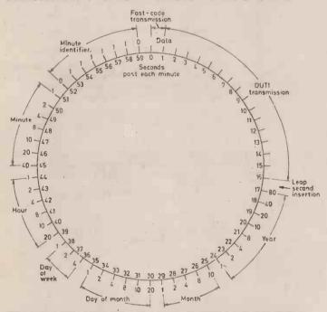
The Rugby MSF clock, this diagram represents one minute in the clock's cycle. The fast code lasts from the zero mark to the first second. The two fast codes are from the second second (oh dear, oh dear) to the 16th second and the 17th to the 59th.
