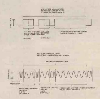
described as "proportional" that is to say a small control stick movement results in a small servo movement — a large control stick movement a large servo movement etc., the servo moving directly in sympathy with the control stick.
