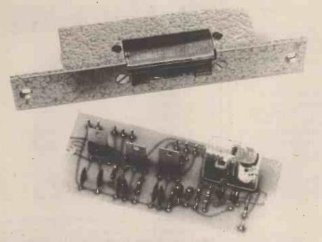
The printed circuit board and solenoid striker plate we used. Naturally any type of solenoid lock can be protected using this system.
