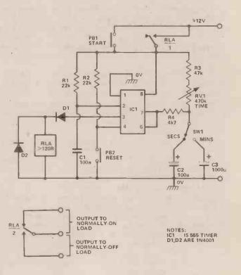
Fig. 2. A 2 range 6-60 second and 1-10 minute timer circuit.
