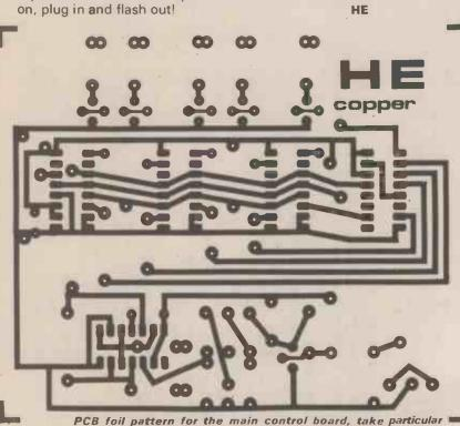
PCB foil pattern for the main control board, take particular care when soldering in the ICs to avoid any solder bridges.
