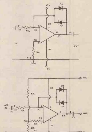
Fig. 3.13 The diode compressor circuit (a) dual voltage supply version, (b) single voltage supply version.
