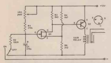
Fig. 6, A timer using a FET, the delay can be varied from about 10 seconds to 1 minute.
