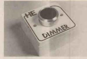
The HE Dimmer in its wall mounting box. For safety we recommend using a plastic, flush mounting box.
