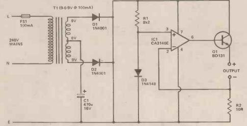
however, as a higher voltage here reverses the comparative input levels to IC1, resulting in the output going lower in voltage, and reducing the voltage across R2 back 0.65 V. The maximum output current (and the charge current obtained) is therefore the current produced with 0.65 V. across 10 ohms, or 65 mA. in other words. Some AA NiCad cells have a
