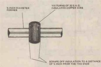
Fig. 4. Details of coil L1, try to keep the coil as neat as possible to avoid any short circuits.
