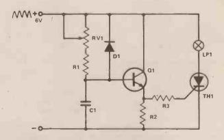
Fig. 13. Using a transistor for triggering a low-voltage circuit.
