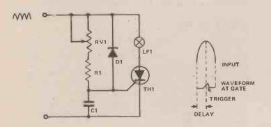
Fig. 11. Simple CR low voltage phase control. Because of the time that C1 takes to charge, the voltage at the gate reaches trigger level some time after the input voltage starts to rise. The delay can be adjusted by altering the setting of RV1. D1 discharge C1 when the input voltage drops to zero again.
