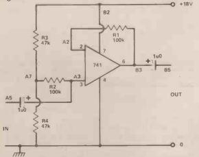
Fig. 3.4 The single-supply version of the circuit of Fig. 3.2. Eurobreadboard line A7 is used for the additional resistors R3, R4 junction with R2.
