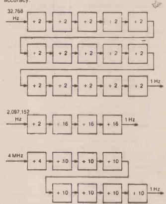
Divider chain found most modern digital watches, the three frequencies are the most common ones in use today. The actual frequency is governed by a quartz crystal oscillator, this is fed to the chain inside the IC. (See page 54.)
