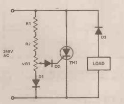
Fig. 15. Mains-voltage power control. All parts of the circuit can be at a dangerous voltage.
