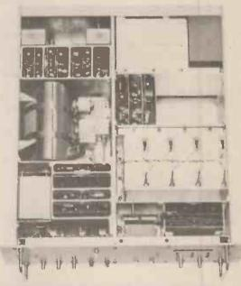
Inside an Atomic Clock, the cylinder in the middle, on the left-hand side is the actual gas cell, the control circuitry and quartz oscillators can be seen at the top, again on the left.
