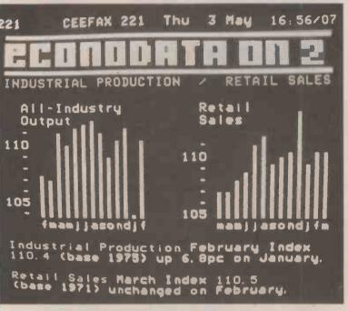
CEEFAX, the clock can be seen on the 'header' on the left-hand side. CEEFAX and ORACLE are both linked to the MSF clock at Rugby so should be accurate to within one-fiftieth of a second.
