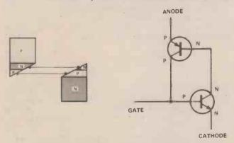
Fig. 2. Two-transistor equivalent (a) as layers, (b) as separate transistors.
