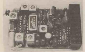
Futaba 6 channel FM receiver/decoder. Employs 'transistor radio' type ICs and filter. Decoder chip is the one nearest the output block connector on the right of the photograph. Note the plug-in crystal bottom left of the PC board.
