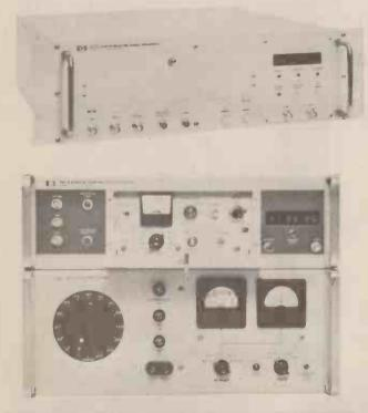
Atomic clocks. The upper one is a laboratory standard Cesium Beam Frequency Reference, a time output is displayed on the right. The lower one is a portable version of the Cesium Beam clock intended for experimental use, the freedom from mains electricity enables the clock to operate safely even during power cuts.
