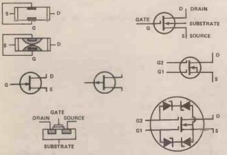
Fig. 1. Construction and symbols used for field effect transistors.
