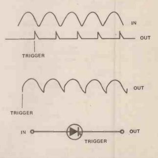
Fig. 10. Phase control of a wave. The average voltage at the output depends on how late in the cycle the thyristor is triggered.
