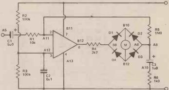
Fig. 3.21 The AC milliammeter circuit.
