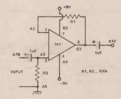
Fig. 3.2 The voltage follower circuit using dual power supplies. The dotted lines indicate where capacitors can be used connected to isolate the 741 from bias voltages in any circuits it's connected to. The letter / number references are to the line positions of the Eurobreadboard.
