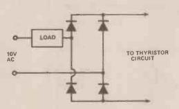
Fig. 14. Using an AC load and a bridge rectifier circuit. The thyristor circuits of Figs. 11 or 13 can be used if the voltage is low.
