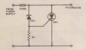
Fig. 4. A crowbar protection circuit.
