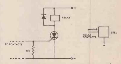
Fig. 5. Burglar alarm basic circuit — the bell cannot be connected directly to the thyristor because each stroke of a bell interrupts the current; this would shut off the thyristor.
