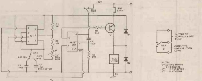
Fig. 3. A 2-range 1-10 minute and 10-100 minute timer circuit.
