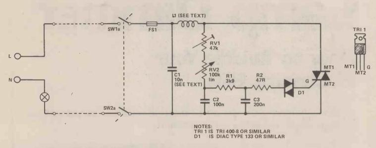
Fig. 1. Circuit diagram of the HE Dimmer, for details of the coil L1 refer to the text and drawing.
