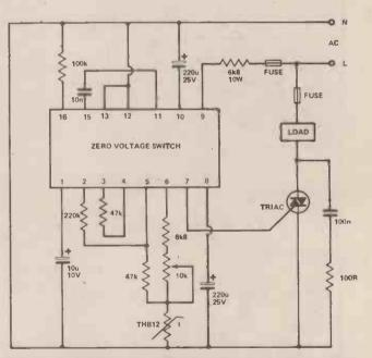
Fig. 19. A zero-crossing switch circuit used for temperature control. Note that all points can be live. (Courtesy of RS Components Ltd).
