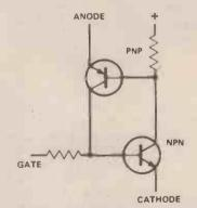
Fig. 3. The equivalent circuit, with gate resistance added.
