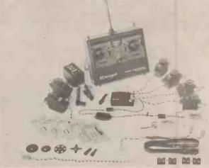
Typical good quality 6 function system with a comprehensive array of accessories including mains voltage charger for receiver and transmitter batteries, alternative capacity receiver batteries and alternative frequency crystal pairs.
