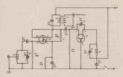
Fig. 3. Circuit for a 144 MHz converter for short wave receivers.
