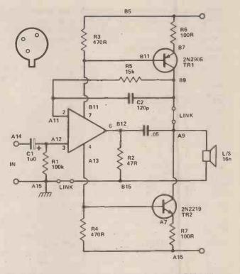
Fig. 3.18 A medium-power output stage using a 741 with two transistors.
