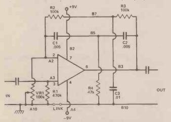
Fig. 3.14 The 'Buzby-cheeper', dual voltage supply version. Input and output capacitors are shown dotted; they will not be needed if the input is a microphone and the output is to an amplifier or tape recorder. RV1 controls the amount of 'cheep' in the sound.
