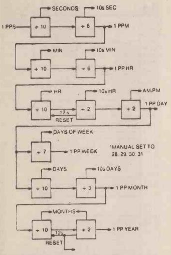
Divider chain for turning a 1 Hz pulse into hours, minutes, seconds, days, months, etc, etc.
