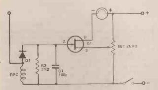
Fig. 4. Field strength meter, useful for determining the efficiency of RF equipment.
