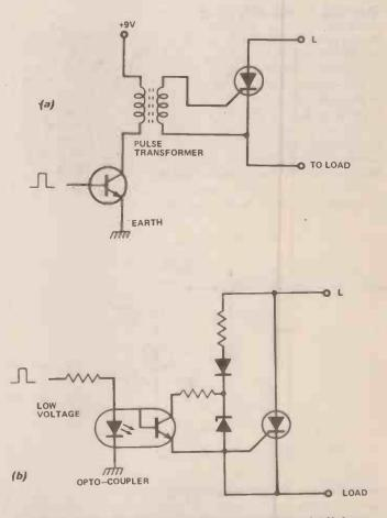
Fig. 16. Isolating the firing circuit from the thyristor. (a) Using a pulse transformer. (b) Using an optoisolator. With either device, the insulation between the circuits can be good enough to withstand several thousand volts.
