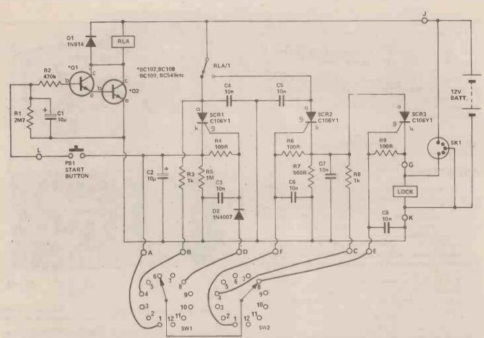
Fig. 1 The circuit diagram, SW1, SW2 and PB1 have to be operated in the correct sequence before the lock will open. Any deviation in sequence will result in the lock remaining secure
