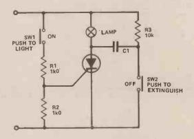
Fig. 7. Using a capacitor to switch off a thyroistor.
