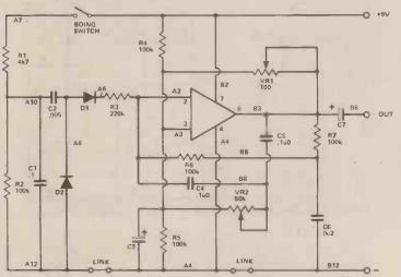
Fig. 3.20 The 'Boing' circuit.
