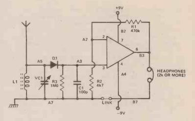
Fig. 3.9 A simple radio circuit, using the high gain of the 741 to amplify the feeble signals from the diode detector. D1 must be a germanium diode such as OA91. Note the link (wire) between A7 and B7 to ensure enough plug-in points on the earth line.
