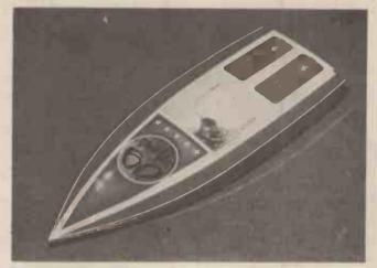
A typical G.R.P. hulled R / C speedboat — this example powered by a 10cc engine. Radio control is limited to throttle and steering. Note the water cooling pipes in the engine compartment.
