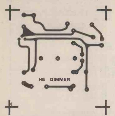
Fig. 3. PCB foil pattern for the Dimmer, take extra care if you make your own PCB to avoid any stray whiskers of copper creating short circuits, mains is dangerous stuff to play around with.
