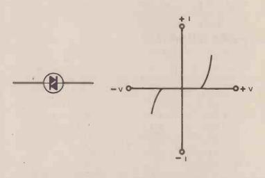
Fig. 12. Trigger diode. (A) symboll (b) characteristic
