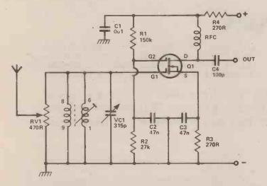
Fig. 2. Circuit diagram for a Medium Frequency RF amplifier.
