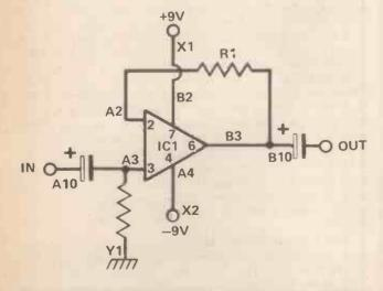
Fig. 3. Instant circuit! When the Eurobreadboard numbers are put on to the circuit, the few extra components that are needed go between these lines and earth or supply lines, or can be accommodated on spare lines.
