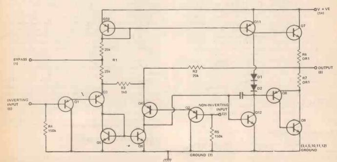
Fig. 1. The internal circuitry of the LM380 IC.
