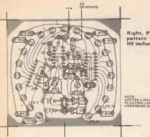
**Right**, PCB foil pattern for the HE tachometer.
