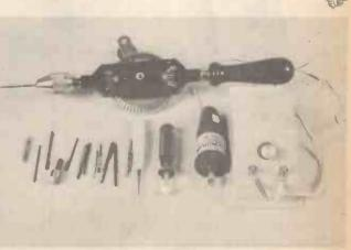
Tools for cutting holes, countersinking etc. The purposedesigned PCB drill is well worth thinking about.
