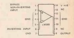
Fig. 2. Outline and pin connections of the standard 14 pin Dual-in-line (DIL) version of the LM380.
