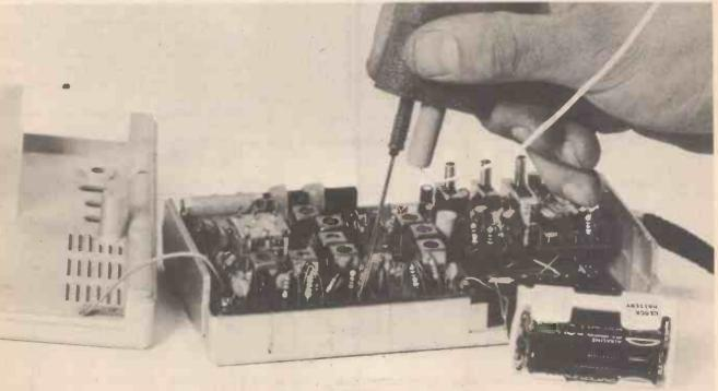
start fault-finding by injecting a signal at the slider of the volume control. If the resulting 1 kHz signal is heard in the set's speaker you'll know that the audio amplifier is OK, and the fault therefore lays further back, in the IF or RF sections of the receiver. If the signal is not heard, you'll know that the audio amplifier is defective. By systematically working either forwards or backwards through the circuit, injecting or tracing as appropriate, the fault area can be easily located.
