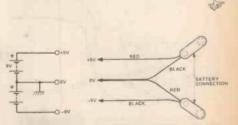
Fig 8. Using two batteries for a power supply.
