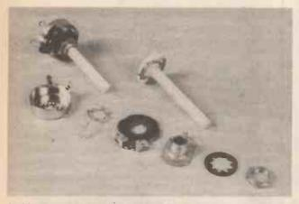
Inside the potentiometer, note the metal wiper pressed on to the shaft, the resistive element (centre) is moulded on to a phenolic former.
