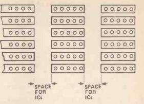
Fig. 7. The track pattern of DIL-board. Using this type of board saves on cutting.
