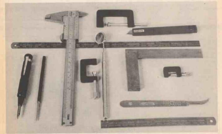
Essential metal working tools, the automatic centre-punch (far left) will ensure that drills don't go wandering all over your neat front 'panels. The mirror on a stick is handy for seeing into the inaccessible corners. You'll need a sharp scalpel or knife for trimming, slicing etc, it'll also come in handy for cutting the Band-aid when you miss. Remember, it doesn't hurt so much with a sharp knife.
