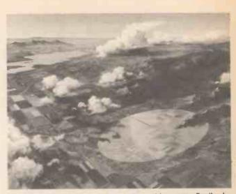
The 'Rectenna as seen from the air, it would measure 5 miles by 7 1/2 miles. Microwave levels beneath the structure would allow grazing and farming.
