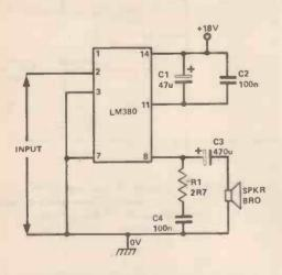
Fig. 3. A simple Non-Inverting 2 watt audio amplifier.
