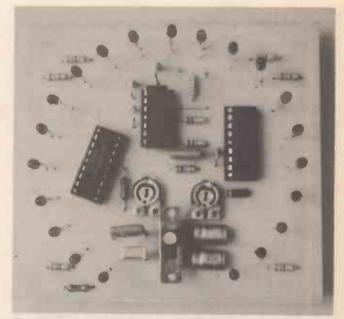
The HE tachometer, make sure all polarised components are inserted the correct way round.
