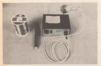
A temperature controlled soldering iron, nice to have if you plan to leave it on for prolonged periods.
