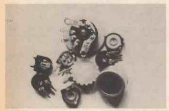
A collection of pre-sets, the upper one is in fact a thumb-wheel pot, with switch, often found in cheap transistor radios, not dissimilar to the genuine pre-set immediately below.
