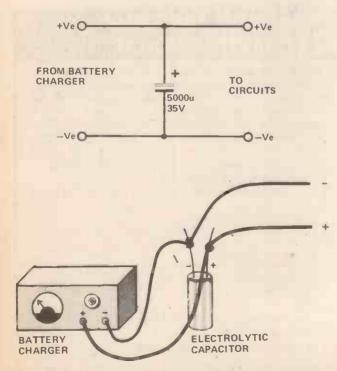
Fig. 9. Adding smoothing to a battery charger — a cheap way to get a single voltage supply suitable for many circuits.
