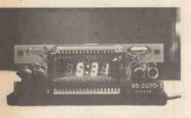
The completed clock before insertion into the case the two metal strips at the top right and left of the PCB are for time setting.
