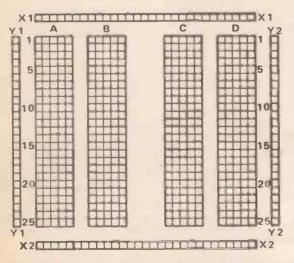
Fig. 1. The Eurobreadboard layout. Columns AB or CD are used for small ICs, the larger spacings between B and C can be used for the bigger ICs with 15 mm between lines. (B and C) so that any of the normal IC's right up to the monster microprocessor can be fitted in. The size of the board is enough to permit assembling any of the circuits we shall use, but the price is as low as several much smaller and less suitable competitors.
