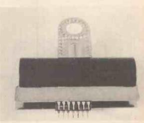
Fig. 4. Using an office paper clamp as a heat-sink. These clamps come in various sizes which are suitable for all the common linear ICs.
