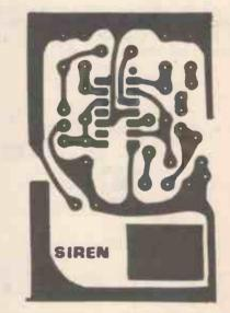
Fig. 6. PCB foil pattern for the optional electronic siren.
