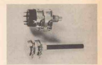
Ganged pots, the two separate pots are joined together by a single shaft, most often seen in stereo systems.
