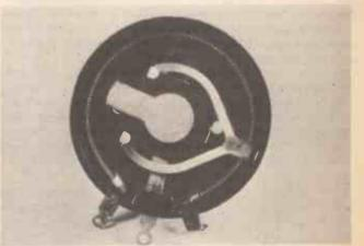
Inside a wire-round potentiometer, the windings are clearly visible inside the outer casing, a small tab of carbon is usually bonded to the underside of the wiper.
