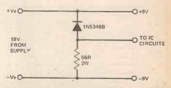
Fig. 10. Obtaining dual supplies from a single 18 V supply. The 1N5346B is a 9.1 V zener diode rated at 5 W and obtainable from RS Components stockists.
