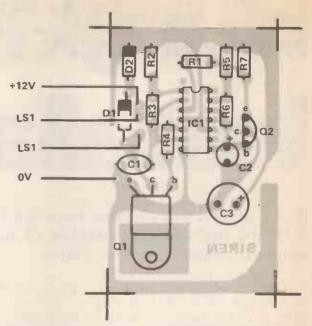
Fig. 5. Overlay diagram for the optional electronic siren.
