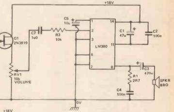
Fig 9. Above: A general purpose 2-watt audio amplifier with an input impedance of 10 Meg ohms.
