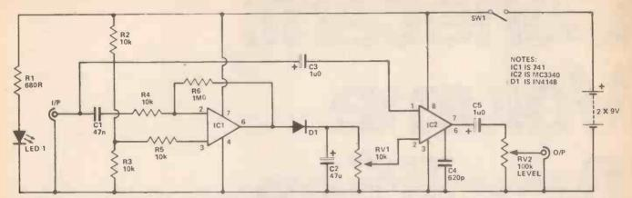
Figure 2. Circuit diagram of the HE Constant Volume Amplifier.
