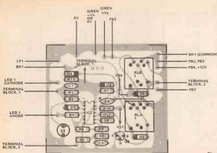
Fig. 2. PCB overlay for the Home Security System, note the position of all polarised components.
