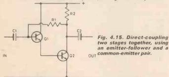
with its input signal, bias and negative feedback can be applied by the resistance R1. If we want this to act for bias only, the total resistance can be divided into two sections with a capacitor to remove (or 'decouple') signals.
