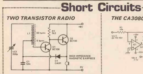
Although transistors are cheap, this was certainly not true some years ago and transistors werei made to work at maximum efficiency. A common technique in simple radio circuits was to use a reflex circuit, that is one transistor amplified both at RF and AF
