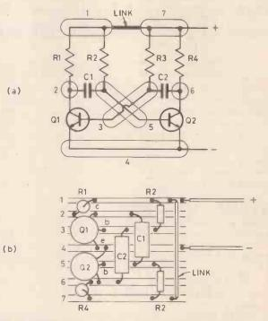
Fig. 3. Mirror-image layouts (A) Marked-out circuit (B) Board layout.
