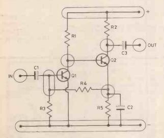
Fig. 1. Marking out circuit junctions.
