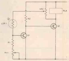
Fig. 4.21. A more controllable circuit with variable hysteresis.
