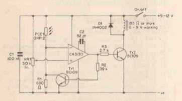
Fig. 5. A modification to Fig. 3. which holds the relay on, once it has switched, irrespective of the level of light falling on PCC1.
