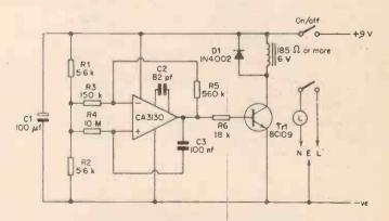
Fig. 9. C3 and R4 make the IC oscillate slowly and in turn the relay switches on and off in sympathy.
