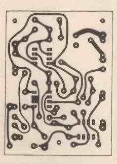
The PCB pattern for the car alarm, shown here full size.
