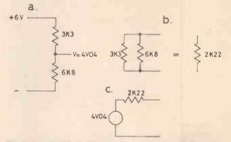
Fig. 5. A potential divider circuit (a) is equivalent to a voltage (the open circuit voltage) in series with resistance, found by combining the resistors in parallel (b). The result is shown (c).
