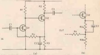
Fig. 17: A high gain two transistor circuit (a) with direct coupling negative feedback of signal can be achieved by removing C2, or by using the circuit in (b) where only part of R3 is bypassed.
