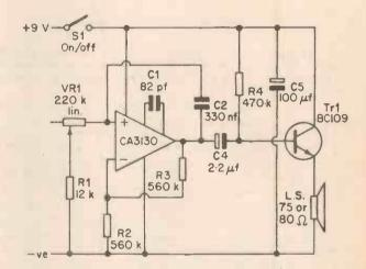
Fig. 1. Here the IC is converted as a low frequency oscillator operating over the range of 50-200 pulses per minute, this is determined by C2 and VR1. The transistor acts as a simple amplifier to drive the loudspeaker.
