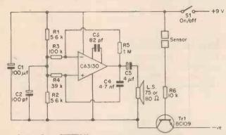
Fig. 2. Rain alarm circuit. Basically an audio oscillator with the negative supply controlled by Tr1. When a drop of rain bridges the sensor, Tr1 acts as a low value resistor allowing current to reach the rest of the circuit.
