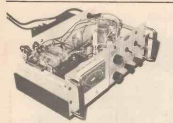
With the lid off the exposed transformer tags can be seen at the left of the box.
