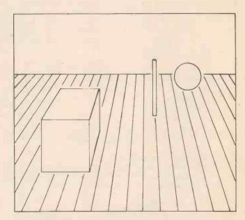
Two dimensional pictures such as this do not change with different viewing angles. With a hologram the sphere would move behind the pole, and the cube could obscure the pole if the viewing angle was changed, by moving your head.
