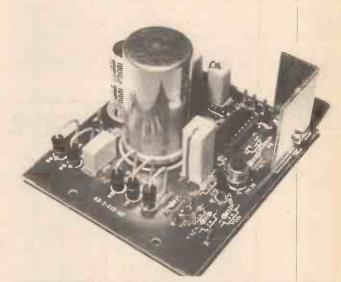
Above: the PCB with all the components in place, but without wiring: some of the pins can be seen.
