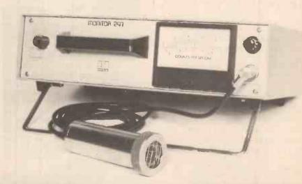
Simple radioactivity measuring equipment. The end-window Geiger tube is shown at the front. The meter indicates the counting rate. (Courtesy: ESI Nuclear Ltd.)
