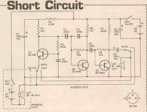
in the connecting cable, and it also gives a good match to the microphones. The following two stages are both straightforward common emitter amplifiers. C4 rolls off the high frequency response of the circuit and this aids stability. It can also help to prevent RF breakthrough.
