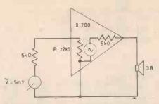
Fig. 4.4. Single-transistor amplifier, input from a pick-up cartridge, output to a loudspeaker.
