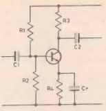
Fig. 4.9. Using a decoupling capacitor (Ce) so that there is no series feedback caused by the emitter resistor R4.
