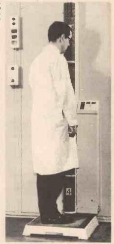
Monitor for checking the contamination of personnel working with radioactive materials. It comprises a vertical array of 11 beta / gamma Geiger detectors with an additional detector for monitoring the soles of shoes. An alarm bell is included in this equipment, whilst the tone chimes sound when there is no contamination. (Courtesy: Nuclear Enterprises Ltd.)
