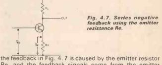
the feedback in Fig. 4.7 is caused by the emitter resistor Re, and the feedback signals come from the emitter current and affects the base-emitter voltage. The action is something like this.
