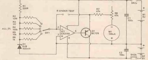
input, and in this case is the resistor under test.
