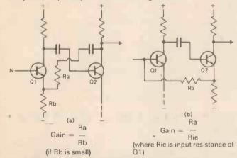
Fig. 4.14. Methods of connecting negative feedback over two stages. (a) Collector-to-emitter, (b) emitter-to-base.
