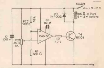
Fig. 4 Connecting Fig. 3. differently, the same components can be used to switch when the light level increases.
