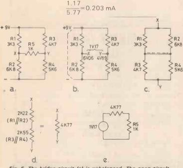
Fig. 6. The bridge circuit (a) is unbalanced. The open circuit voltage across R5 is easily found (b); finding the resistance (c) needs a little bit of re-drawing (d). The final equivalent is shown in :e).
