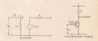
Fig. 4.2. Equivalent circuit of a transistor with a load resistor.
