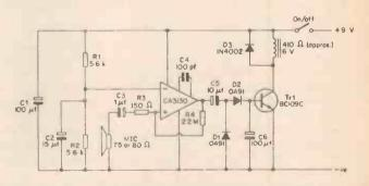
Fig. 7. A sound operated switch circuit which has applications as a baby alarm.
