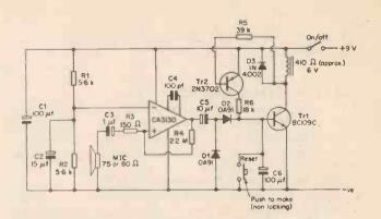
Fig. 8. A self-latching version of Fig. 7. In this arrangement Tr1 and Tr2 act in much the same way as a thyristor (SCR).
