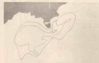
Radioactive clay was mixed with the sea bed off Dodman Point, Cornwall. The contours show how the radioiostope has spread 10-12 days after it was added. Such charts can be used to estimate the movement of the sea bed. (Courtesy: U.K.A.E.A.).
