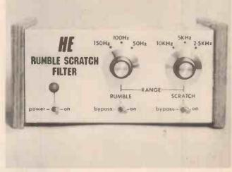
The finished filter. Note the two range switches, for the rumble and scratch sections, and the frequencies which they select.
