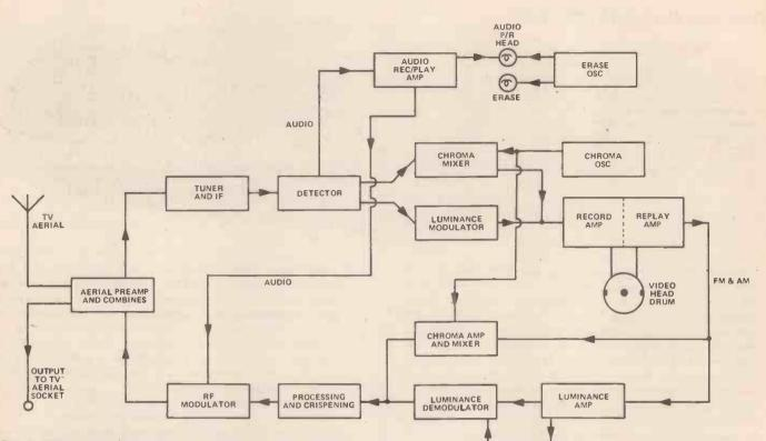
Fig. 2. Video Tape Recorders are easily the most complex pieces of machinery ever to find their way into the home as they contain most of a colour TV circuit plus sophisticated mechanics. This block diagram gives the essential circuit elements; see the text for a more detailed explanation.
