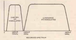
Fig. 3. To get the most out of a tape recorder, the original TV spectrum is considerably rearranged when put on the tape. The whole luminance section (the monochrome picture) is shifted up the spectrum and is frequency modulated. The colour information is slotted onto lower frequencies and amplitude modulated.
