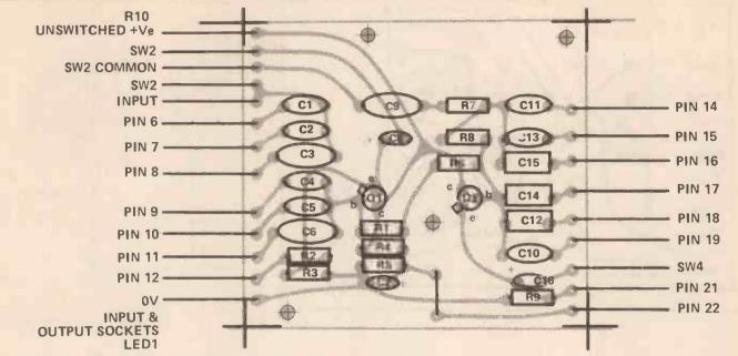
How to position the components on the PCB.
