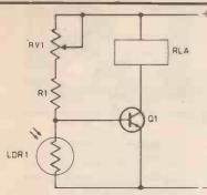
Fig. 4.18. Circuit for operating a relay when the light level drops.
