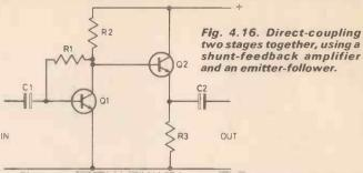
emitter resistor ensures that the biasing of the emitter follower is correct, and the biasing of the first stage is set by the shunt feedback resistor R1.
