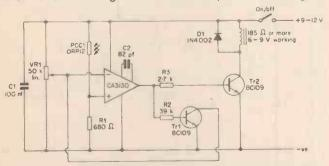
Fig. 6. A latching version of Fig. 4. makes a circuit which operates nicely as a burglar alarm.
