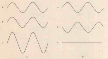
Fig. 4.5. Adding wave voltages. (a) in phase, (b) in antiphase. The sum or resultant wave can be large or small depending on the phase of the waves being added.
