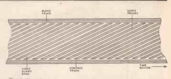
Fig. 1. The high tape head to tape speed is achieved by rotating the heads to give diagonal strips of recorded material. The audio is recorded on a narrow track on one edge.
