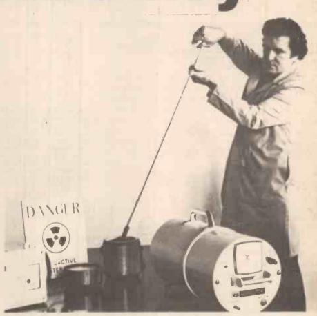
The operator uses long tongs to keep his body away from the radioactive material in the container, whilst the monitor continuously checks the radiation level. (Courtesy Nuclear Enterprises Ltd.)
