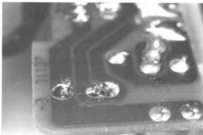
*With both component joints now desoldered, the component immediately fell out and the new device could then be inserted and re-soldered.*
