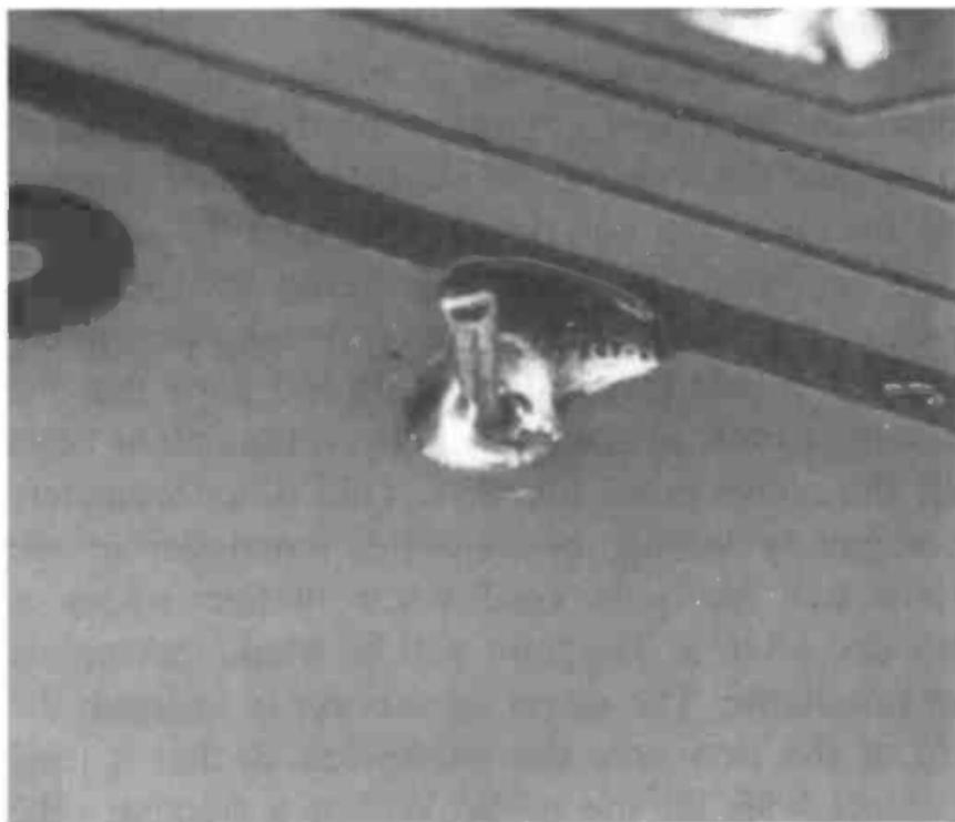
*An example of a “dry joint” – the solder failed to flow into the component lead because of impurities and grease present on the lead. It would need to be desoldered, removed and cleaned.*
