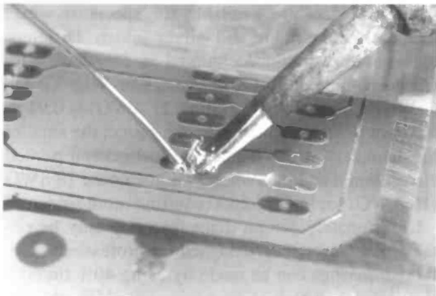
*Then melt a few millimetres of solder to flood the joint with molten solder. Remove the iron and allow the joint to cool naturally.*
