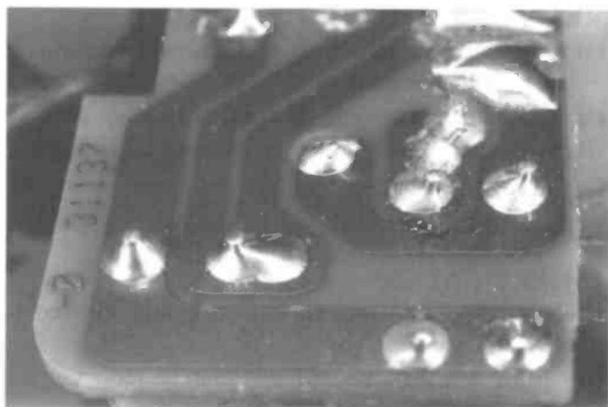
*An example of commercial mass-produced solder joints, note how smooth and shiny they are.*
