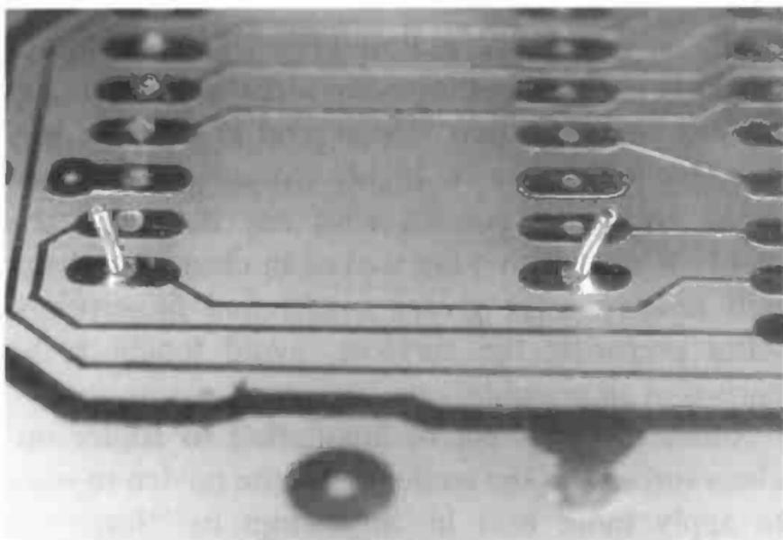
*Snip any component leads to length ready for soldering.*
