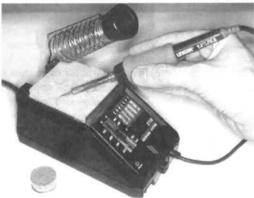
*Wipe the tip of a hot soldering iron on a damp sponge to remove debris from the bit, which should be shiny before applying to the components.*
