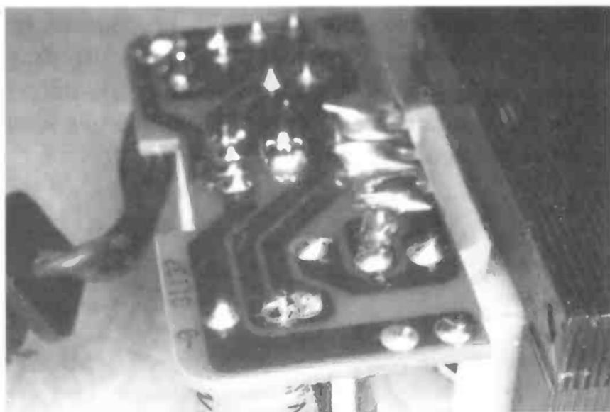
*The component solder pad with the solder removed.*
