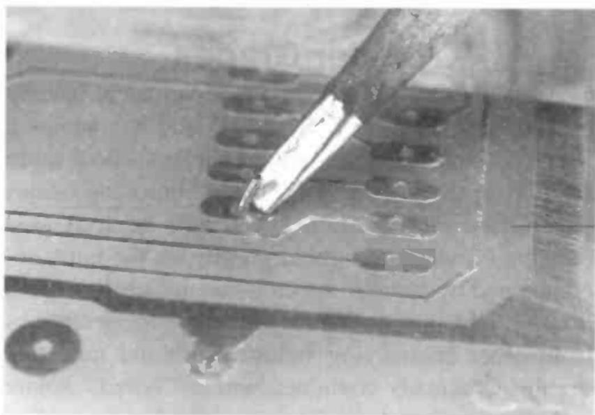
*Apply the hot iron tip in order to heat both the lead and the copper solder pad at the same time.*
