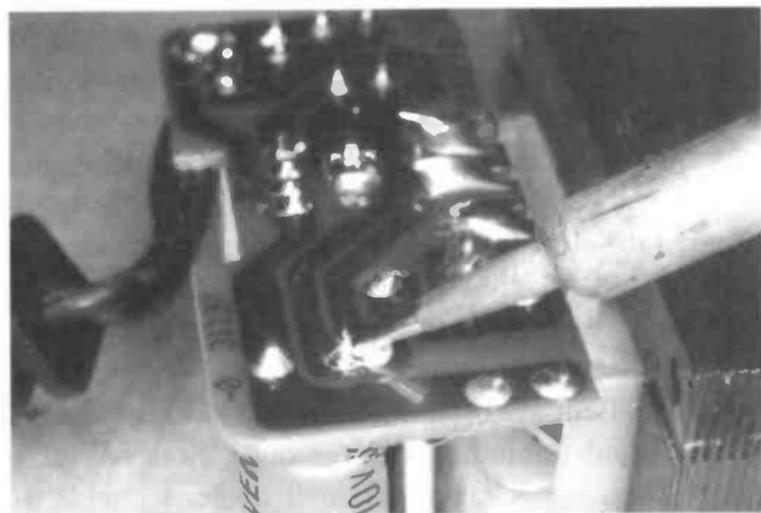
*Apply a hot soldering iron to the joint to be desoldered.*
