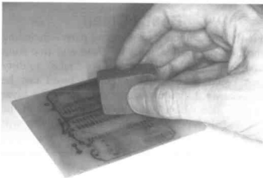
*Copper clad boards should be cleaned using an abrasive rubber block, for example, in order to remove tarnishing and contamination. Wipe over with a solvent cleaner afterwards and avoid touching the copper.*
