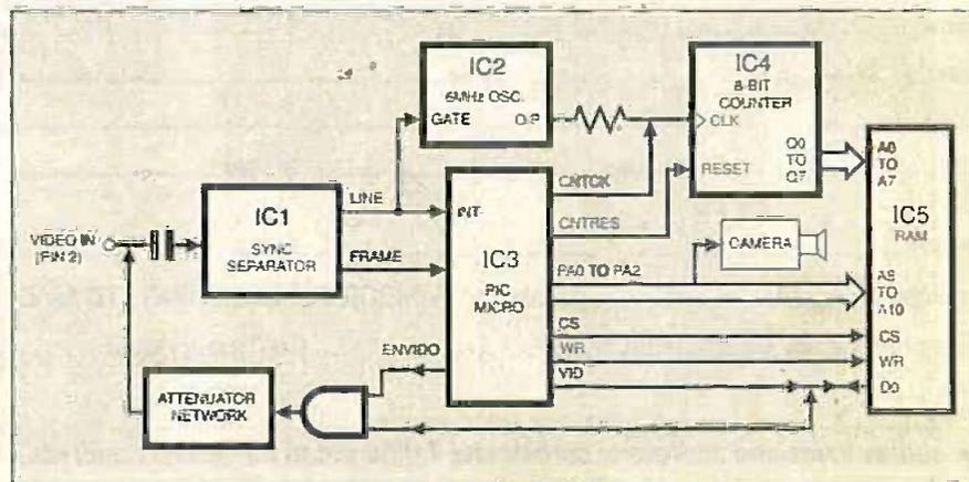
Fig.1. System block diagram for the Time and Date Generator.
