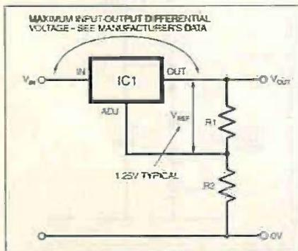
Fig.3. Calculating the output voltage from a variable voltage regulator. A typical value for  $V_{ref}$  is 1.25V.
