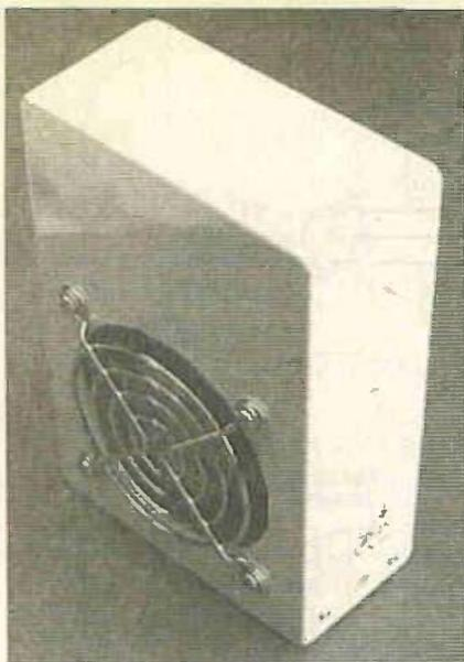
The filter consists of open-pored foam, which is partly charcoal filled. This type of structure offers very little resistance to the passage of air. Charcoal is an excellent absorber of gaseous contaminants but in this application the flow of air is very fast and absorption may not always be complete.
