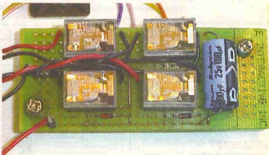
Fully assembled relay board.
