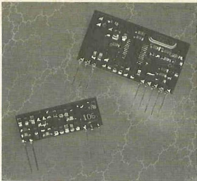
DIP International has introduced new UHF transmitter and receiver radio devices specifically designed for low power radio applications. The MK KES modules are designed for use on 418MHz, 433.92MHz and the new proposed pan-European standard of 898.95MHz.
