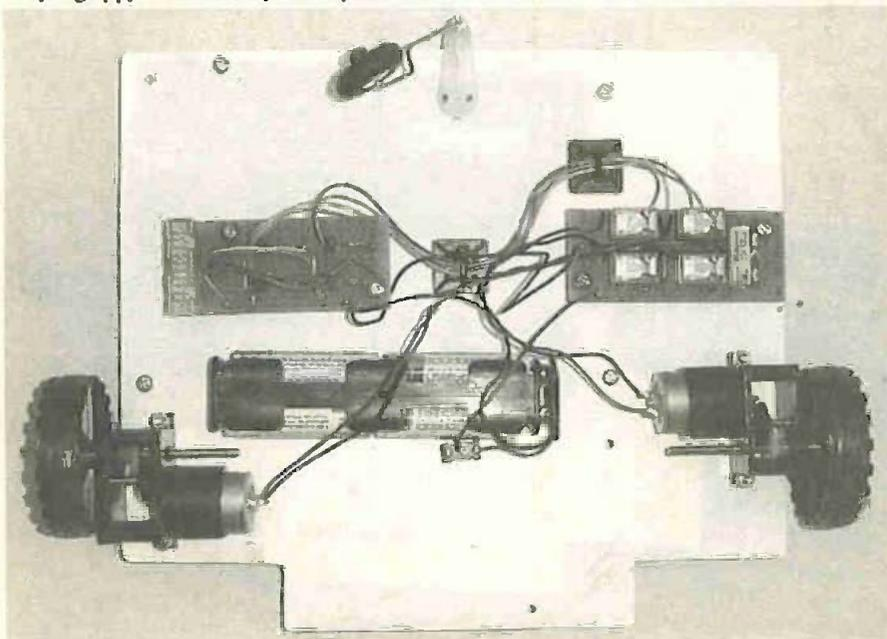
The underside view of the motor platform showing the complete PhizzyBot hardware in position.
