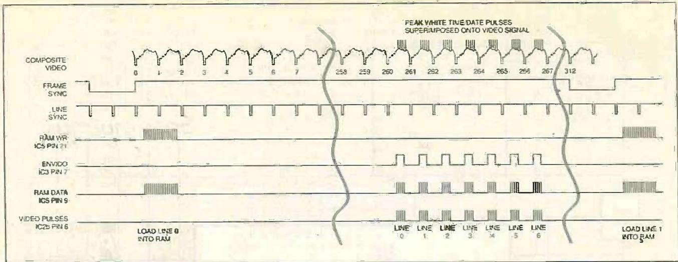
Fig.4. Example waveforms for the Time and Date Generator circuit.
