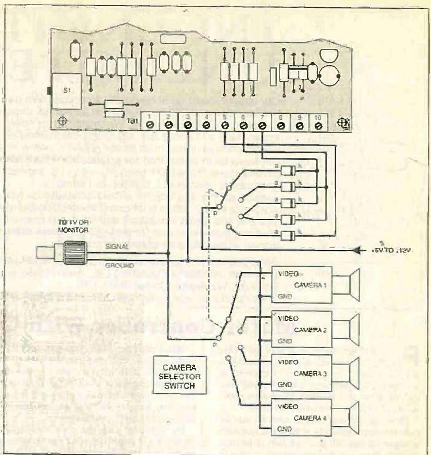
Fig.9. A typical four camera system using a 4-way 2-pole rotary switch for camera selection. The power supply connections are not shown in this diagram - see Fig.8.
