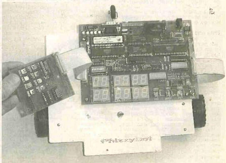
The PhizzyBot platform with the PhizzyB computer board mounted in position, plus the temporary connection of the switched control board.
