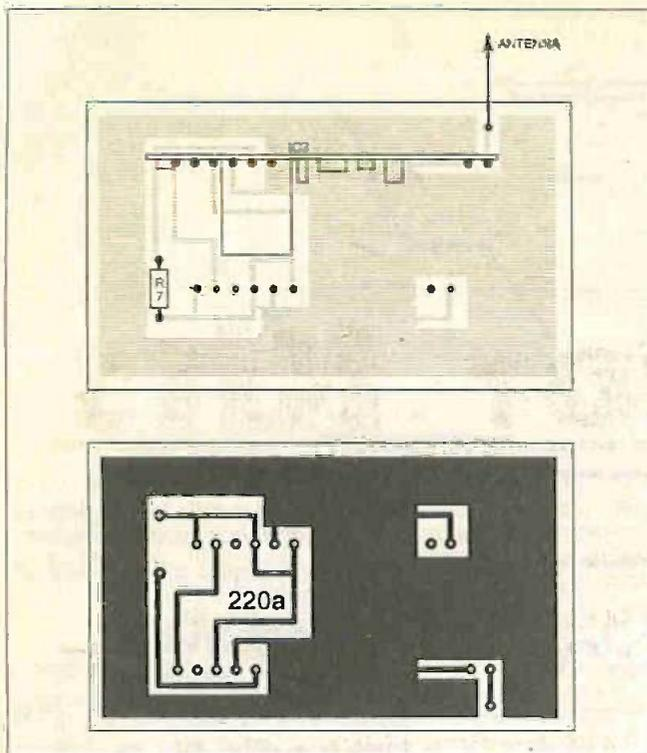
Fig. 18. F.M. Receiver adaptor printed circuit board details.
