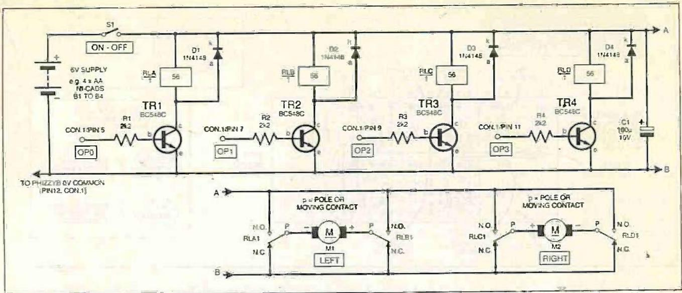
Fig. 1. Complete circuit diagram for the PhizzyBot motor control interface.
