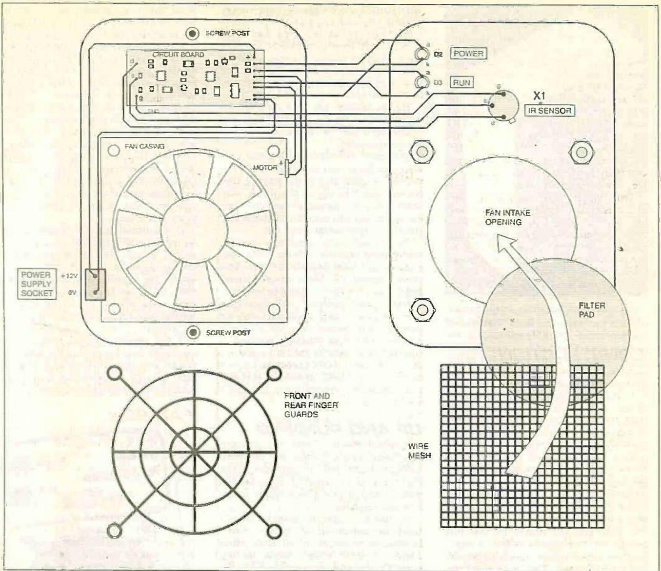
Fig. 4. Internal layout and interconnections of the Smoke Absorber components within its case.
