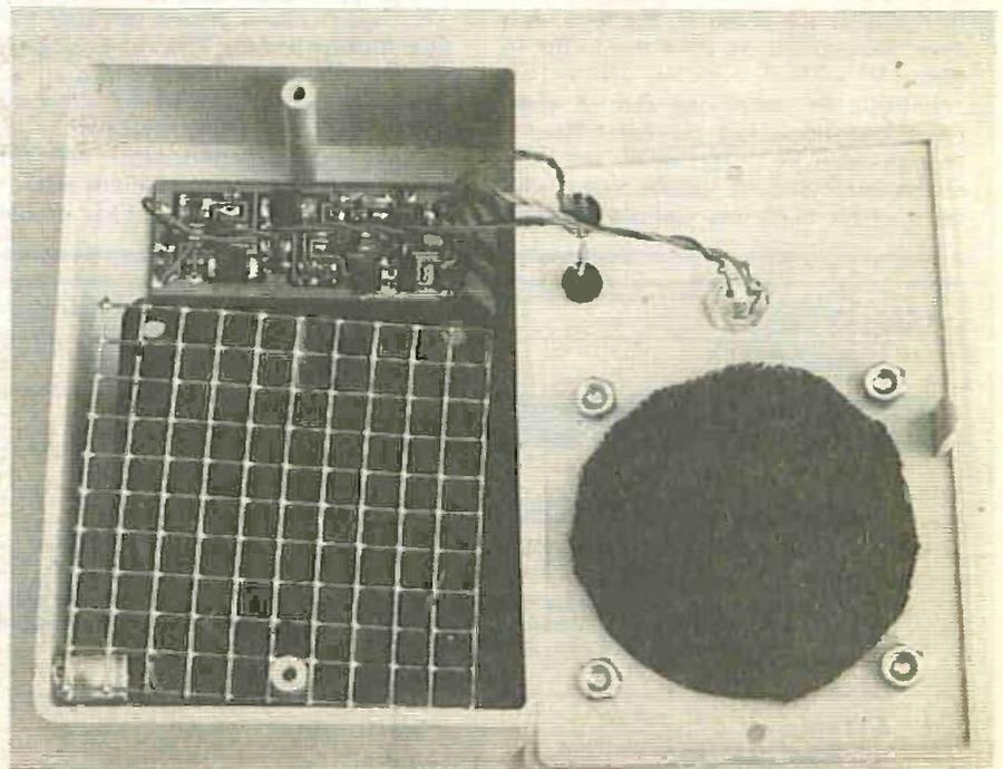
Internal layout of the Smoke Absorber
