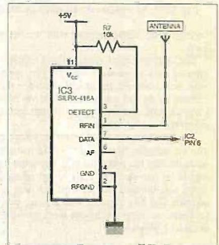
Fig. 17. Receiver modification details for f.m. operation.
