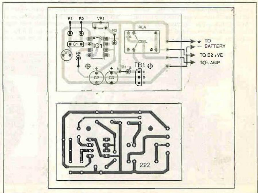
Fig.2. Auto Cupboard Light printed circuit board component layout and full size underside copper foil master pattern.
