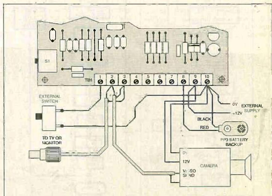
Fig.8. Typical interwiring and power supply arrangement for a single video camera setup. The external switch is optional and replaces S1 on the p.c.b.
