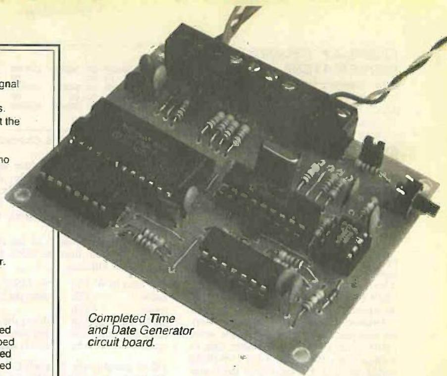
Completed Time and Date Generator circuit board.
