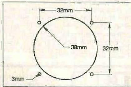
Fig.1. Mounting holes for a panel meter look easy enough, but a 38mm dia. hole can be awkward to produce.
