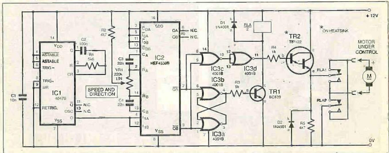
Fig. 1. Circuit diagram for a PWM Motor Controller, with centre off.
