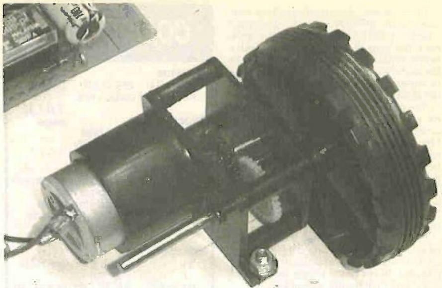
Close-up detail of a motor and its wheel.
