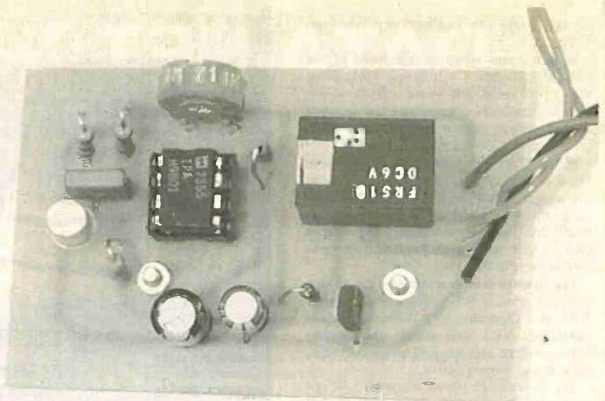
Layout of components on the completed p.c.b. Note that the metal cased tilt switch, to the left of the i.c., should be carefully bent so that the wire end is slightly higher when the unit is mounted on a door.
