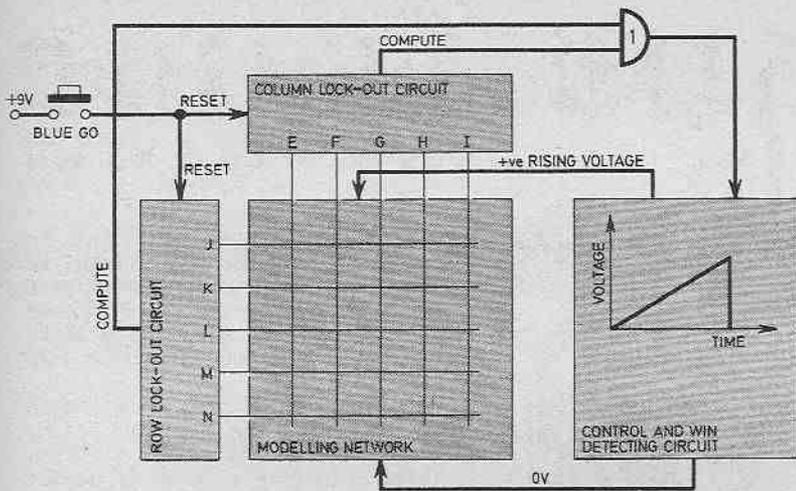
Fig.2. Block diagram showing all sections of the game.
