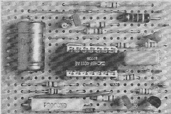
The prototype component board. This differs from that shown below where D2, D3 and R14 have been incorporated on the board.
