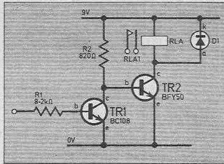
Fig. 8.8. A relay with its higher current requirement and back e.m.f., requires a slightly more complicated circuit. This circuit also produces an inversion of the logic input.
