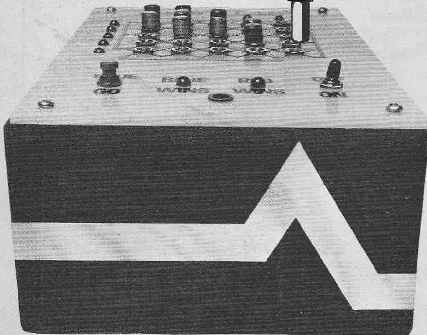
strategy of the machine consists of choosing the resistor across which the maximum voltage occurs. If two or more resistors show the same maximum voltage, one is selected at random.
