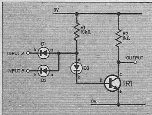
Fig. 8.9. The circuit shown is a logical NAND gate. Only when both inputs are high does the output go low.
