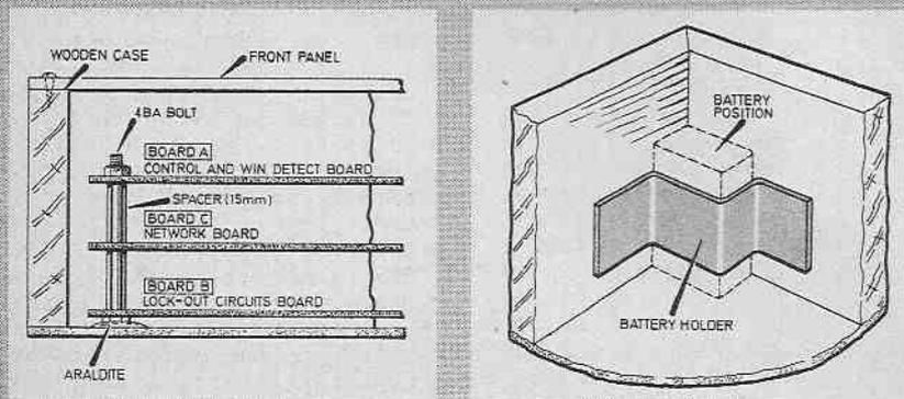
Fig. 10. Interior views of the cabinet. The diagram left, shows the circuit board mounting arrangement and the one on the right shows the battery mounting clip.
