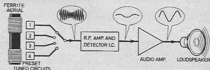
Radio frequency signals from the transmitter induce voltages in the coils on the ferrite rod aerial. Four r.f. tuned circuits are formed with the aerial which can each be inputted to the r.f. amplifier/detector i.c. The output from this is the required audio signal which receives boost from the audio amplifier to be heard in the loudspeaker.
