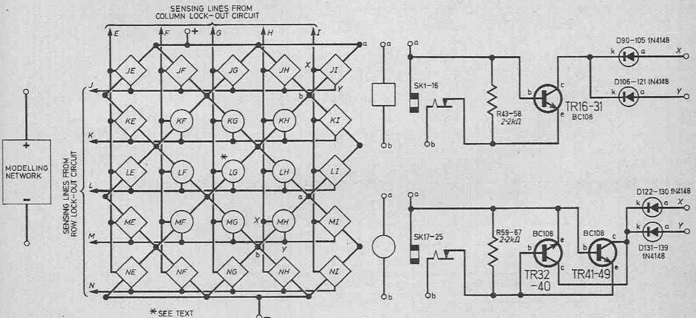
Fig.5. Circuit diagram of the modelling network. Note that this is made up of identical network elements, the circuit diagrams of which are shown on the right. This is built up on board C.
