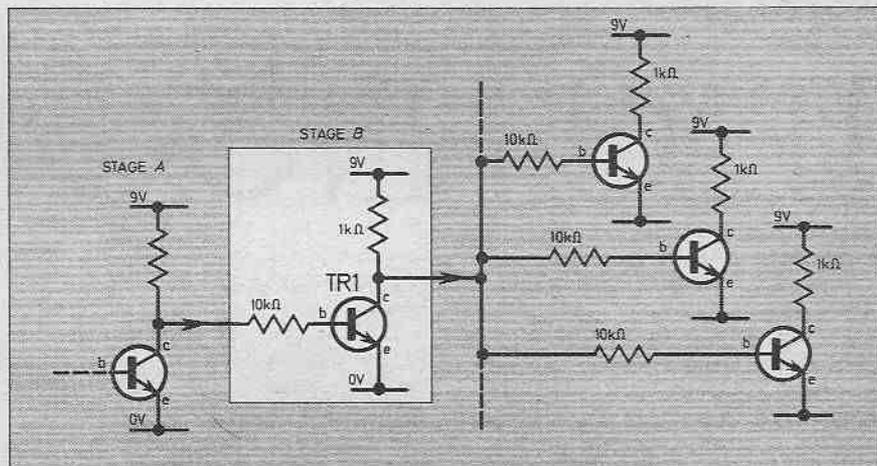
Fig. 8.4. The transistor switch (Fig. 8.3) as it looks when in a system. Note that only one output feeds it whilst it feeds many inputs.
