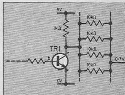
Fig. 8.5. The loading on the switch in Fig. 8.4 can be redrawn thus. The load appears as a number of 10kΩ resistors in parallel all to 0.7V.
