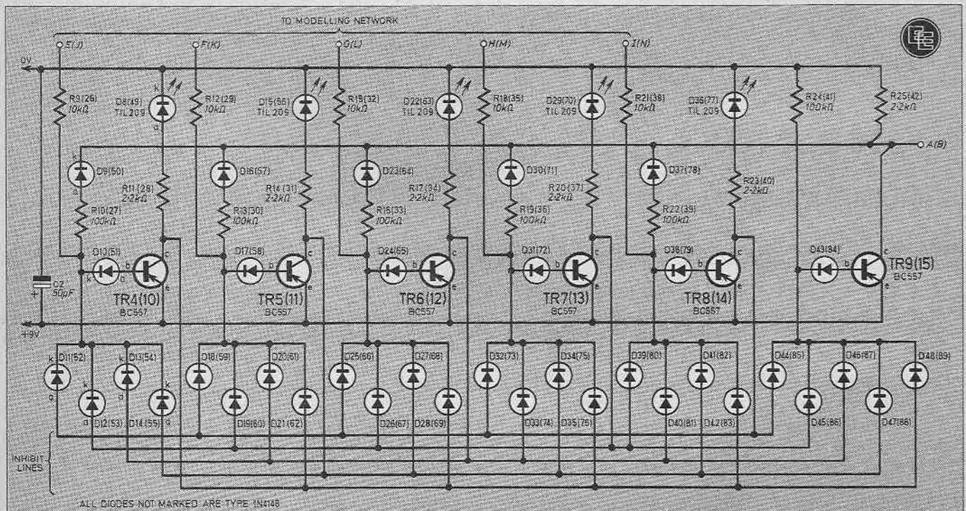
Fig. 4. Complete diagram of the lockout circuits. Note that two of these are required, one for the rows and one for the columns. Bracketted component references are for the column lockout circuit and unbracketed ones for the row lockout circuit. These are both built on board B.
