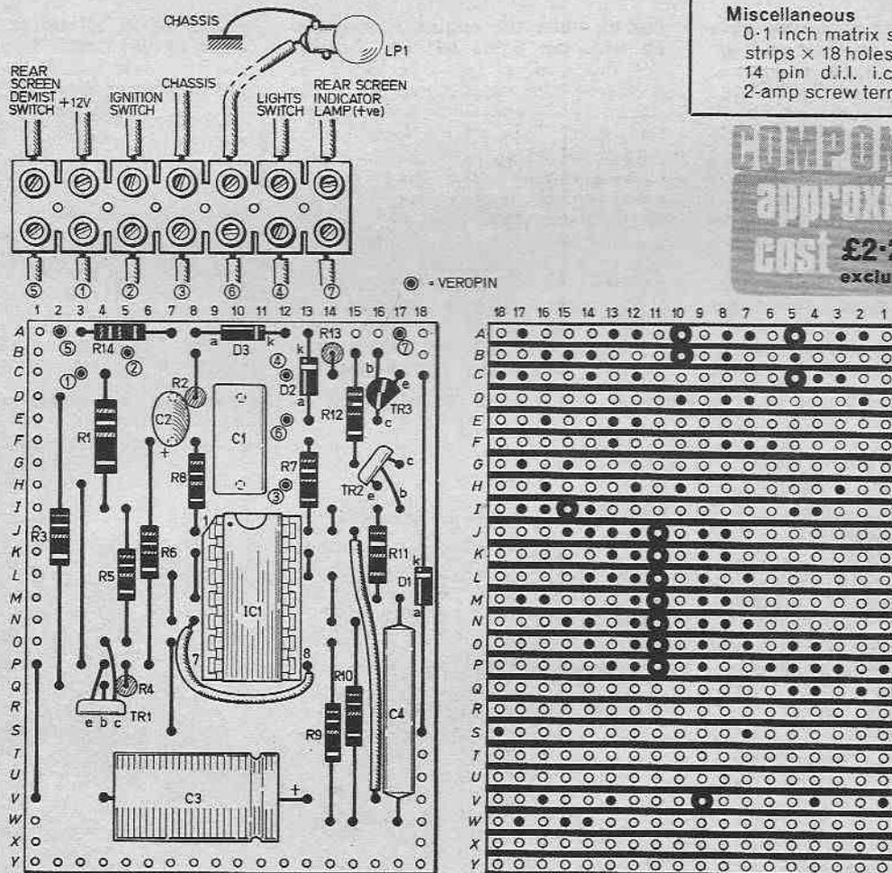
Fig. 2. The layout of the components on the topside of the board and the breaks to be made in the copper strips. Numbered leads from the terminal block refer to Veropins on board. Only one indicator lamp should be used, either LP1 or existing panel lamp for some other function (e.g. rear screen demister indicator).
