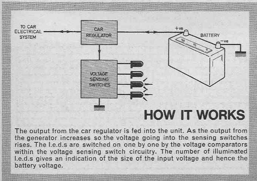
The output from the car regulator is fed into the unit. As the output from the generator increases so the voltage going into the sensing switches rises. The l.e.d.s are switched on one by one by the voltage comparators within the voltage sensing switch circuitry. The number of illuminated l.e.d.s gives an indication of the size of the input voltage and hence the battery voltage.
