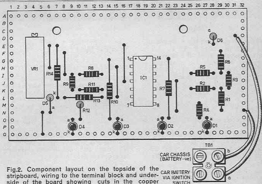
Fig.2. Component layout on the topside of the stripboard, wiring to the terminal block and underside of the board showing cuts in the copper track. The l.e.d.s may be mounted separately from the board, see text.
