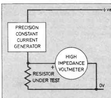
Fig. 1. Method of operation of the Resistance Meter.
