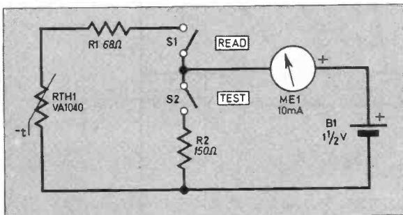
Fig. 2. Circuit diagram of the Remote Reading Thermometer.
