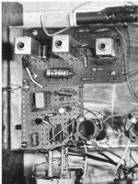
It is probably advisable to insert a few components at a time, turn the board over, and solder the joints, then snip off any excess wire. The MC connections are to the metal chassis.
