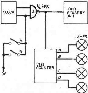
Fig. 8.9. Circuit diagram of the reaction timer.
