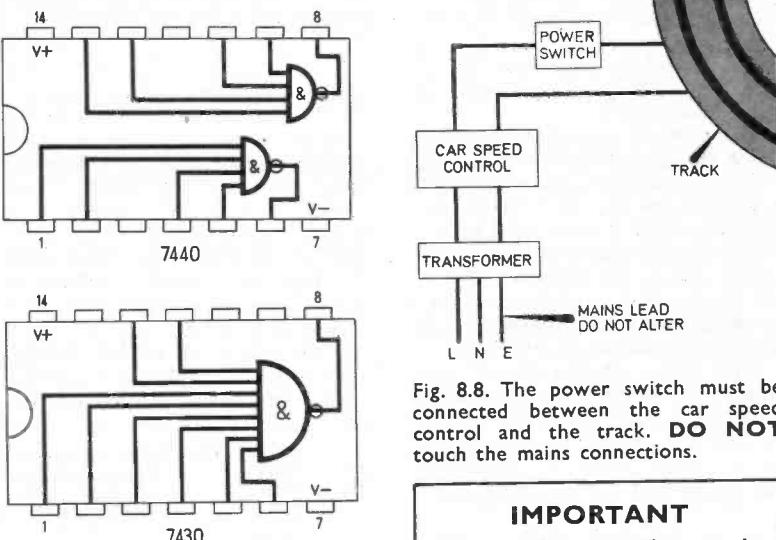
Fig. 8.7. Pin connection details of the 7440 and 7430 integrated circuits.
