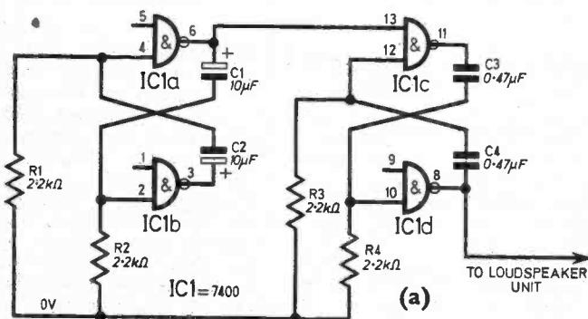
Fig. 8.10. Interrupted tone alarm. The circuit diagram is shown at (a) and the layout on the experimental deck at (b).
