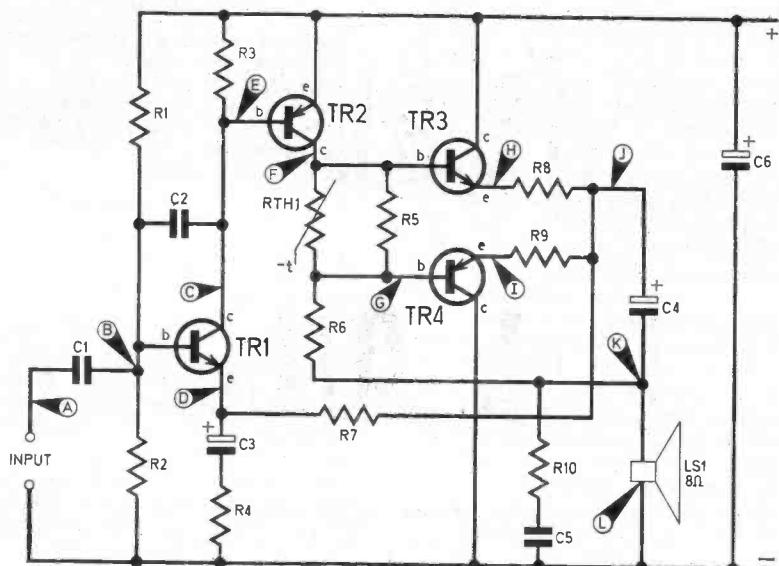
Fig. 1.4. The circuit diagram of a typical audio amplifier with test probe points indicated by A to L.
