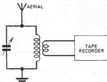
Fig. 2. Tuned circuit arrangement for experimentation.
