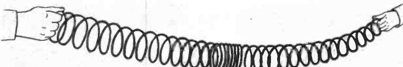
Fig. 1. An "energy packet" travelling along a Slinky spring.
