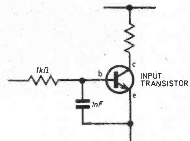
Fig. 3. Low pass filter to reduce unwanted r.f. signals.
