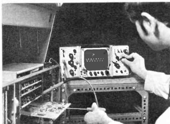
Type 21 marine radar console under test.
