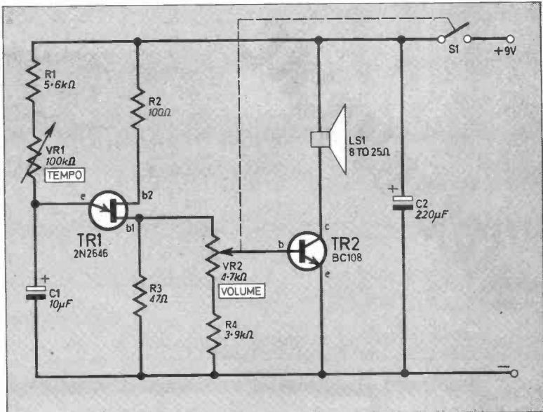
Fig. 2. Complete circuit diagram of the Metronome.
