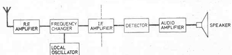
Fig. 1.1. Block diagram of a typical radio receiver.
