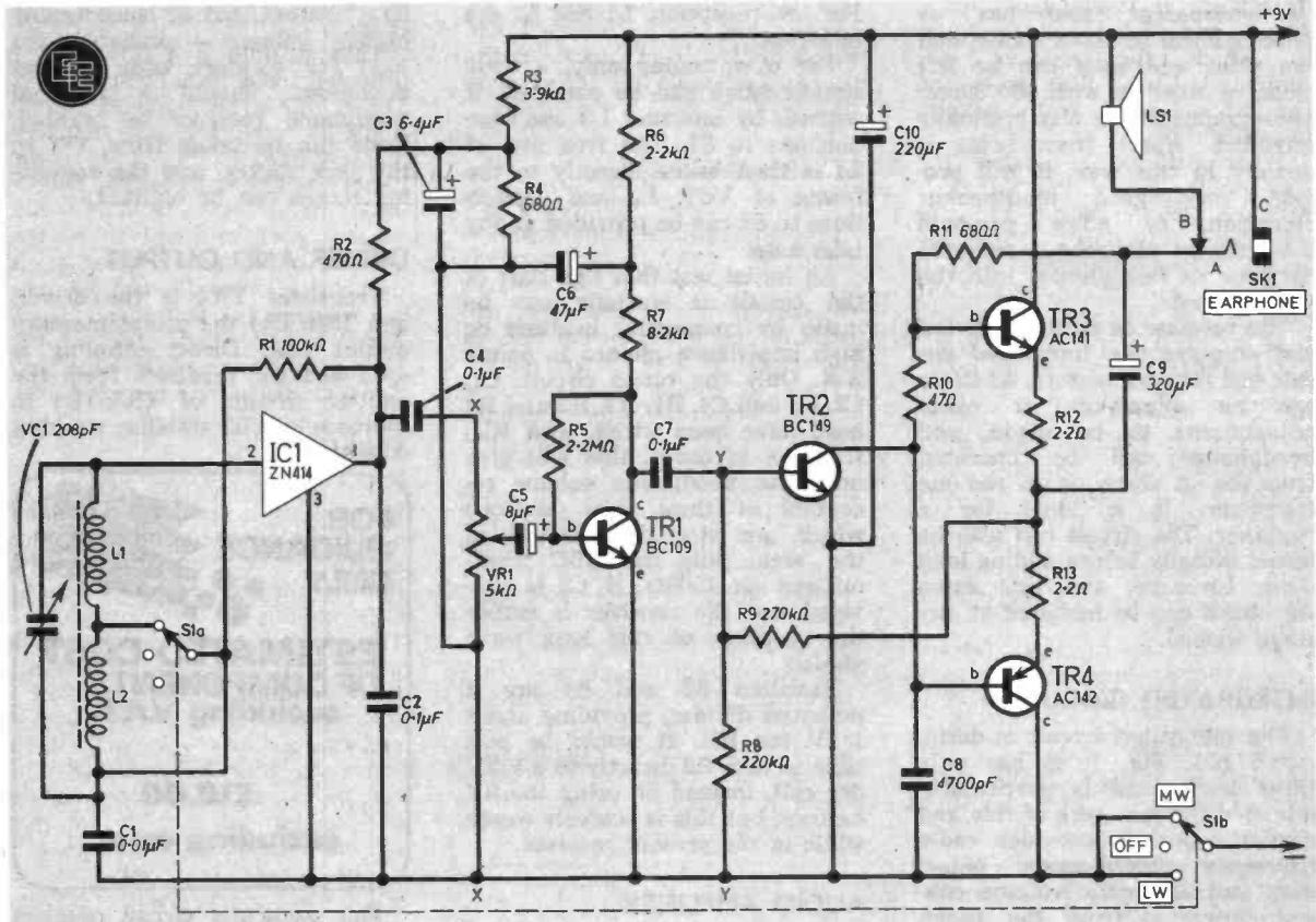
Fig. 1. The circuit diagram of the Photocube Receiver.
