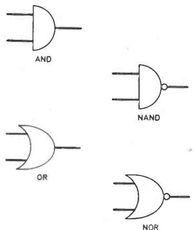
The symbols you show are to the MIL STD 806B specification which is an American spec. used by some i.c. manufacturers. Our symbols for the gates you show are in accordance with BS 3939 section 21 which is the relevant British standard specification. Maybe you work for an American company?
