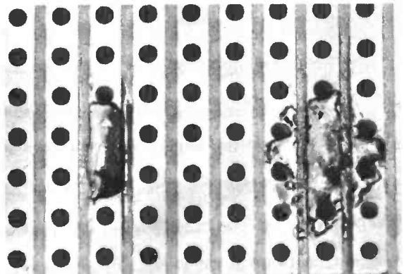
**7** On the left how a good joint should look. On the right a mess made by using too much solder and keeping the iron on too long, burning off all the flux.
