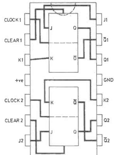
Fig. 4.2. Pin connections of the 7473 integrated circuit.
