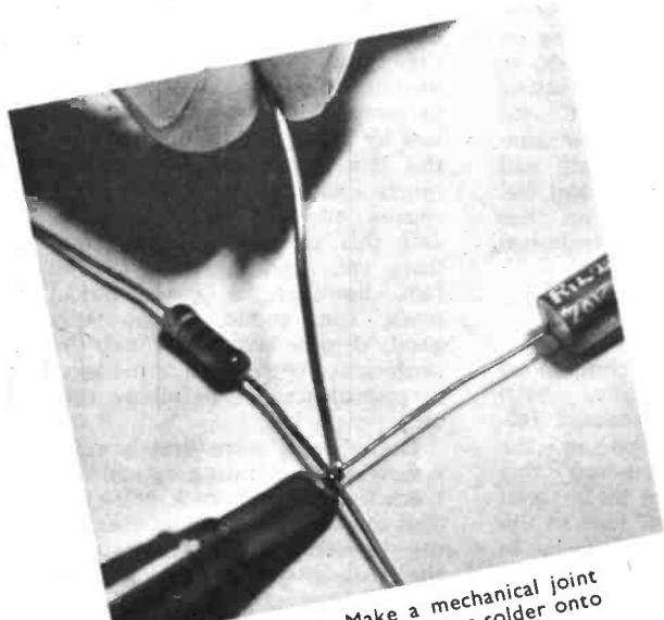
**8** Joining two wires. Make a mechanical joint first then proceed as in 5, melting solder onto the wires not the iron.
