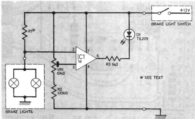
operational amplifier are derived from potential dividers across the supply lines. An adjustable reference voltage is produced by means of the divider action of R2 and VR1 in series. The input to pin 3 being taken from the wiper of VR1. The latter is used for limited fine adjustment. With VR1 set to midway position there is about 11.5 volts on pin 3.
