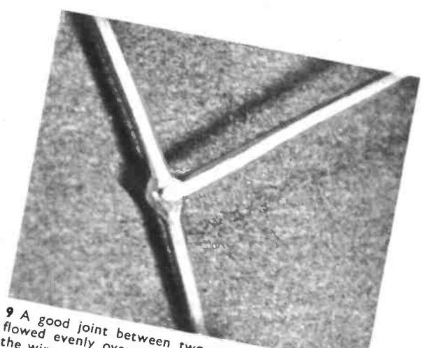
**9** A good joint between two wires, the solder has flowed evenly over the area, but not too far along the wires, and is clean and bright.
