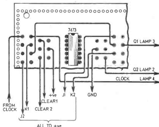
Fig. 4.4. Wiring of both flip-flops in the 7473.
