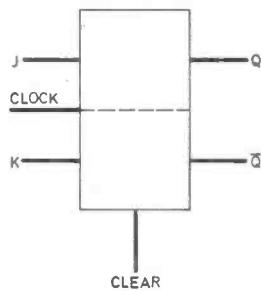
Fig. 4.1. Symbol for the J-K flip flop.
