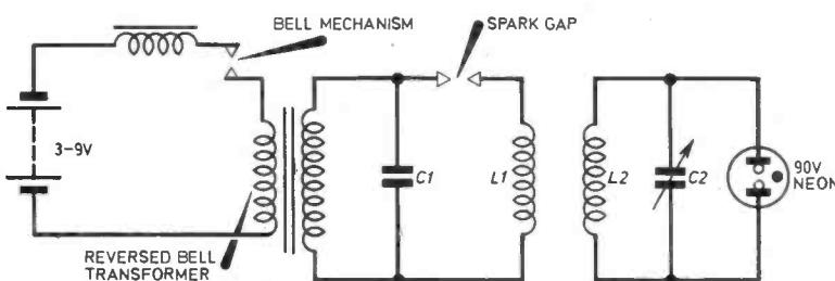
Fig. 1. The circuit of the spark equipment.
