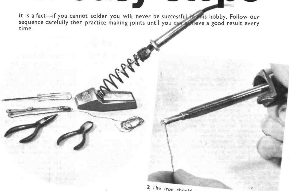
1 You will need a lightweight soldering iron with a 3 to 5mm bit, some flux cored solder and a few general tools.
