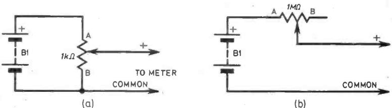
Fig. 3. Connections for testing the Multi-Tester.
