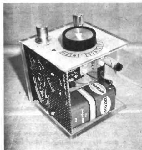
speaker. The front was backed by a piece of 2mm paxolin, 90 × 90mm, and with matching holes, to which the speaker was cemented. Three 6BA bolts and the jack outlet secure the paxolin in position.
