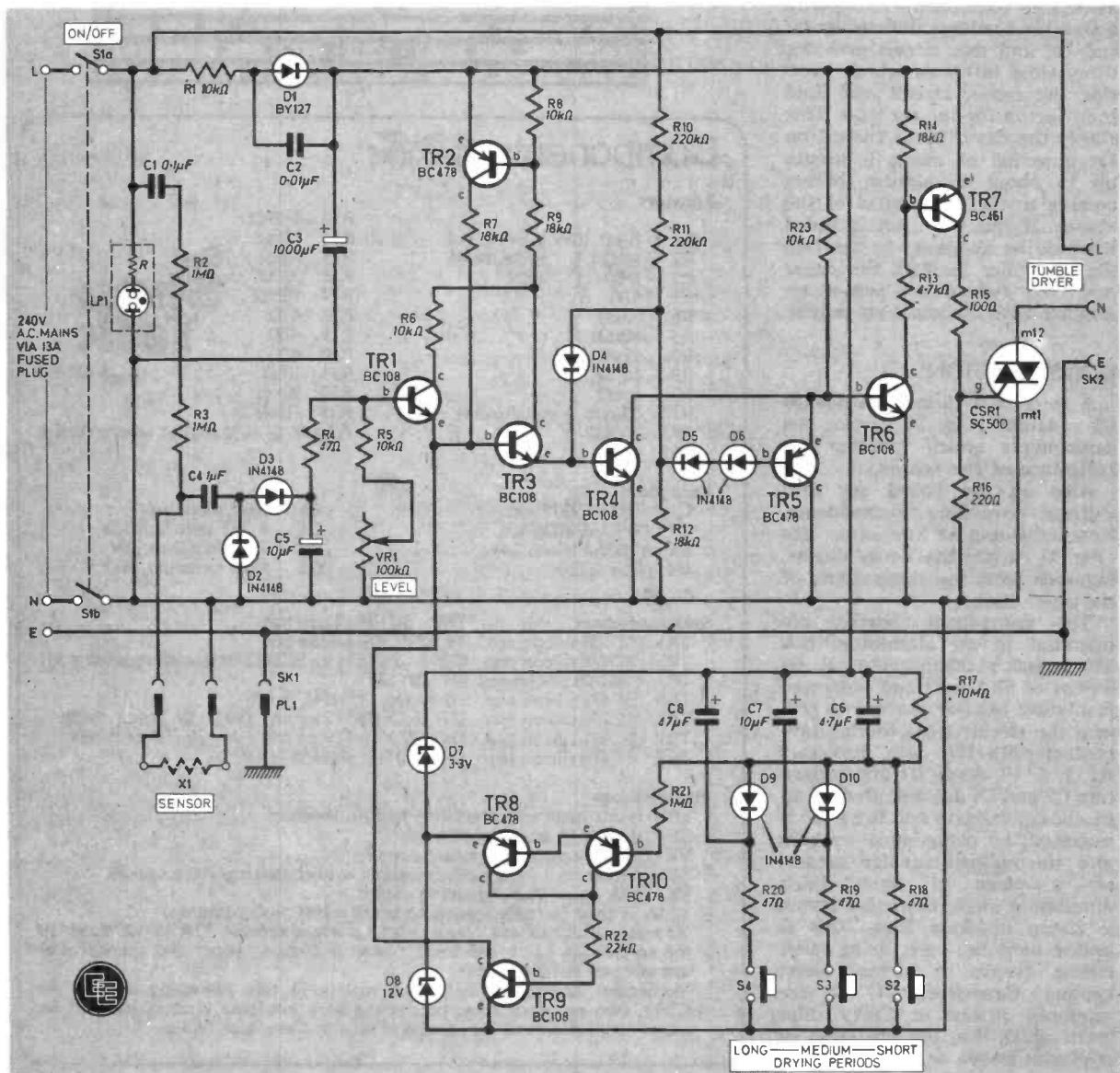
Fig. 3. Layout and wiring of the main circuit board.
