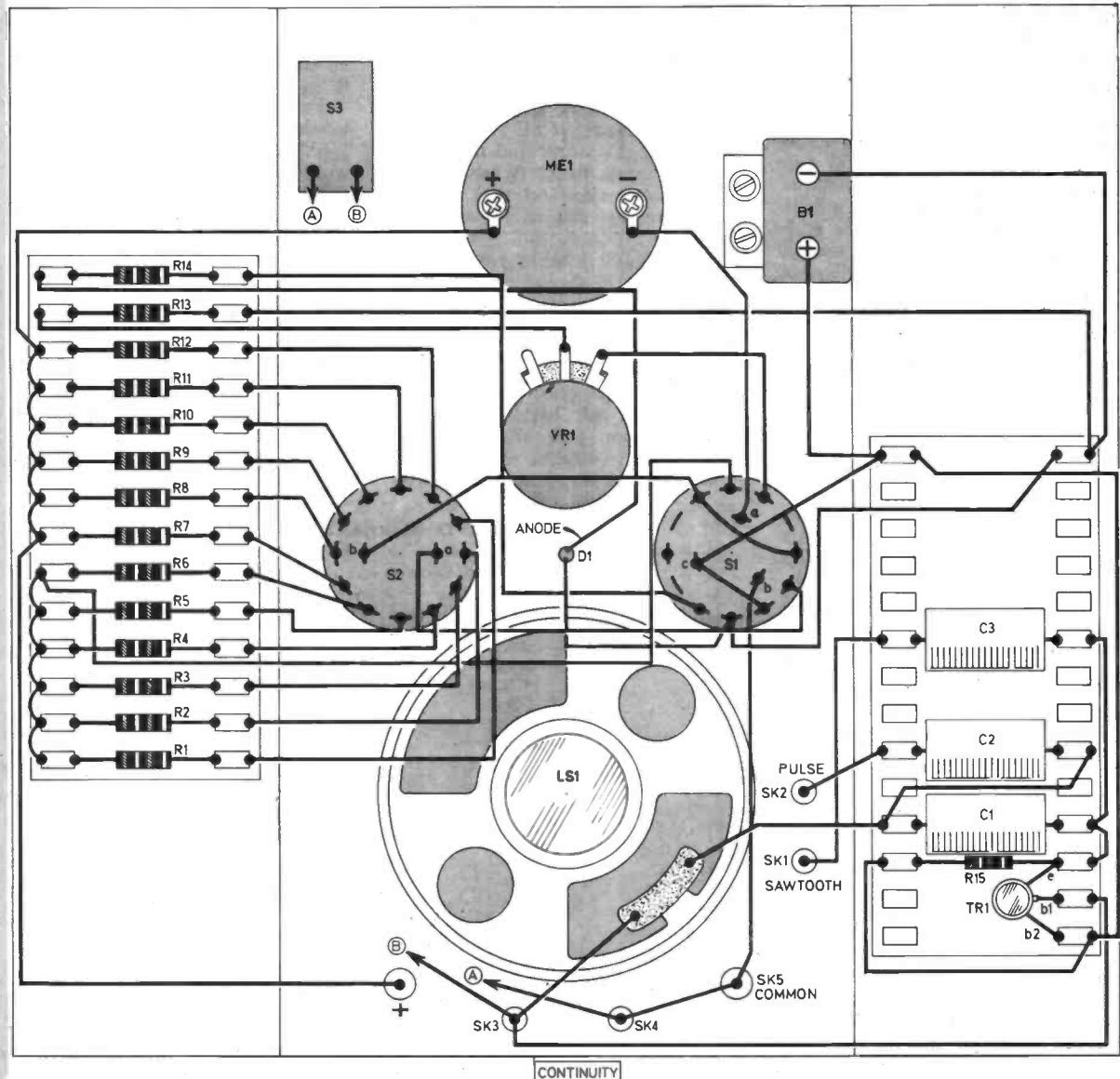
Fig. 2. Construction and wiring of the Multi-Tester.
