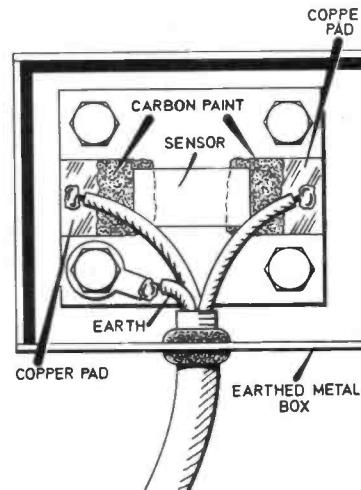
according to Fig. 1. It employs a piece of printed circuit board for mounting the sensor paper, with graphite conducting paint used to make the connections between copper and sensor, to avoid corrosion.
