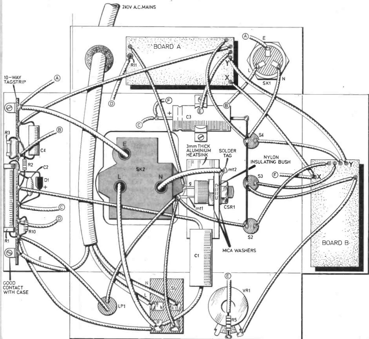
Drill and cut the aluminium box to accommodate the 13A socket SK1, the sensor socket SK2, humidity control VR1, on/off switch S1, the neon indicator, the three push-buttons S2, 3, 4, and the internal component mountings. Before fitting the 13A socket, connect to L, N, E using 13A single cable flex, as it is usually awkward to wire after fitting. Fit the 13A socket, then 3A mains cable using a p.v.c. grommet, and clamping the cable securely by means of a cable clamp.
