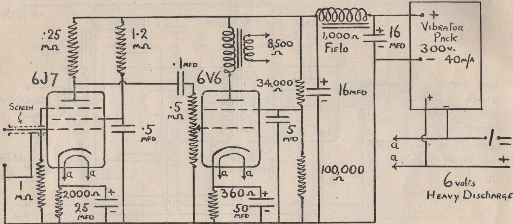
NO. 4. 4 WATT BATTERY (VIBRATOR) AMPLIFIER
