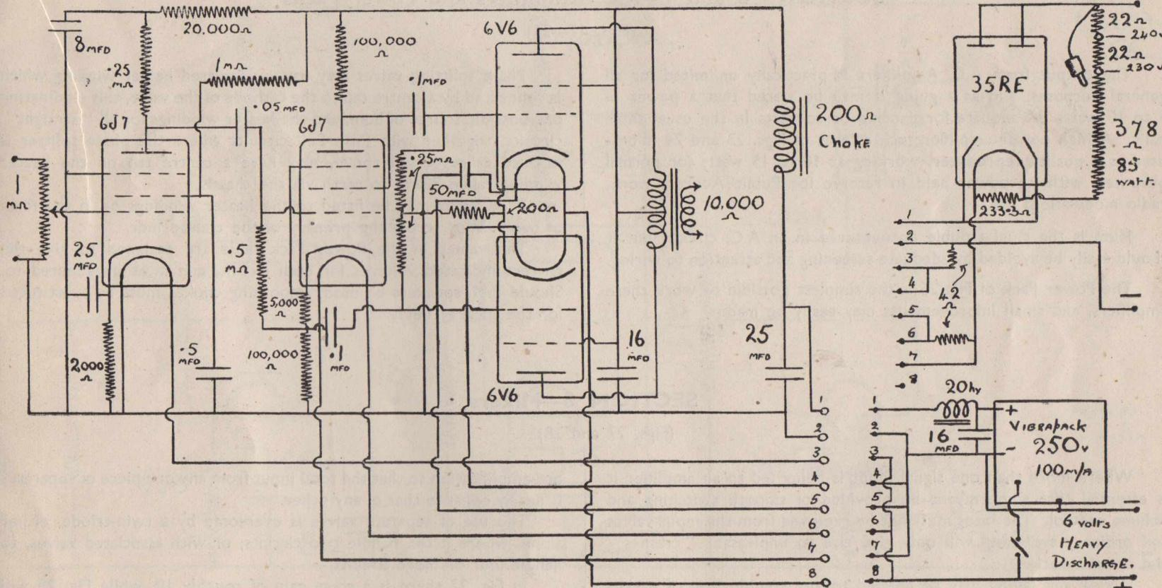
No. 16. - A.C./D.C./BATTERY AMPLIFIER, 8 WATTS
