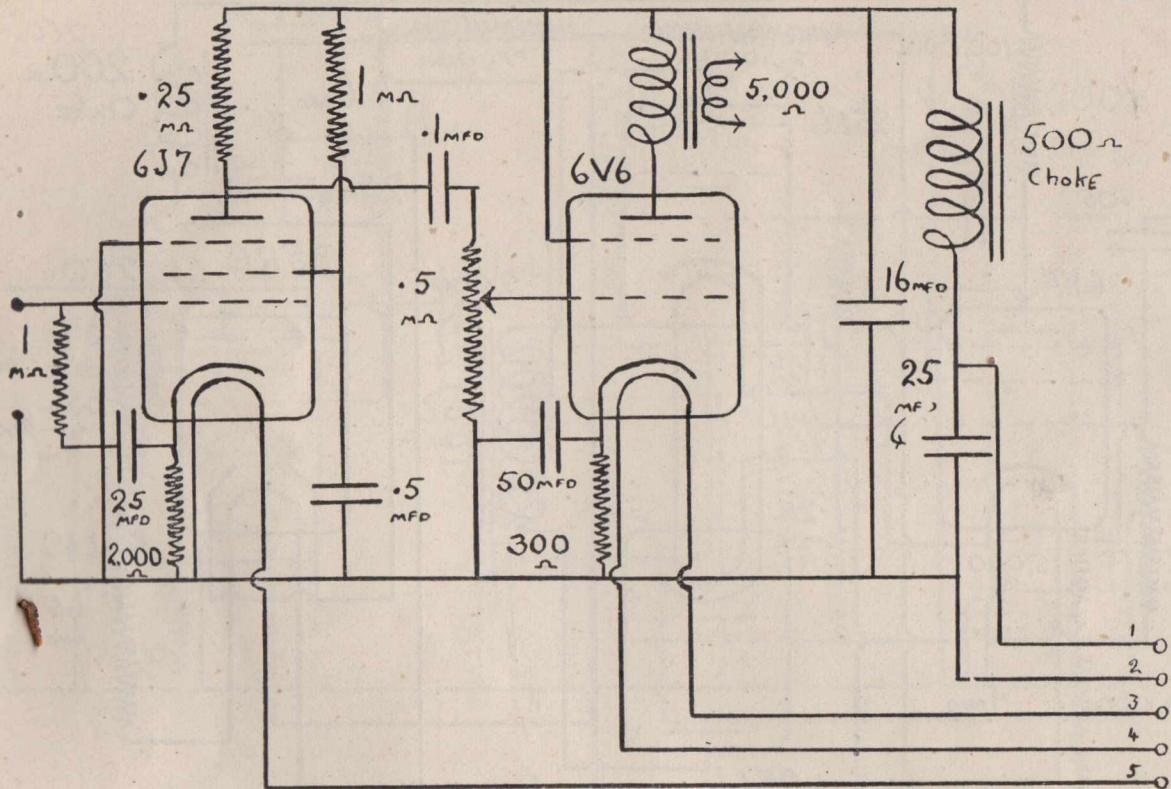
NO. 15. A.C./D.C./BATTERY AMPLIFIER, 3-4 WATTS
