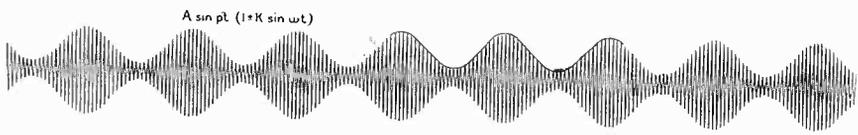
by moving the signal wave along the frequency base by the amount of the H.F. carrier. In addition to this a reversed image spectrum is created on the lower side of the carrier as is shown in Fig. 2B, from which it can be seen that the high frequency spectrum is roughly twice the width of the signal band.
