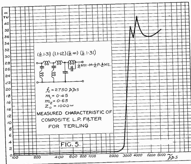
The derivation of such a type of section is rendered easy by the use of a parameter " $m$ ," which is determined from a knowledge of the frequency of cut-off and the frequency at which infinite attenuation is required. The properties of the
