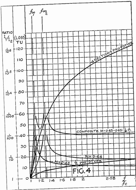
In passing, it should be noted that  $f_c$ , the frequency of cut-off does not mean that at the frequency  $f_c$  attenuation is present. In an ideal filter  $f_c$  is the boundary at which the pass region ends and the attenuation begins; hence the attenuation starts from zero at the frequency of cut-off.
