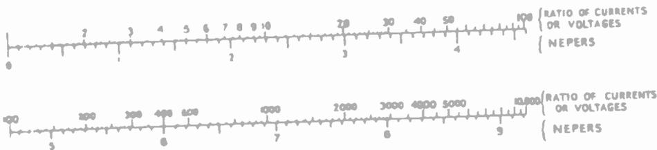
NOTE II—There is also a voltage or current ratio unit based on the Napierian or Hyperbolic system of logarithms which differs in value from the Bel and Decibel. The number of 'nepers' is obtained as follows, using hyperbolic logs
