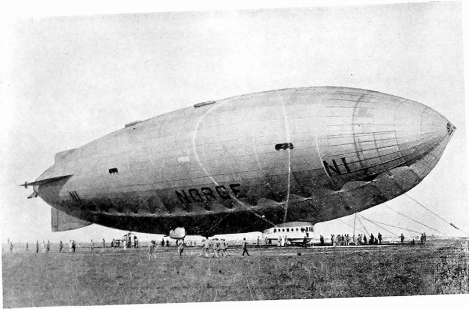
*The Airship "Norge" which was fitted with Marconi wireless transmitter, receiver and direction finder for its Arctic expedition*
