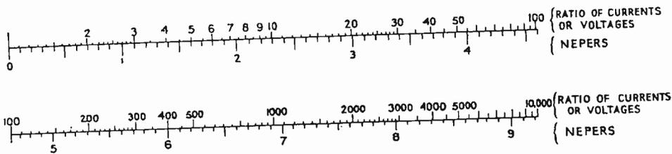
NOTE II. There is also a voltage or current ratio unit based on the Napierian or Hyperbolic system of logarithms which differs in value from the Bel and Decibel. The number of "nepers" is obtained as follows, using hyperbolic logs:—
