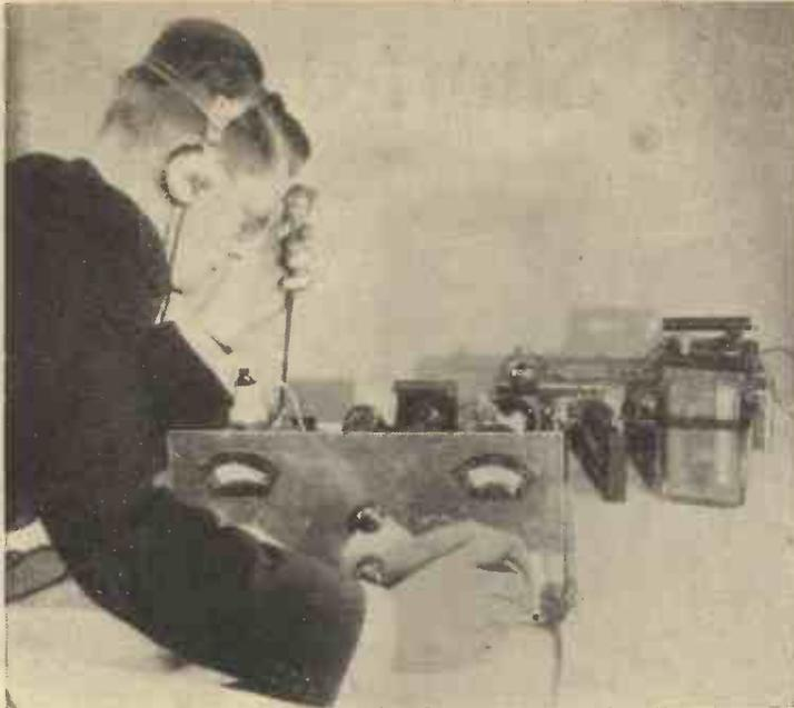
Operation of the short-wave hook-up depends very largely on a realisation that the controls must be handled very carefully—one knob for tuning, one for reaction and an optional control for grid bias
