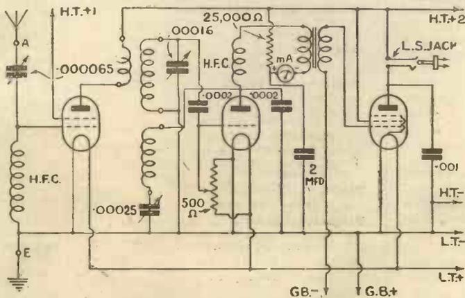
Theoretical circuit diagram, showing the untuned high-frequency stage, triode detector and pentode output
