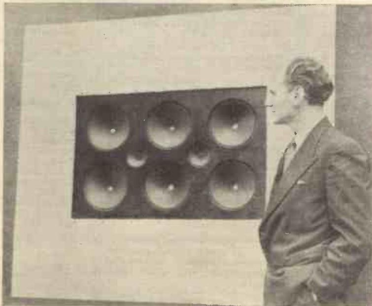
A. L. Williams, of the Brush Development Co. of America, the engineer largely responsible for the commercial development of Rochelle-salt crystals, is seen here standing by a baffle containing moving coils and piezo "tweeters" for high-fidelity reproduction
