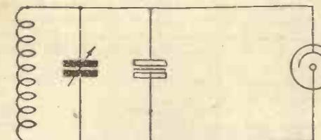
Fig. 3.—Neon-cum-crystal circuit for transmitting
