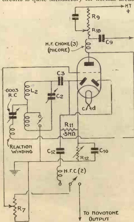
Fig. 5.—Showing how reaction may be introduced. Only the medium waves are affected
