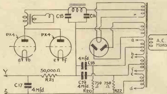
Fig. 3.—Showing the best arrangement for auto-biasing the output valves working in parallel, so as to preserve the lower frequencies
