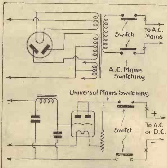
Fig. 3.—Two typical circuit applications for snap-type switches. Above is shown a double-pole on-off for mains set and below the same type of switch in a universal set where it is quite essential
