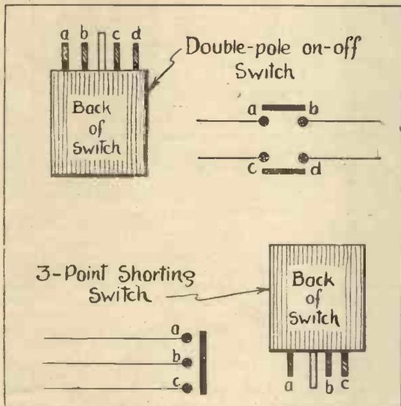
Fig. 2.—Back views of two more snap-type switches—at the top a double-pole on-off and below a three-point shorting switch for dual-range coils
