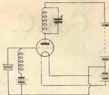
Fig. 2.—Another method of connecting a quartz crystal
