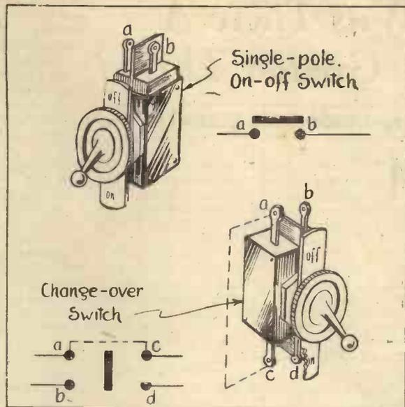
Fig. 1.—Two typical snap-type switches, a single-pole on-off and a change-over switch. Note the symbols beside them showing their mode of connection
