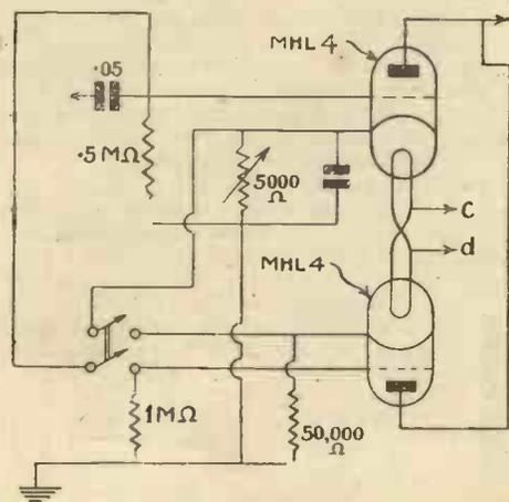
Fig. 4.—A switching arrangement by which an MHL4 valve can be, if desired, added in parallel with the MHL4 in the second low-frequency stage, thus reducing both amplification and impedance when the MHL4 is switched out of circuit; in this way practically no anode current is wasted
