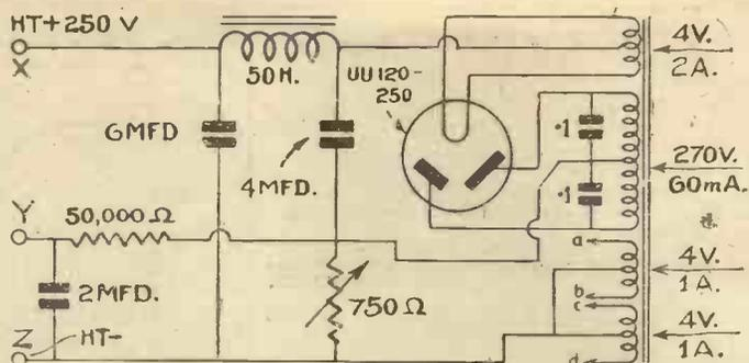
Fig. 2.—Circuit of the mains unit for the A.C. radio gramophone
