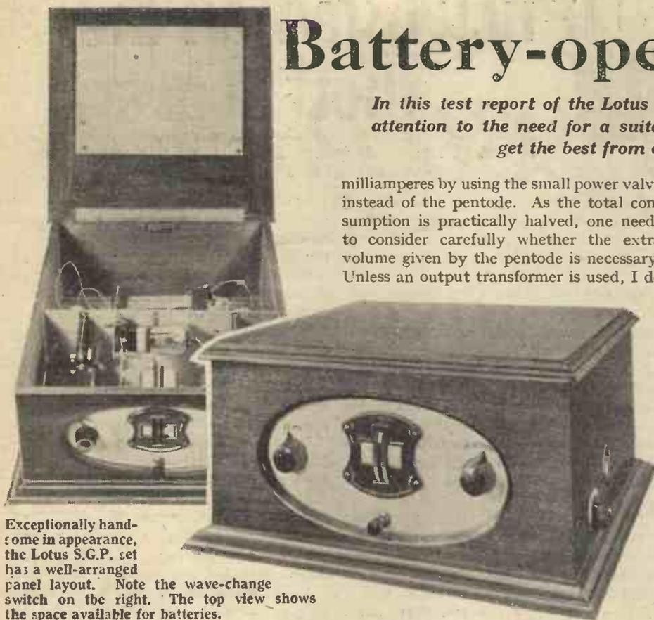
Exceptionally handsome in appearance, the Lotus S.G.P. set has a well-arranged panel layout. Note the wave-change switch on the right. The top view shows the space available for batteries.
