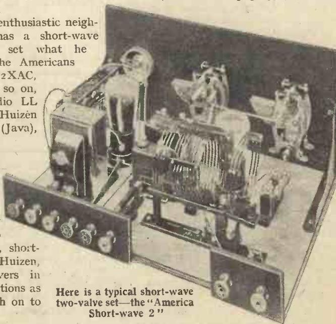
Here is a typical short-wave two-valve set—the "America Short-wave 2"
