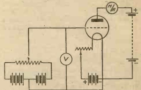
Fig. 2.—Circuit for Plotting Characteristic Curves.
