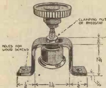
Fig. 7.—Method of Mounting Rheostat.
