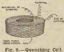
Fig. 9.—Quenching Coil.
