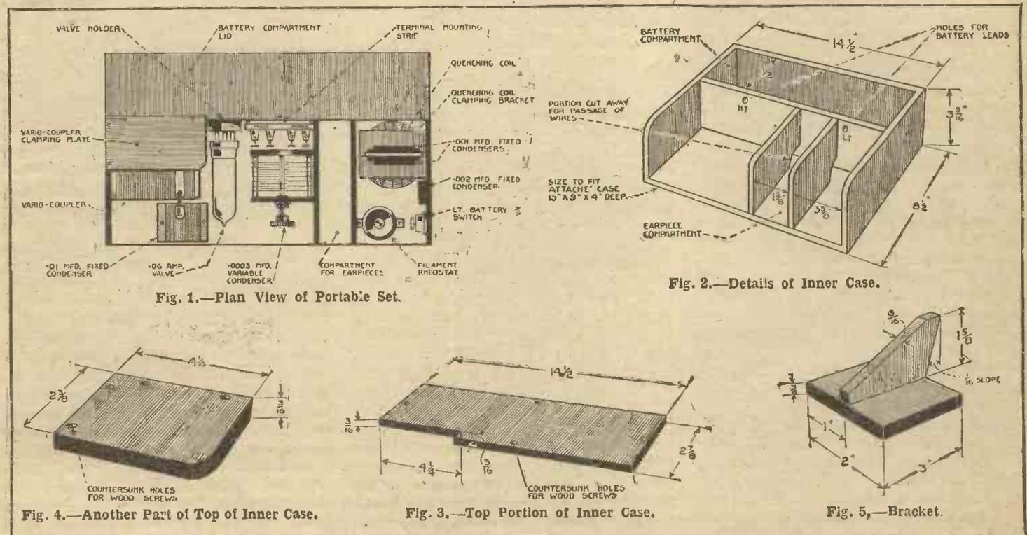
while the two .001-microfarad condensers are attached by means of wood screws to the sides of this bracket. The two remaining condensers (.01 and .002) are attached as shown in Fig. 1 to the base and side of the case respectively.
