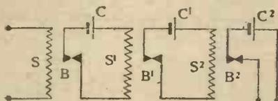
Fig. 1.—Telefunken Sound Intensifier.
