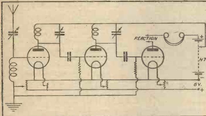
Fig. 3.—Use of Potentiometer in 3-valve Circuit.
