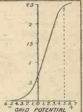
Fig. 5.—Characteristic Curve showing Rectifying Point.
