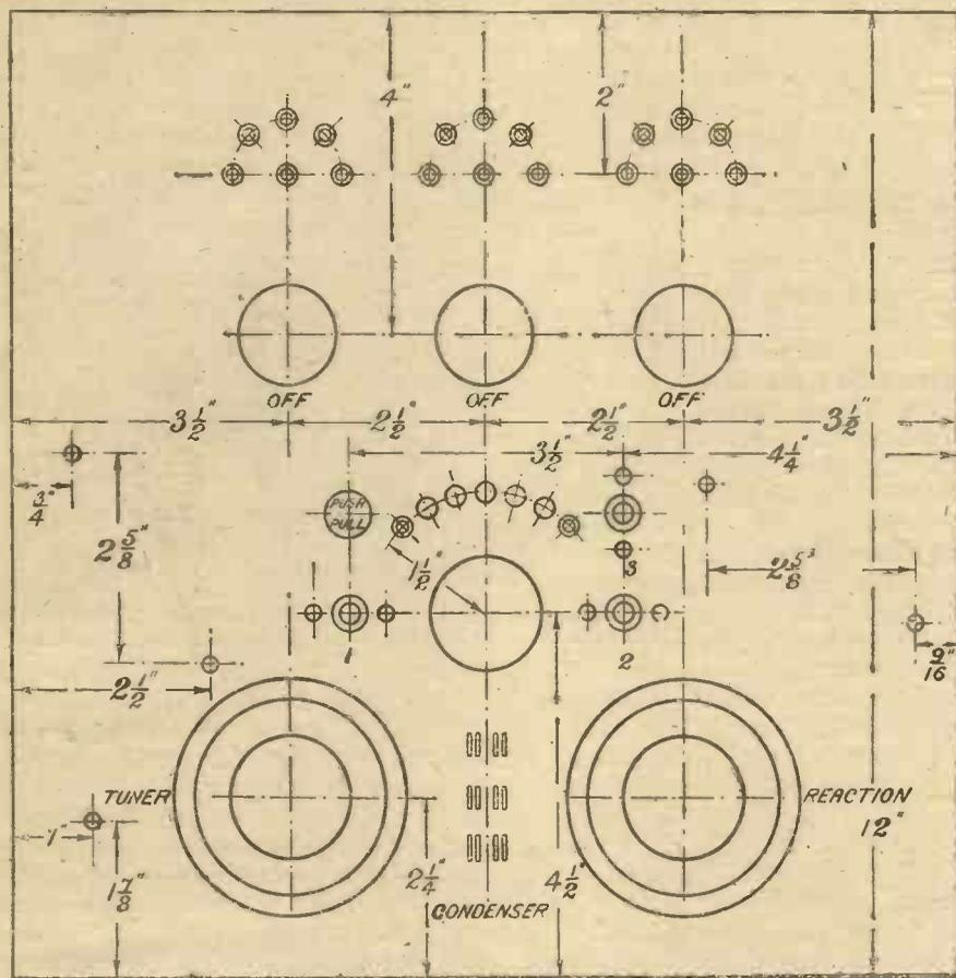
Fig. 3.—Layout of Front Panel.
