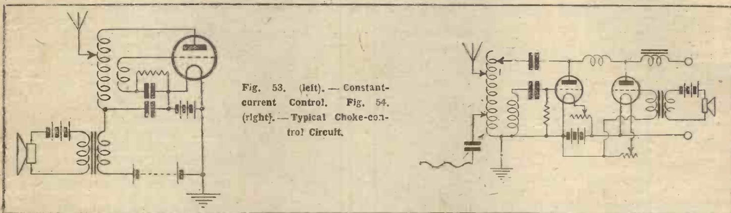
Fig. 53. (left).—Constant-current Control. Fig. 54. (right).—Typical Choke-control Circuit.
