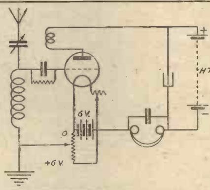
Fig. 4.—Use of Potentiometer in Single-valve Circuit.
