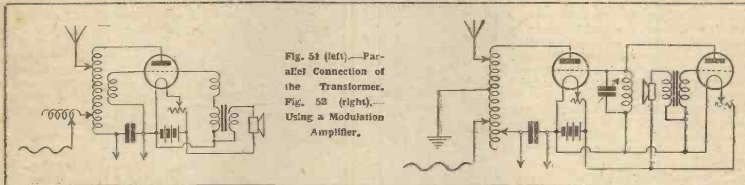
Fig. 51 (left).—Parallel Connection of the Transformer. Fig. 52 (right).—Using a Modulation Amplifier.
