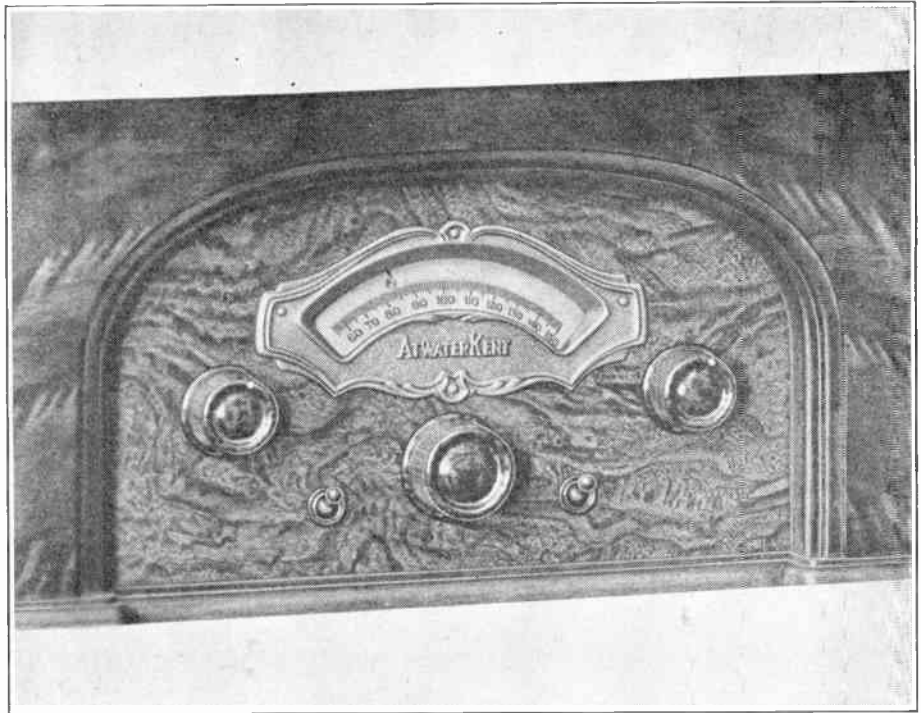
The Atwater-Kent Control Panel, showing the new and exclusive quick vision dial. Left to right—Volume control knob, local distance switch, tuning knob, on-off switch and tone control knob.
