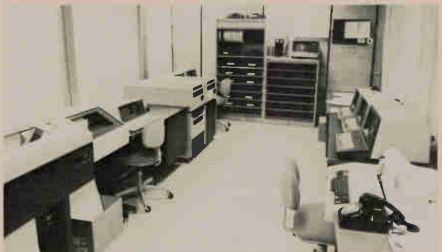
Central computing facility is devoid of mainframes or front-end processors. Series of minicomputers are tied together into flexible data network.
