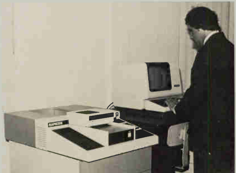
Electronic public mail in action. Correct codes are entered into computer for transmission of Intelpost message from Canada to London, England. Material to be transmitted from Canadian centres is scanned, then stored in disc memory. Digital signals representing message go via satellite to earth station in receiving country, where message is received for delivery. Intelpost operates from Edmonton, Calgary, Winnipeg, Montreal, Ottawa, Toronto and Halifax.
