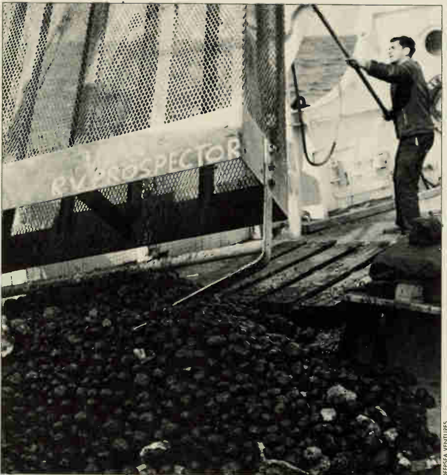
The crew of a survey ship hauls up a wire dredge basket filled with nodule samples to record their location and metal content for later ocean-mining missions.
