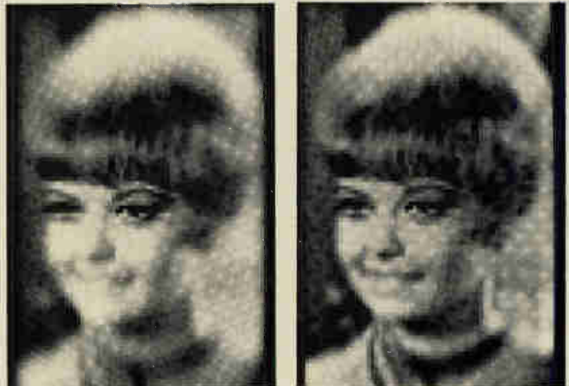
A restoration experiment where attempts are made to remove blur from the image. Restoration is from SVPSF or Space Variant Point Spread Function. At left, blurred image with no 'noise'; at right is the restored image using a quadratic programming algorithm. Mottled appearance of photo is caused by Moiré effect between individual pixels in the picture generated by the computer and the printing.
