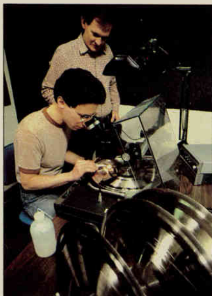
Above: Quality-control check of a mother disc is crucial in making a superrecord. Here the grooves are being microscopically examined as the disc is played. Rack holding other mothers is seen in foreground. Right: Stages in the manufacture of a record, top to bottom: lacquer master, master mold (“father”), mother, stamper, the final disc, and raw vinyl from which the final disc is pressed.
