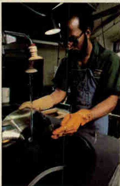
Far left: A technician leans over a cutting lathe to check the grooves with a microscope as a master is cut. Top: The master mold is prepared for plating to produce the mother. Left: The newly made mother is separated from the master mold after plating. Above: The mother disc is washed with a special goat-hair brush before the next plating step. Similar cleaning precedes all stages that require plating.
