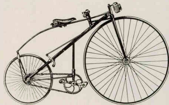
Left: An 1888 issue of Bicycling World commemorated Thomas Stevens, whose Expert Columbia took him across America in 1884 and around the world by 1887. Top: The Acatene chainless safety of the 1890s was as sturdy as the operatic woman advertising it. Middle: By using a crank axle with chains and sprockets, the wheel size of the 1885 Kangaroo could be reduced. Bottom: Lawson's safety Bicyclette of 1879 pointed the way to modern bike design.
