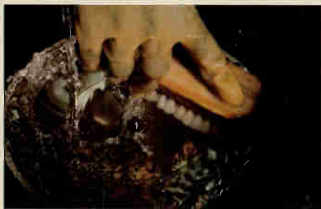
Far left: A technician leans over a cutting lathe to check the grooves with a microscope as a master is cut. Top: The master mold is prepared for plating to produce the mother. Left: The newly made mother is separated from the master mold after plating. Above: The mother disc is washed with a special goat-hair brush before the next plating step. Similar cleaning precedes all stages that require plating.
