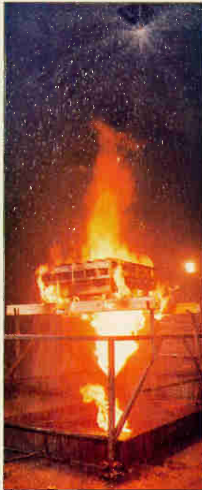
Left: A sample of appliances tested in the electrical lab. Above: Sprinklers spray a burning crib of wood for half an hour; if the wood retains 80% of its weight and the ceiling temperature doesn't rise more than 530°F, they pass this test for controlling a fire.
