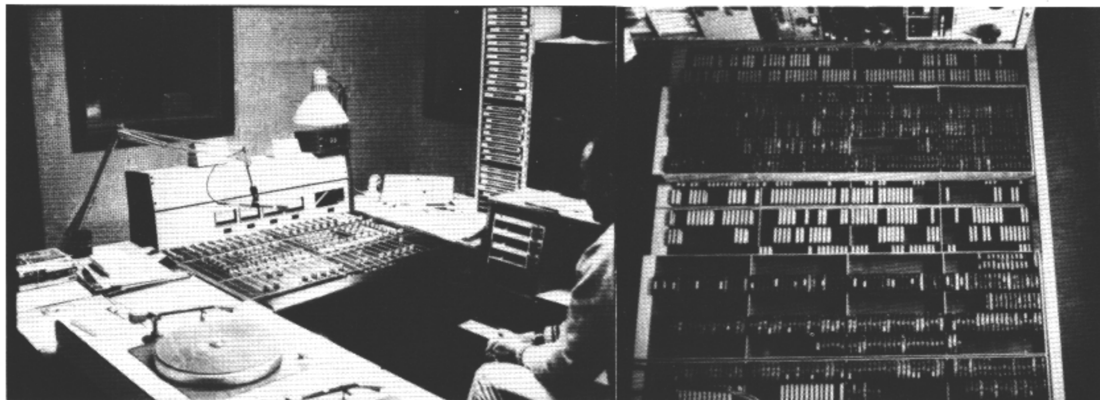
CFRA production studio is equipped with Auditronics 4-channel console, McCurdy turntables. At right is cartridge storage unit in CFRA master control.
