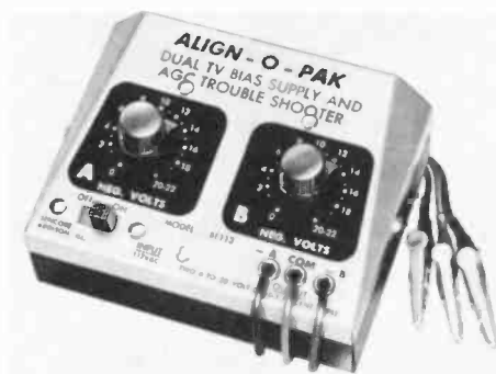
Fig. 209—A high-impedance bias box is useful to clamp agc lines and restore normal voltages for test.
