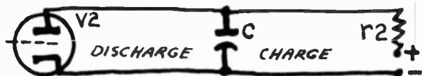
This is the elementary charge-discharge circuit as it would appear if it were removed from the multivibrator.
