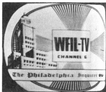
Fig. 7-H. Photo shows example of horizontal nonlinearity.
