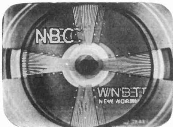
Fig. 1-J. Example of horizontal jitter.
