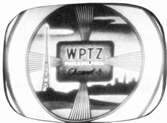
Fig. 2-B. Vertical wedges show severe bending.
