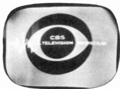
Fig. 3-L. Low-voltage B+ causes reduction in height and width.
