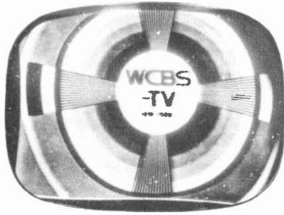
Fig. 3-C. Pix is improperly centered due to intermittent horizontal shift.
