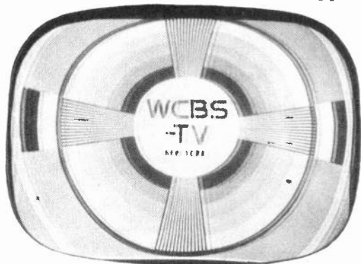
Fig. 5-R. Pix of test pattern shows echo.
