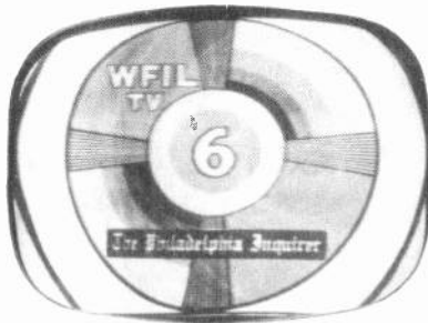
Fig. 3-D. Poor pix detail because of loss of higher video frequencies.
