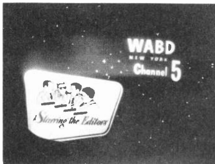
Fig. 1-D. Poor dc restoration results in a gray picture. Dc restorers are found in old receivers, many of which are still in use.
