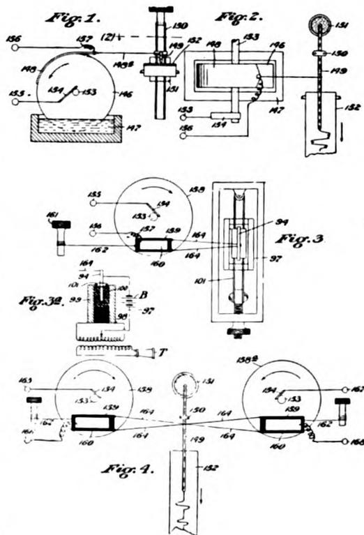
gram of an amplifier or relay. Fig. 4 is a similar view of a modified form in which pressure effects are balanced and operate differentially to produce a more sensitive instrument.
