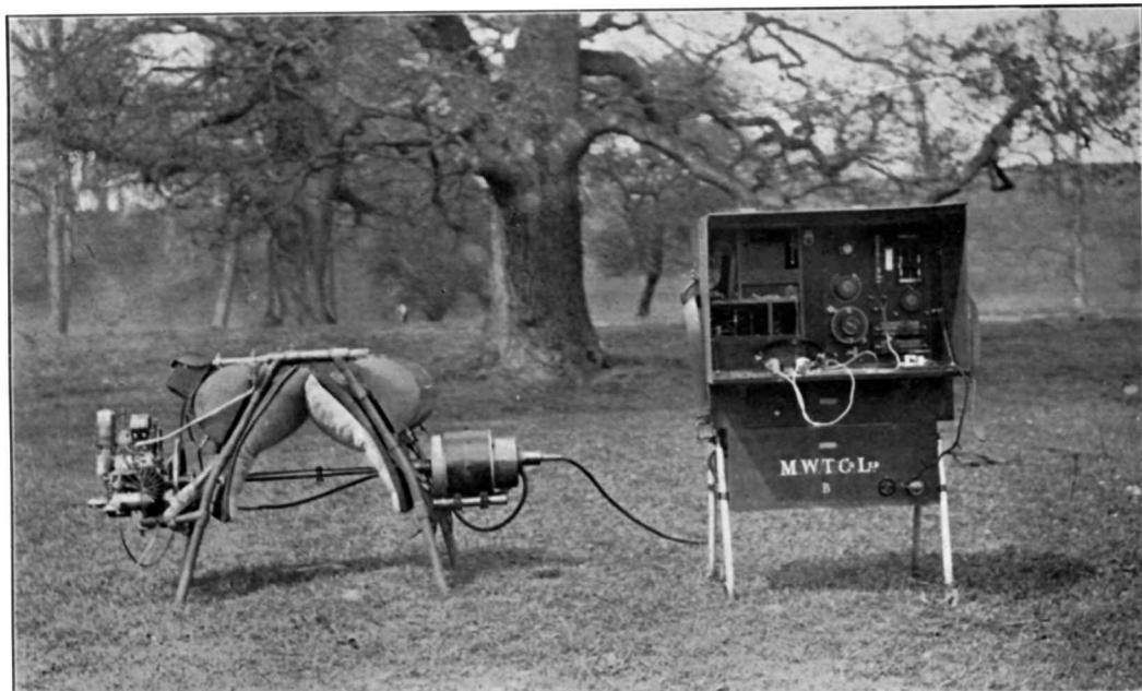
*A Marconi Cavalry Pack Set, comprising Engine and Dynamo, Transmitting and Receiving Apparatus.*
