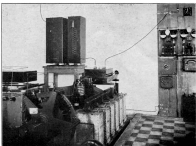
*The Rotary Spark Gap, Oscillating Transformer, and Inductances.*
