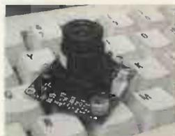
The A-721-S Micro-video camera with lens outputs composite video and costs just £65\*
