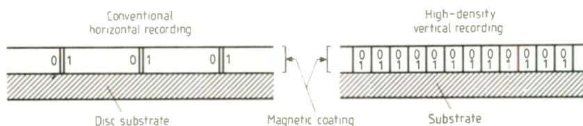
Vertical recording places the domains in the vertical direction increasing data packing density substantially. This technology promises to extend the usefulness of conventional magnetic media
