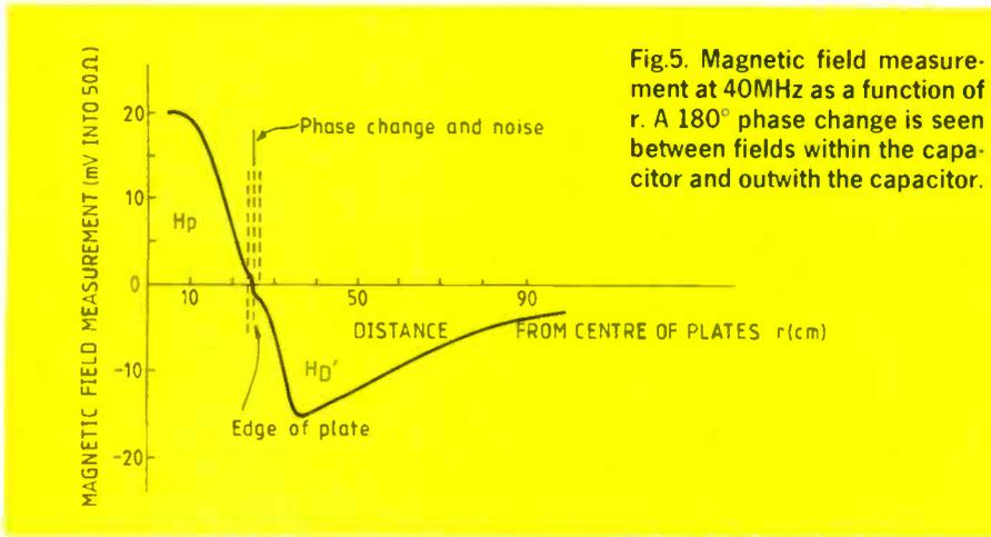
Fig.5. Magnetic field measurement at 40MHz as a function of  $r$ . A  $180^\circ$  phase change is seen between fields within the capacitor and outwith the capacitor.
