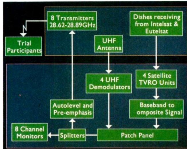
Fig.5. BT M<sup>3</sup>VDS system parameters.
