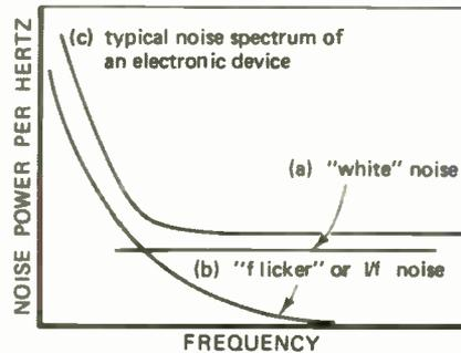
fluctuations in the spatial and energy distributions of the charge carriers. Simple mathematical treatment suggests that shot noise is also white and that the mean square noise current per unit bandwidth associated with a current of mean value  $I$  is given by
