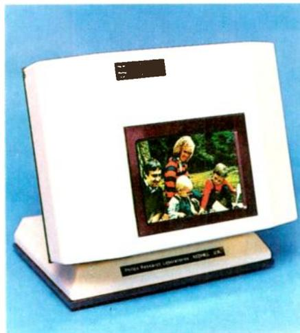
Flat-screen full-colour televisions should be available this year – this prototype was made by Philips researchers at Redhill.
