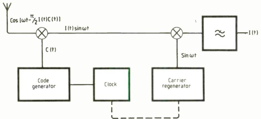
Fig. 3. Basic receiver for a DS spread system.
