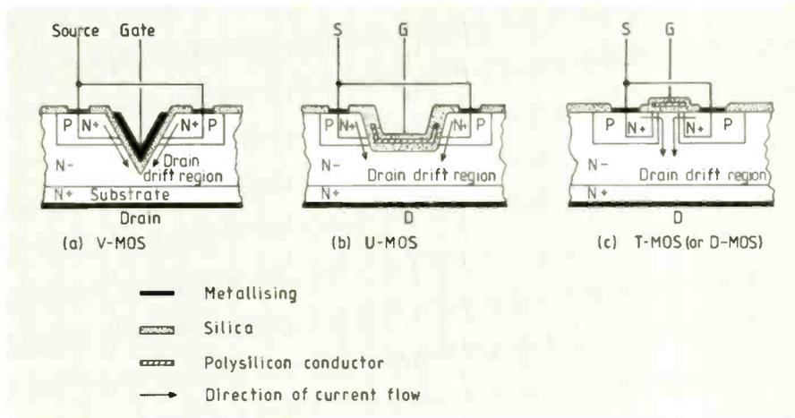
Fig. 2. Three forms of the power mosfet.
