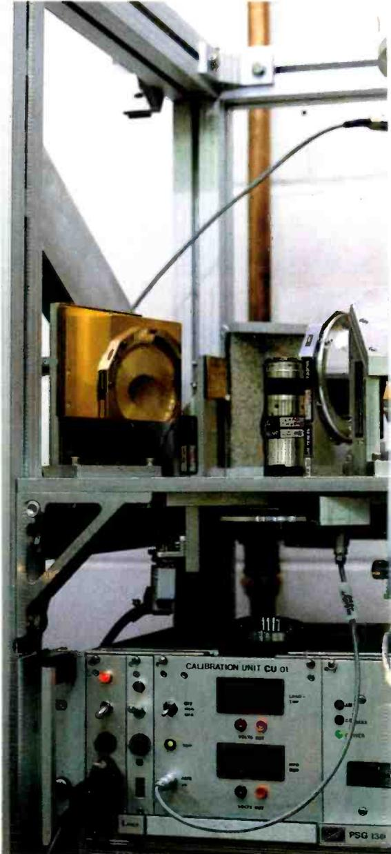
**Close up of the 460-490GHz receiver.** The gold-coloured vacuum vessel (above) houses two InSb homodyne detectors for two polarizations of the incoming signal. They are cooled to 0.2K above absolute zero using liquid-helium refrigerant.
