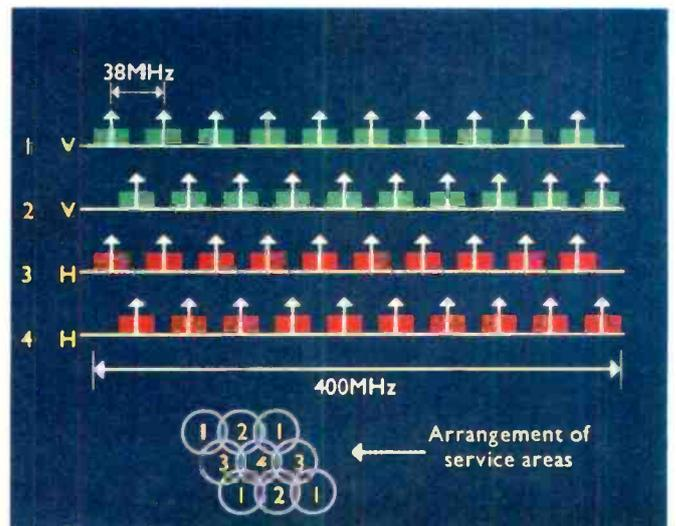
Fig.4. FM 10-channel MVDS plan with lattice arrangement.
