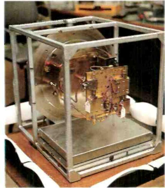
**Superconducting receivers.** The Radio Astronomy group at the Cavendish Laboratory is developing, in collaboration with the Materials Science Department, superconducting receivers for use on the James Clerk Maxwell Telescope in Hawaii (right).
