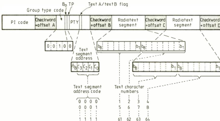
Fig.9. Decoding RDS groups: this one is type 2A.
