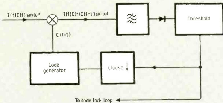
Fig. 4. Signal acquisition in a DS spread system.
