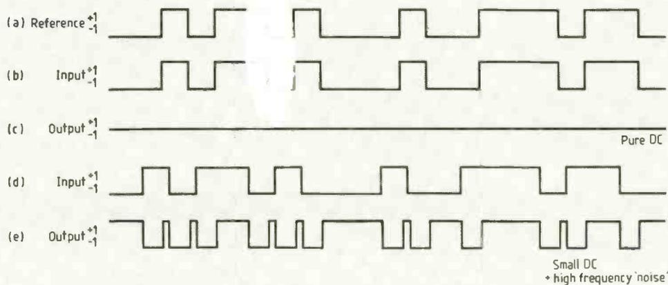
Fig. 1. Correlation process. Waveform(e) is the product of (a) and (d).
