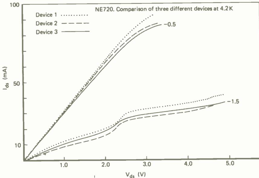
Fig. 5. Comparison of the characteristics at 4.2K of three individual devices of the same type (NE720) for two different values of gate bias. The dotted, dashed and full lines respectively represent the three devices.
