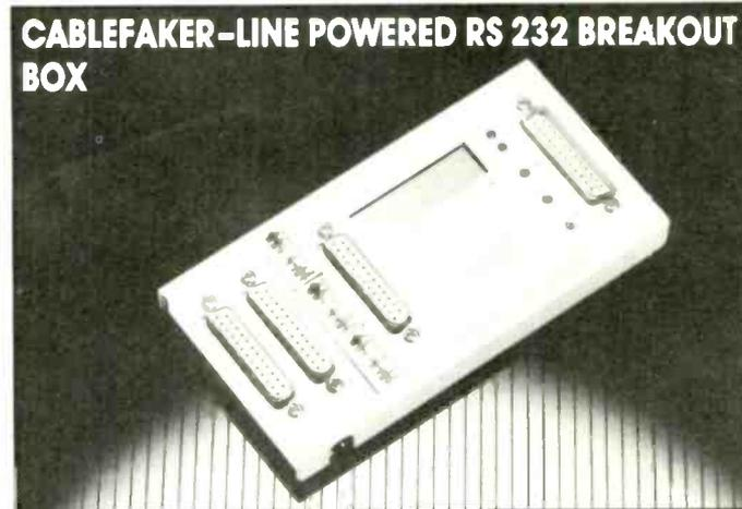
Featuring a custom LCD which uses easily recognisable mnemonics for the signal states, the Cablefaker offers a complete RS 232 breakout and patch facility, yet costs only £74.95.
