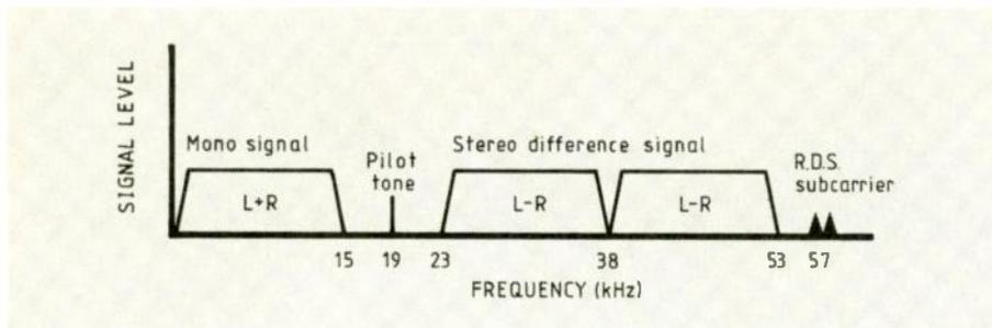
Fig.8. Spectrum of the multiplex signal.
