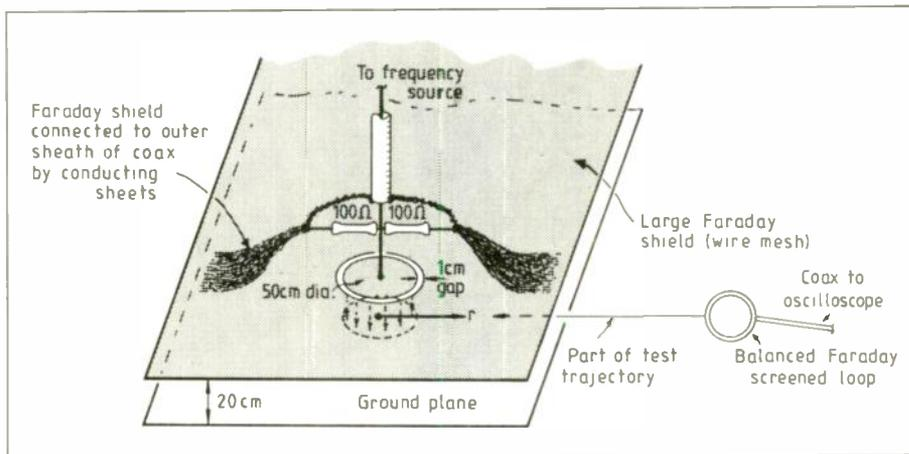
Fig. 3. Experimental set-up to measure the magnetic field surrounding "large circular capacitor plates.
