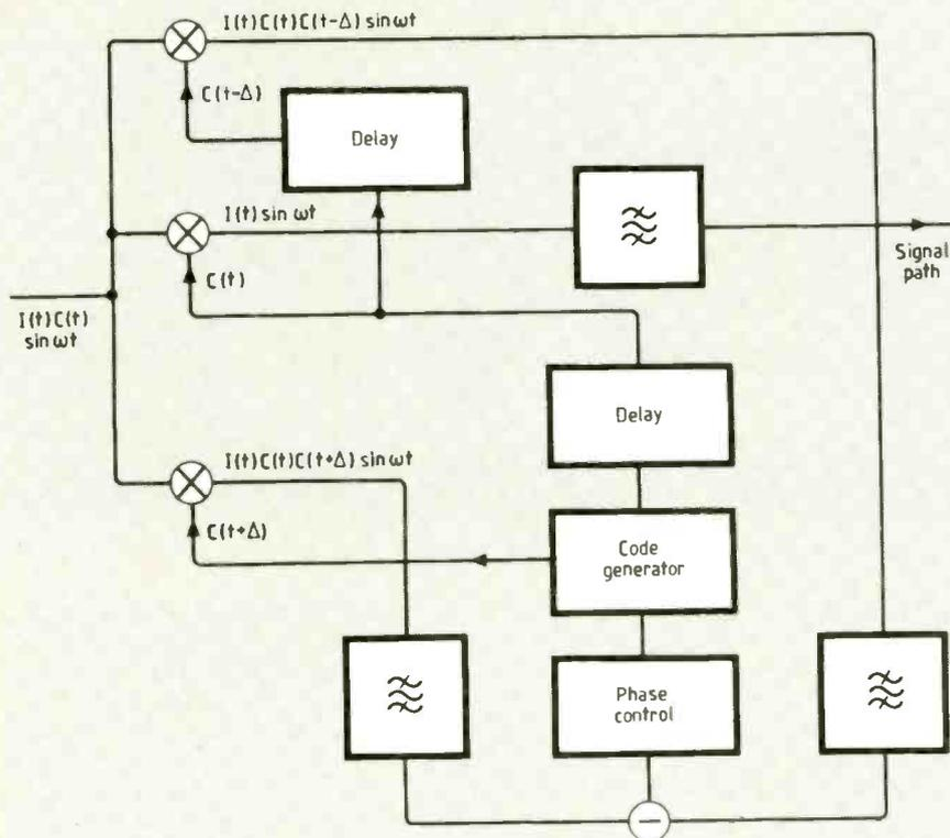
Fig. 5. Code lock loop. This generates three versions of the local code, slightly shifted in time or phase.
