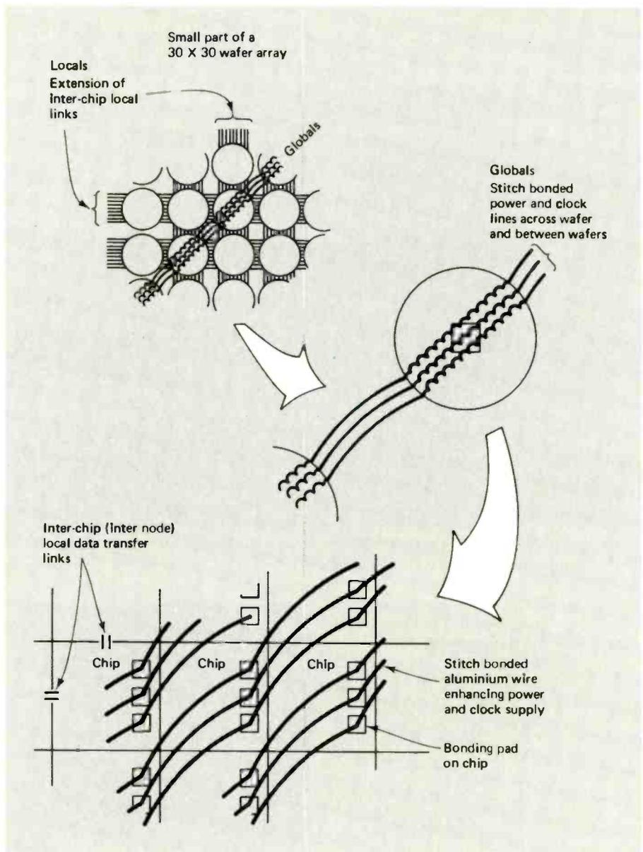
ideal for the purpose. At a cost which is only a fraction of the cost of the processed wafer, parallel columns of aluminium wires can be stitched across the wafer, reducing the effective resistance of the aluminium track beneath. The yield on such stitch bonding is very high, and faults, on the rare occasions when they do occur are to a harmless open circuit to the bonding pad (the aluminium
