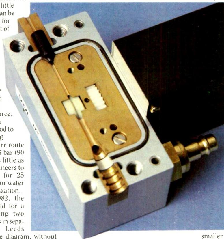
*Rudimentary blowing 'head' used in the Leeds trial (below) is superseded by BT's patented design above, which enabled a spliceless link of 3.2km.*
