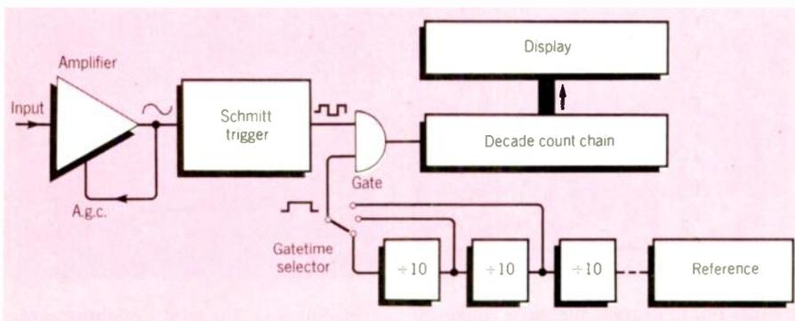
Fig.1(a). In the basic frequency counter, the input signal is squared up by the amplifier and Schmitt trigger and counted for a pre-determined gate time. Resolution is  $\pm 1$  input cycle.
