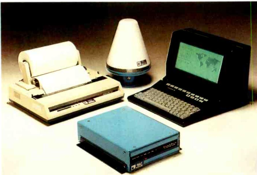
*This Standard-C electronics unit measures 73 × 214 × 279mm and weighs in at 2kg. Any computer or printer with RS232 interface can be used. Inmarsat say that the cost of equipment will be less than US \$5000; in full production it should be much less. Makers will be Racal, Danish company Thrane & Thrane, JRC in Japan and Sperry in USA.*
