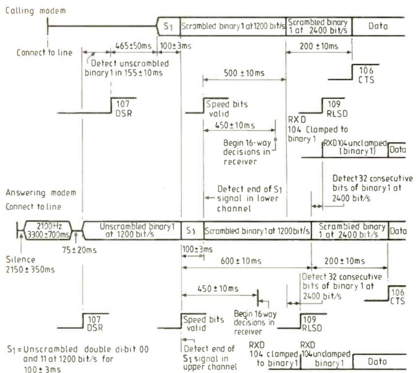
Fig.5 (above). V.22 modem connect sequence (1200bit/s). Three-figure numbers refer to RS-232 (now properly EIA-232) circuit numbers.
