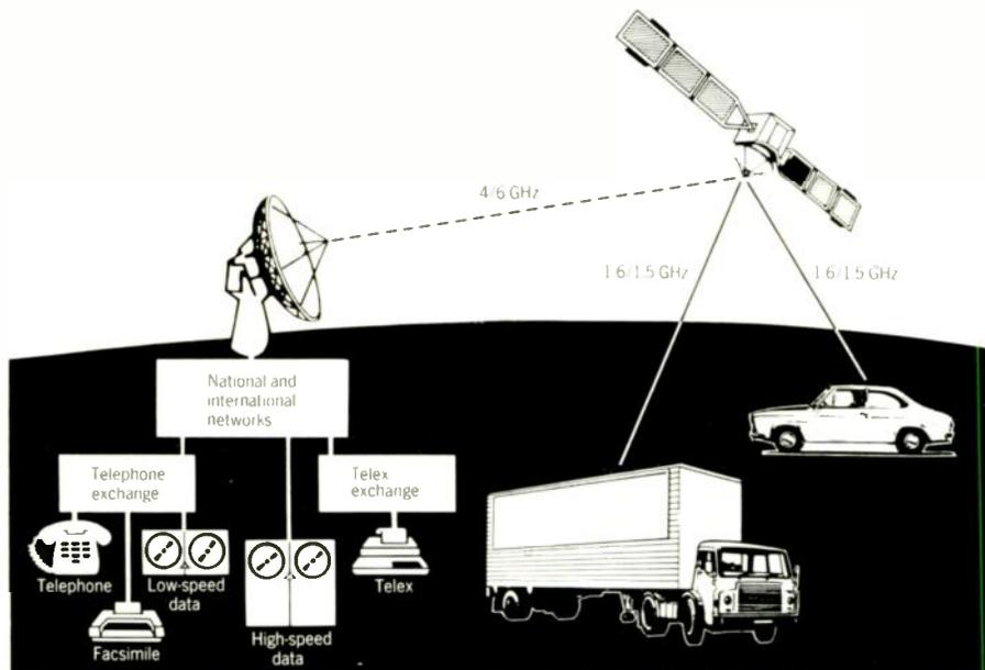
*The Inmarsat system consists of three basic elements: the mobile equipment consisting of transceiver, terminal, printer, a communications satellite and a fixed earth station. The earth station provides interface with the international telecommunications network.*
