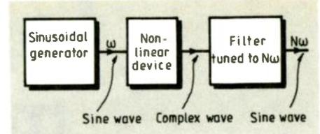
Fig. 2. To multiply some waveforms, a sine wave for example, a non-linear device has to be used to introduce the desired multiplication harmonic.
