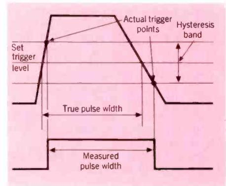
Fig.4. Too small a hysteresis band introduces additional complications due to premature triggering on noise peaks.
