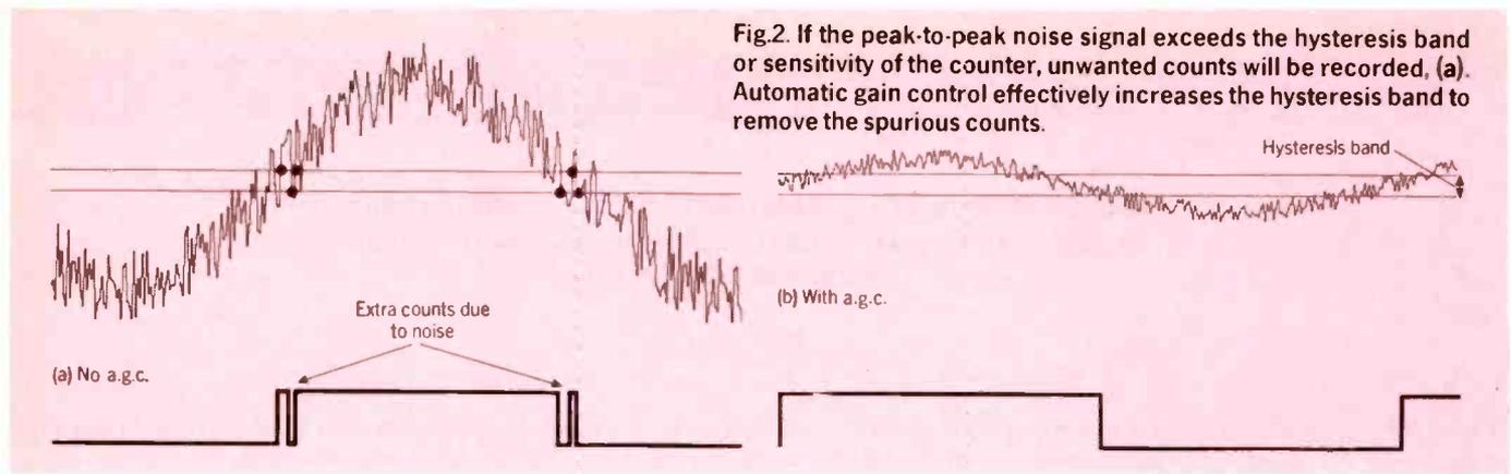
Fig.2. If the peak-to-peak noise signal exceeds the hysteresis band or sensitivity of the counter, unwanted counts will be recorded, (a). Automatic gain control effectively increases the hysteresis band to remove the spurious counts.
