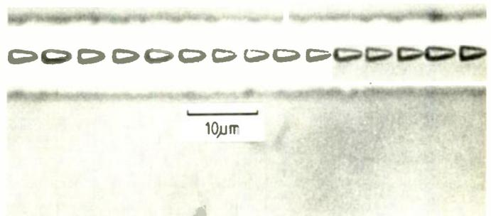
Core region of a fibre after damage, showing oxygen-filled cavities a few wavelengths across.
