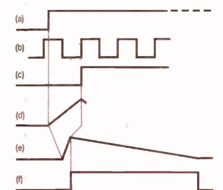
Fig.7. Analogue interpolation increases the resolution of a timing measurement to well beyond the natural limit of the timebase period. The time difference between the 'start' signal, (a), and the next active clock edge used to open the gate, (c), is converted into an analogue voltage by the integrator, (d), which is then discharged at 1% of the charge rate and the discharge time is measured, (e). The result is divided by 100 and added to the conventional measurement.
