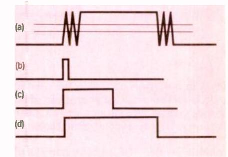
Fig.6. Trigger hold-off is used to overcome the problems of noise or contact bounce. Attempts to measure the signal shown at (a) will result either in extra counts or the short interval in (b). Trigger hold-off uses a monostable period, (c), to inhibit the signal during bounce time to produce the required measurement, (d).
