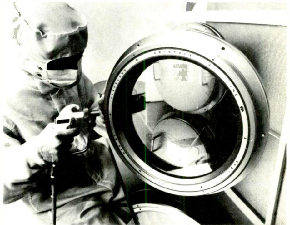
The largest frequency doubler is used in plasma physics and laser fusion experiments with the world's largest lasers. This is a single perfect crystal that took 18 months to grow and polish. It has a working aperture of 36cm and the laser that is used with it is around 100m long. Picture courtesy of Optilas, Milton Keynes.
