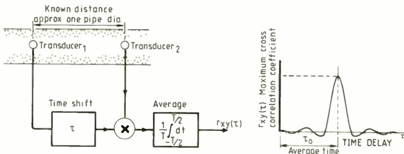
Fig.11. Use of cross-correlation techniques to measure flow-rate. Locating the transducers approximately one pipe diameter apart ensures measurable coefficients without causing prohibitively long signal-processing time (accuracy  $\pm 2\%$ ).
