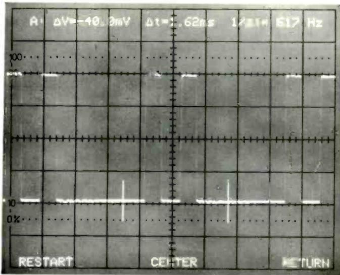
Fig.4. Pressing the 'zoom' (Restart) key automatically calculates the delay and the timebase settings, and....
