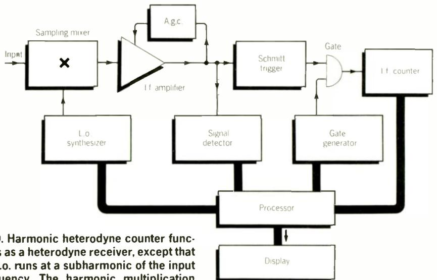
**Fig.9.** Harmonic heterodyne counter functions as a heterodyne receiver, except that the l.o. runs at a subharmonic of the input frequency. The harmonic multiplication factor can be determined by varying the l.o. frequency slightly and measuring the change in the i.f.
