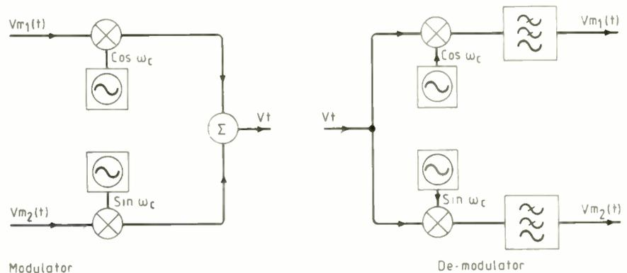
Fig.3. Quadrature-locked oscillators are used to permit product demodulation: this enables two baseband signals to occupy the same carrier space.
