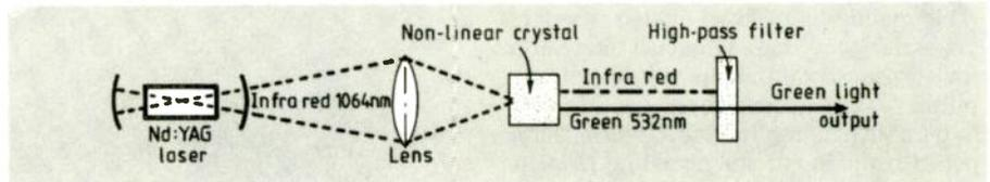
Being distorted in this way, the output wave now contains harmonics which were not present in the input wave and the desired harmonic can be selected by passing the output wave through an optical filter, Fig. 4.
