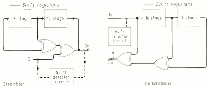
Fig.2. V.22 modems use a form of data scrambling to even out the transmitted energy spectrum.
