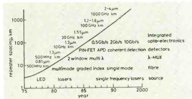
Fig.2 Key milestones for fibre-performance (spacing) projection
