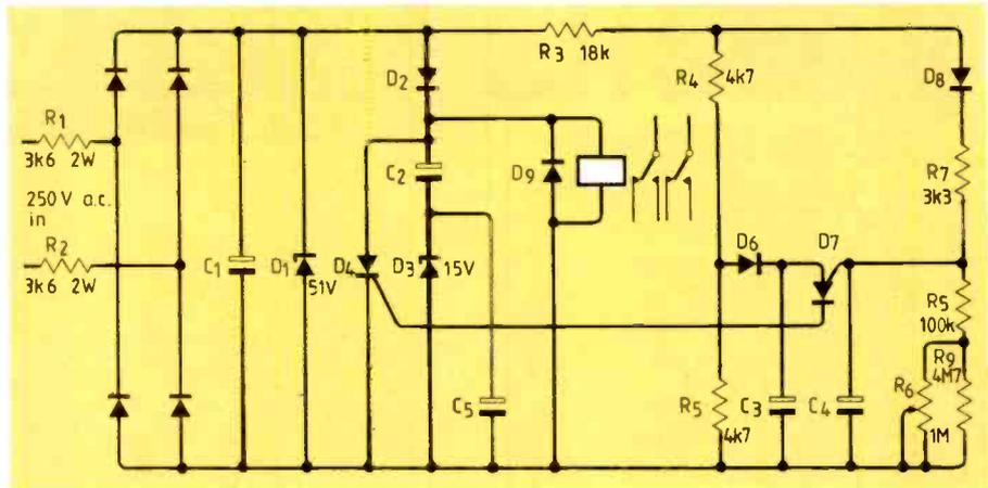
While power is on,  $C_2$  is charged through  $D_2$  and the relay is immediately energized through  $D_3$ . As  $C_3$  charges through  $D_6$  and  $C_4$
