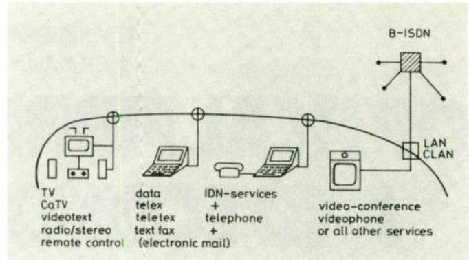
**Fig.4 Broadband communication in integrated or separate networks.**
