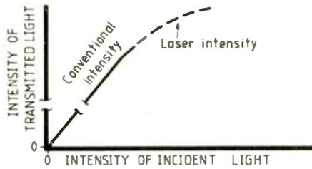
Fig. 3. At low intensity, light output from a given medium is linearly proportional to light entering the medium but when high-intensity laser light is used, transmission becomes non-linear.
