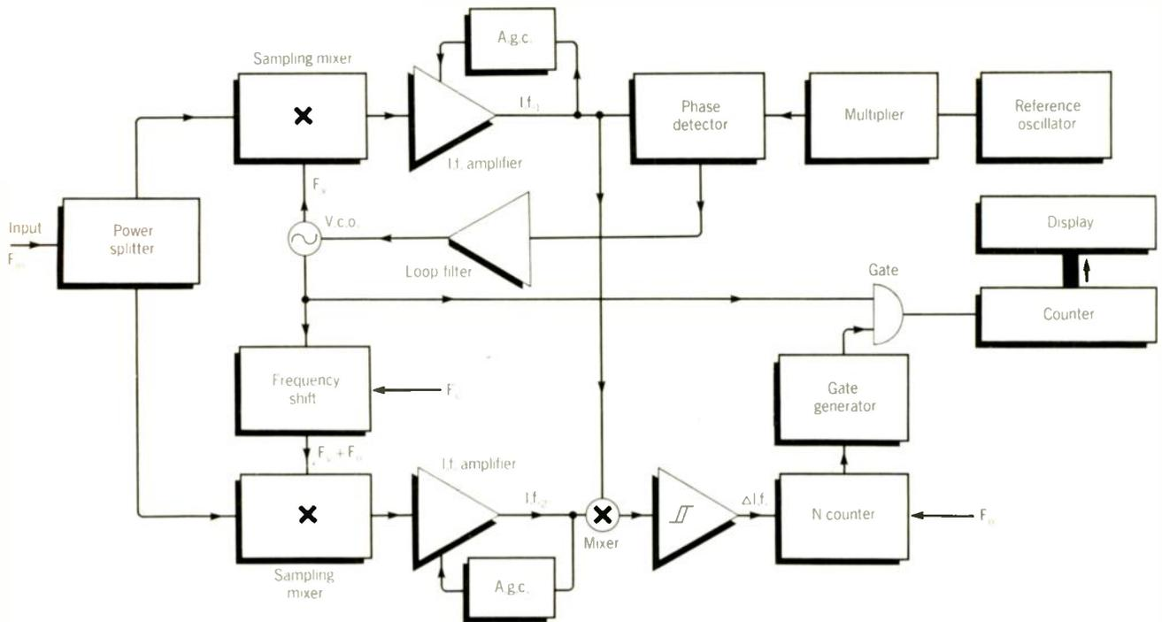
**Fig.8.** In a transfer oscillator, the primary loop is locked onto a subharmonic of the input signal and the harmonic multiplier is determined by the second mixing chain.
