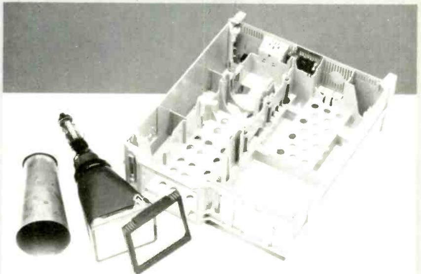
Fig.6. The PM3350's chassis is actually a one-piece injection-moulded frame made from a plastic 'alloy' of polycarbonate and ABS. The frame incorporates all 'click-fit' mountings and stops for p.c.bs and assemblies.
