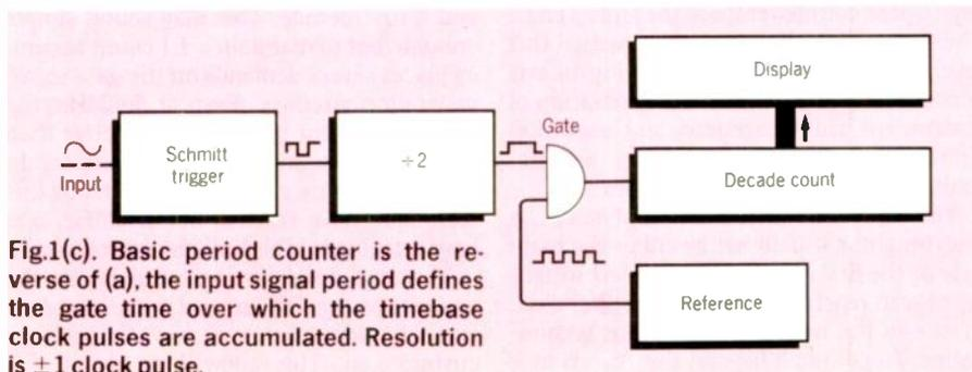
Fig.1(c). Basic period counter is the reverse of (a), the input signal period defines the gate time over which the timebase clock pulses are accumulated. Resolution is  $\pm 1$  clock pulse.
