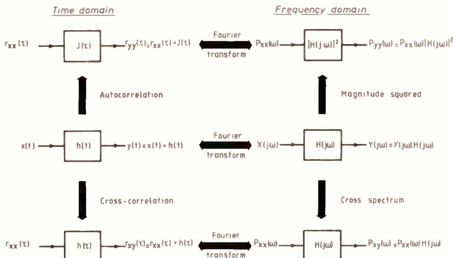
Fig.10. Summary of autocorrelation and cross-correlation signal-processing operations in time and frequency domains. Based on diagrams from Electronic signal processing, T326 Block IV pp.35,37, Open University Press.
