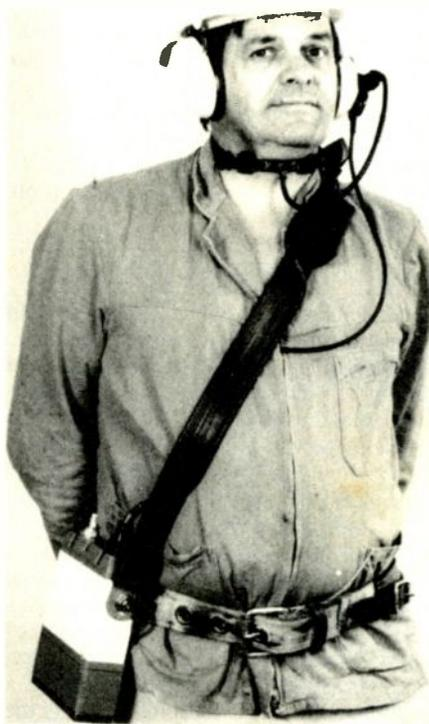
Fig.6. The most recent s.s.b. medium-frequency underground radio equipment, using a throat microphone. The unit contains a noise-blanking system.
