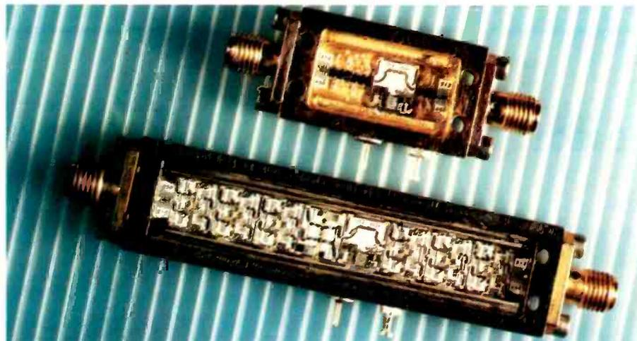
Three cascaded monolithic amplifiers are incorporated in the Thorn EMI 2 to 6GHz microwave amplifier compared with the much larger amplifier it replaces. Apart from the reduction in size, there is a 30:1 reduction in the number of component bonds required, with a saving in both assembly time and cost.
