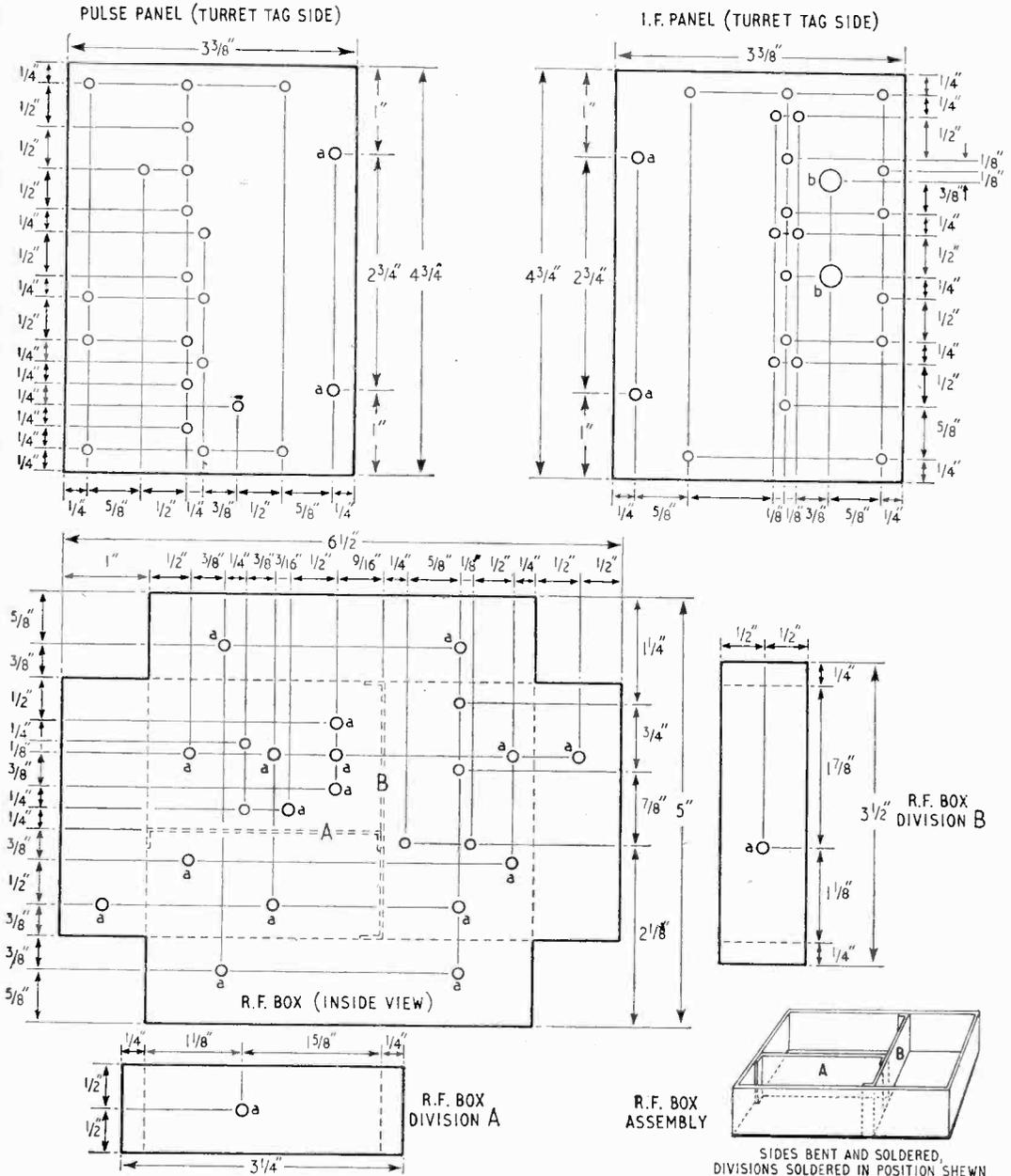
PULSE AND I.F. PANELS MADE FROM  $\frac{1}{16}$ in PAXOLIN
