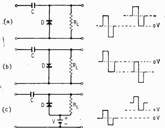
Fig. 64. Diode clammers (unbiased): (a) clamping -ve peak to 0V, (b) clamping +ve peak to 0V, (c) clamping -ve peak to  $+V$ .
