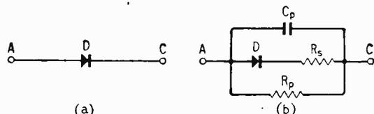
Fig. 62. Ideal and real diodes: (a) ideal diode symbol, (b) real diode equivalent circuit.
