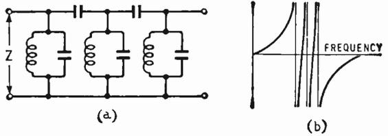
Fig. 7. As additional circuits are coupled, the splitting is repeated.
