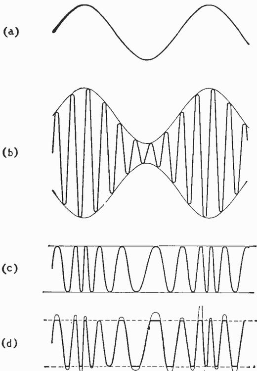
Fig. 1. Amplitude and frequency modulation. Modulating signal at (a) gives a.m. wave as at (b). F.m. signal at (c) is unaffected by random amplitude modulation, as a receiver limiter removes variations.
