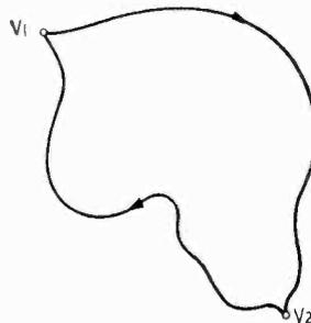
Fig. 2. Derivation of the fact that the net work done in taking any electric charge around any closed path in any electric field is zero.
