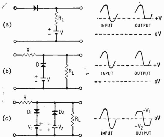
Fig. 63. Diode clippers (or limiters): (a) series, (b) parallel (shunt), (c) double parallel clipper (slicer).
