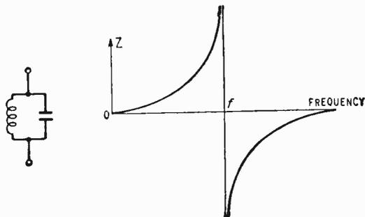
Right:—Fig. 3. Circuit with characteristic frequency  $f$  and its impedance characteristic.
