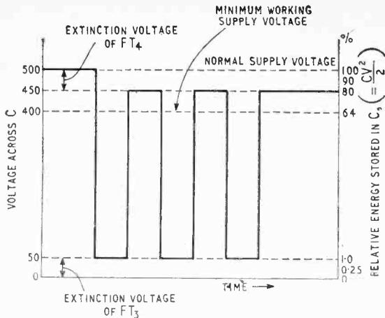
Fig. 2. Voltage and energy changes for the strobe capacitor  $C$ , initially charged to the full supply voltage and used for a sequence of six flashes. The extinction voltage has been exaggerated to 50 V for clarity.
