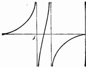
Fig. 6. The impedance diagram for Fig. 5.
