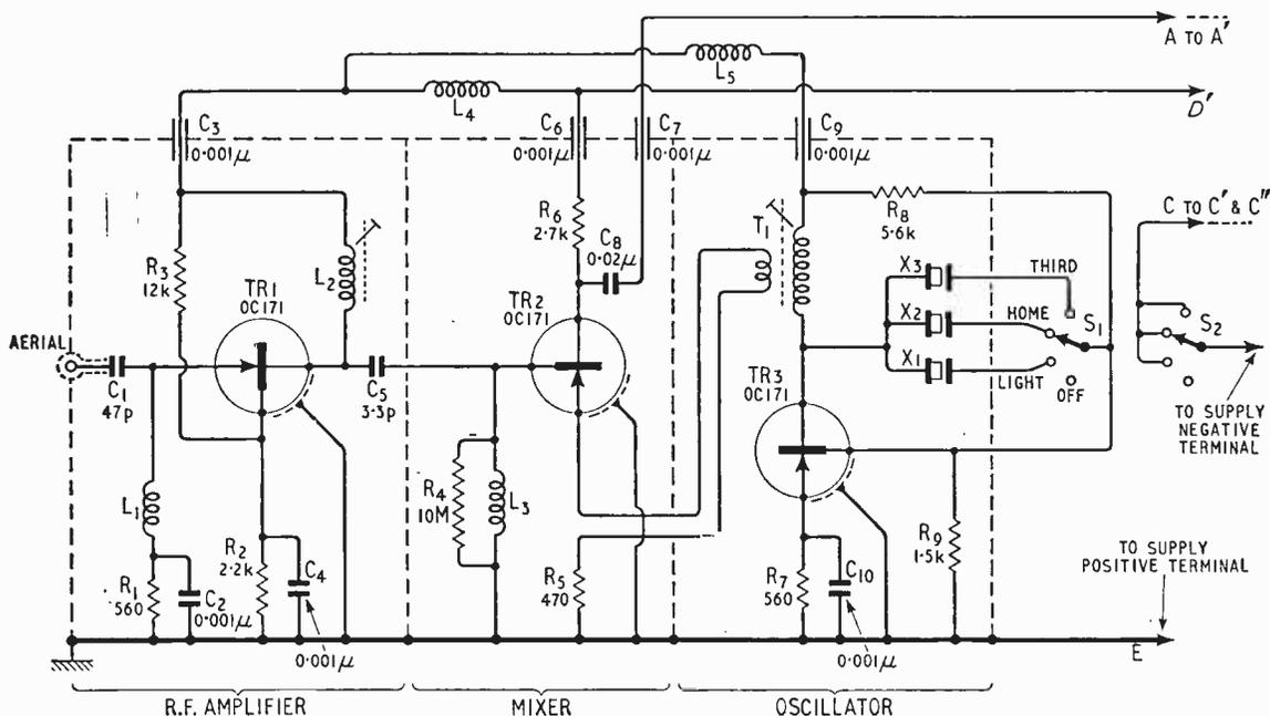
Fig. 6. Circuit diagram of r.f. chassis
