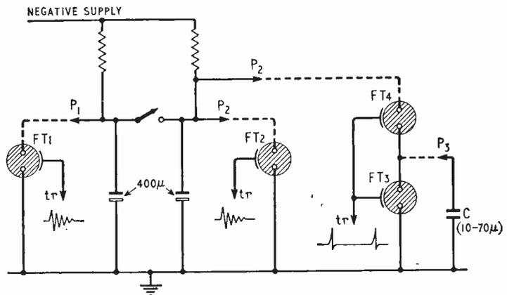
Fig. 1. Basic circuits for single, double or stroboscopic flashes. The points P<sub>1</sub>, P<sub>2</sub> and P<sub>3</sub> refer to the corresponding points in Figs. 4 and 5.
