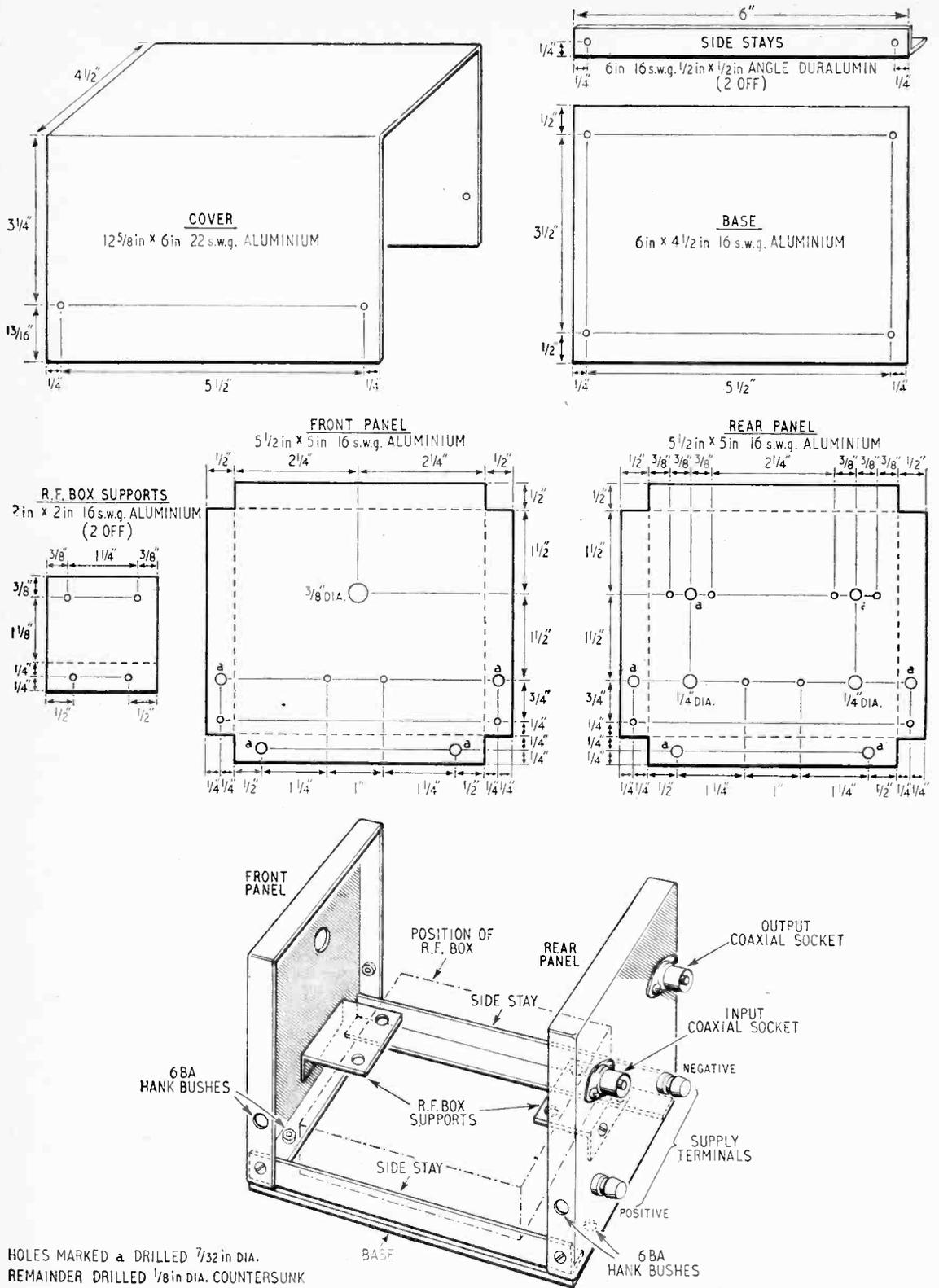
Fig. 11. Construction and assembly of case.
