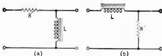
Fig. 61. Linear waveshaping RL filters: (a) high-pass, (b) low-pass.
