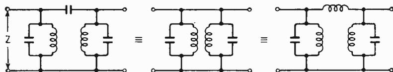
Fig. 4. Coupled circuits, each with characteristic frequencies.
