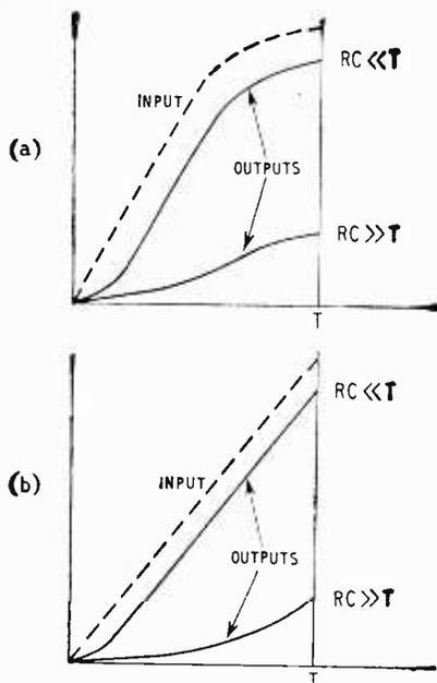
Fig. 60. Low-pass RC filter response to rising ramp: (a) exponential, (b) linear.
