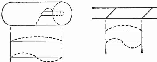
Fig. 1. Coaxial and twin-wire short-circuited resonant structures.
