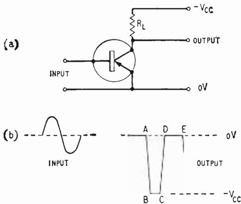
Fig. 65. Overdriven amplifier as amplified clipper.
