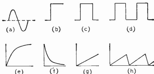
Fig. 56. Waveshapes commonly met with in pulse circuits: (a) sine wave, (b) step, (c) pulse, (d) square wave, (e) exponential, rising, (f) exponential, falling, (g) ramp, (h) sawtooth.
