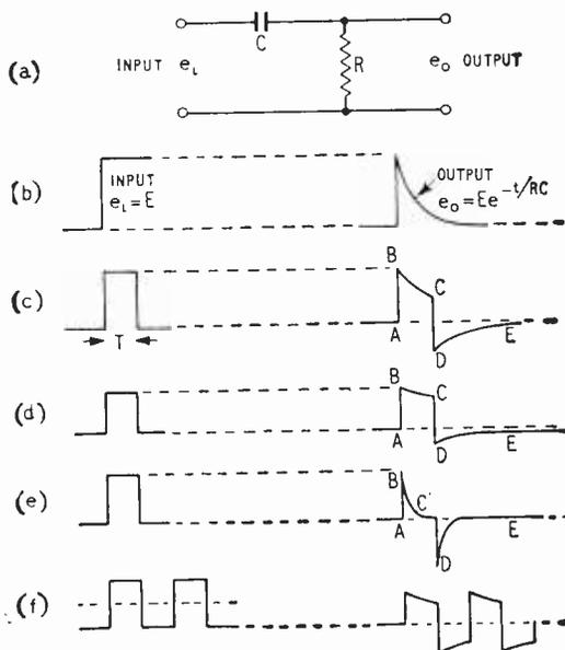
Fig. 57. High-pass RC filter (differentiator): (a) basic circuit, (b) step input, (c) single pulse ( $RC \cong T$ ), (d) single pulse ( $RC \gg T$ ), (e) single pulse ( $RC \ll T$ ), (f) pulse train.
