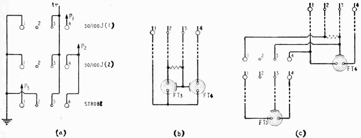
Fig. 5. Diagrams of the output and flash-head wiring. (a) The three UX4 output sockets. (b) A strobe-head consisting of two FA27 tubes on a single base. (c) Two separate heads, one of which bears an accessory UX4 socket for strobe use.
