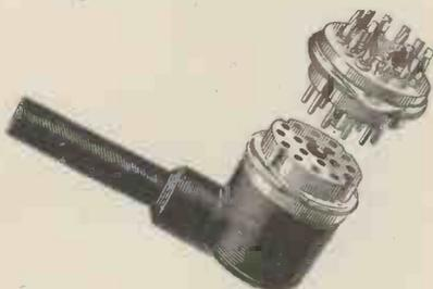
\* No cover and cable clamp worries. We connect your cable to plug or socket and put the assembly in polythene. \* 18 connections in less than 1 inch diameter. \* Standard B9A valveholder mounting. \* Nylon loaded PF. mouldings. \* Cadmium plated or gold pins and contacts.
