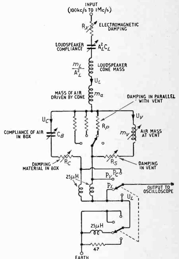
Fig. 3. Analogue network referred to acoustic output for obtaining the performance of a loudspeaker in a bass reflex cabinet.
