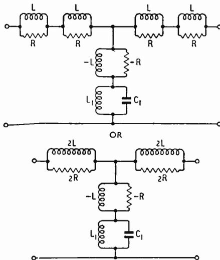
An interesting phenomenon is that this simple T circuit is quite symmetrical whilst the original bifilar -T is apparently not so. This is readily accounted for if we recall that the centre-tapped coil 4L is a 1:-1 transformer with perfect coupling, and so any impedances in its primary are reflected perfectly into its secondary circuit.
