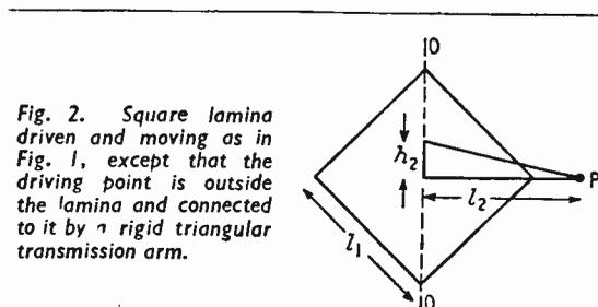
Fig. 2. Square lamina driven and moving as in Fig. 1, except that the driving point is outside the lamina and connected to it by a rigid triangular transmission arm.
