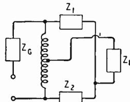
In this shape the two impedances  $Z_1$  and  $Z_2$  of the first network have changed places with the generator and load impedances respectively. This circuit has also been used as a filter, especially by Jaumann.
