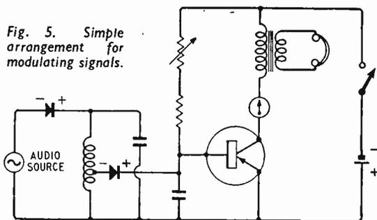
volume. The modulator has been found to be invaluable, however, for quick searching for signals of moderate strength. These are very easily heard, but produce only a small meter deflection, which can easily pass unnoticed if the tuning knob is turned quickly. The presence of an audio note at the appropriate part of the band enables the correct area to be searched slowly, so that the deflection is observed.
