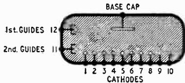
Fig. 1. Symbolic diagram of a typical Dekatron.
