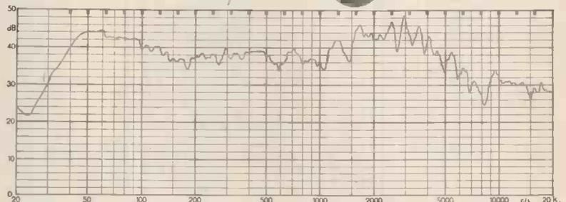
Axial frequency response of Coaxial 12 unit.
