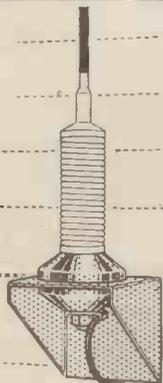
An 18 ft. aerial using copper coated high tensile steel 3 ft. sections, screwed and spigoted for additional strength. It is mounted on a base insulator incorporating a robust double helical spring. Designed primarily for heavy duty mobile applications, for either military or civil use over the roughest country. As a portable aerial, extra sections can be added with suitable guys.
