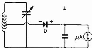
Fig. 1. Simple absorption wavemeter with diode detector.
