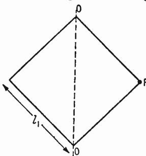
Fig. 1. Square lamina driven at one corner (P) in a direction at right angles to its plane so as to rotate about the diagonal O-Q.
