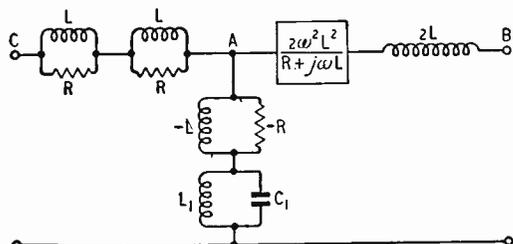
We now add the two impedances in the arm AB and get  $(2j\omega L R)/(R + j\omega L)$ , which is the same as the imped-
