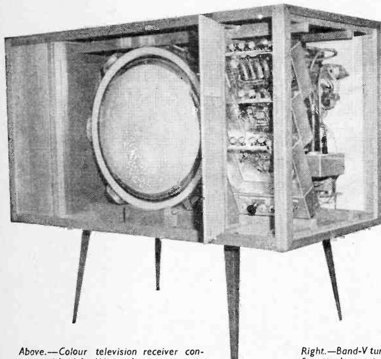
Above.—Colour television receiver constructed by John Ware, showing arrangement of chassis.
