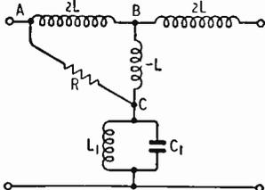
The points A, B and C now form the vertices of a delta, which can be converted to a star whose arms from A, B and C to the centre of the star have the following impedances respectively:
