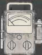
**A.C./D.C. Valve Voltmeter**—Six A.C. ranges from 1–300 Volts f.s.d. up to 200 Mc/s and seven D.C. ranges from 1–1,000 Volts f.s.d. at high impedance.
