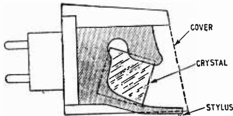
Fig. 9 Sketch of final form of pickup.
