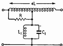
The centre-tapped coil treated as a three-terminal net can be reduced to the following star arrangement (providing perfect coupling is assumed between the two halves of the coil):
