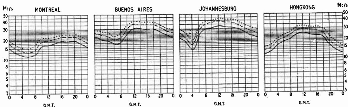
THE full-line curves indicate the highest frequencies likely to be usable at any time of the day or night for reliable communications over four long-distance paths from this country during April.
