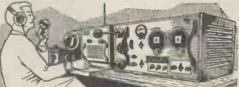
Complete station comprising Transmitter/Receiver 2-8 Mc/s. 12 v. supply unit, Aerial, Variometer, control box, headphones, microphone and all leads, circuit and instruction book. S.A.E. for full details **£9** Carr. 20/6.
