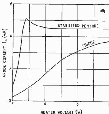
performance, the curves of anode current against heater voltage compare the stabilized triode-connected 6K7 pentode with an unstabilized and normally connected 6J5 triode.
