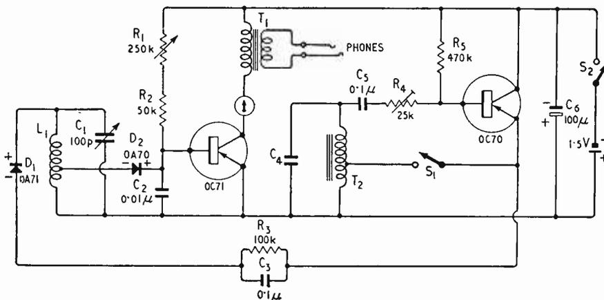
achieved until the collector current is raised to about 3mA, but the reduction is not serious down to 0.5mA, or even 0.25mA. Unless one is prepared to incorporate a backing-off arrangement for standing current, there is therefore little point in using a meter with a f.s.d. much below 0.5mA. If a really sensitive meter is available (say, 100 $\mu$ A) then the circuit of Fig. 2 will probably be adequate. If the standing
