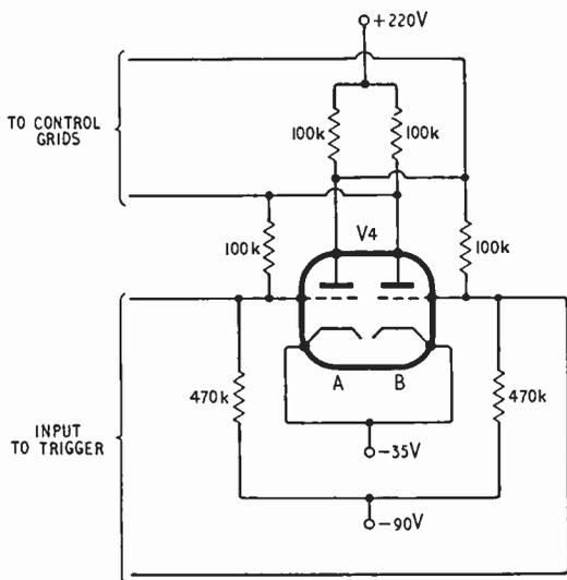
Fig. 3. Bi-stable circuit used in the reversible counter.
