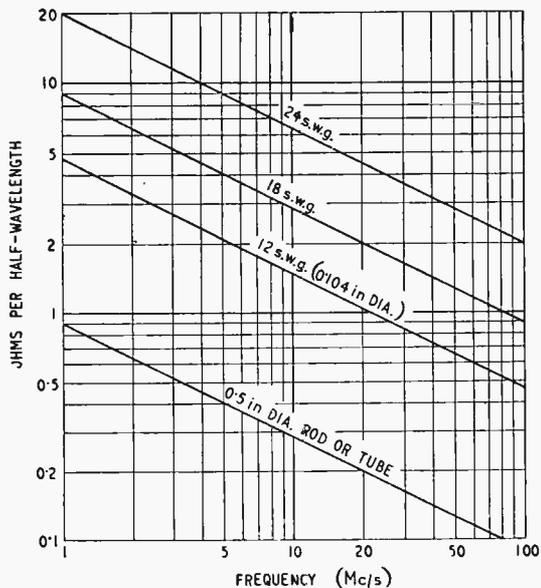
Fig. 5. R.F. resistance of copper conductors. Resistance per unit length is proportional to  $\sqrt{\text{frequency}/(\text{perimeter of conductor})}$ , provided thickness of conductor is large compared with skin depth which is approximately  $0.007/\sqrt{\text{Mc/s}}$  (in cms). For non-magnetic material's r.f. resistance is approximately proportional to  $\sqrt{\text{specific resistance}}$ .
