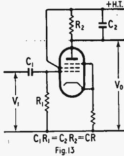
Fig. 13 Pentode isolated circuit.
