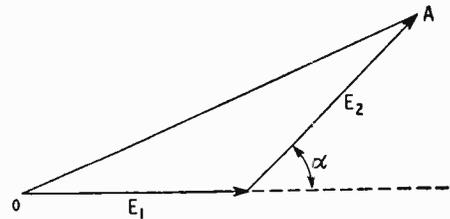
Fig. 10. Vector addition of two fields.  $E_1$  represents field at  $P$  due to element  $A'B'$  of Fig. 3.  $E_2$  represents (same scale) field due to  $A'B'$ . Angle  $\alpha$  is the relative phase of the two fields and is equal to  $360^\circ \times d/\lambda \cos \theta$ . The field strength at  $P$  is proportional to length  $OA$ . Similar procedure is applicable to any number of field components when relative magnitudes and phases are known.
