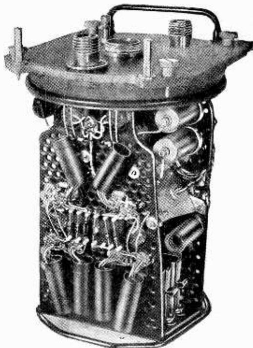
*Early honeycomb-type chassis. High-dissipation valves (wire connections only are visible) are mounted in the integral type of screen shown, detached from chassis, in other photograph. Coolant-hose connections are made to the two large screwed unions on panel. Whole chassis, without components, weighs only 1½ lb.*
