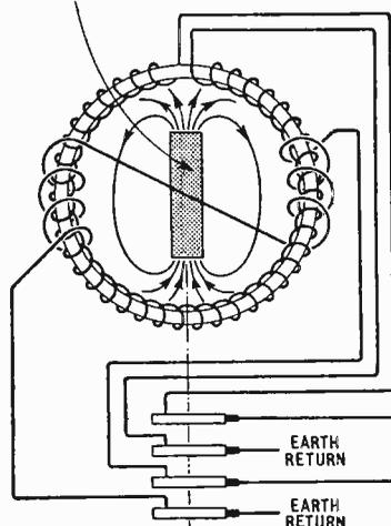
Simplified schematic diagram of transmitting magnetic compass.
