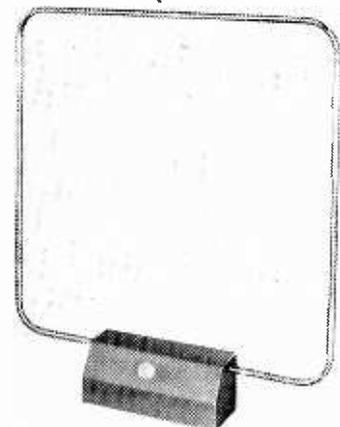
Consisting of a single turn of self-supporting light-alloy tube about 2½ft square, it is tuned approximately by switching in fixed capacitors for reception of three stations, two in the medium waveband and one in the long. Each is broadly tuned.
