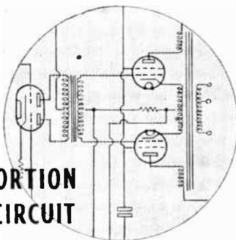
The new low distortion output circuit (an Acoustical Provisional Patent) incorporated in the M31 Amplifier provides a very high standard of reproduction—The output valves operate partly as triodes with cathode follower output and partly as tetrodes with negative feedback, thus giving considerable cancellation of generated harmonics and a high damping factor. Just one reason why you prefer Acoustical.
