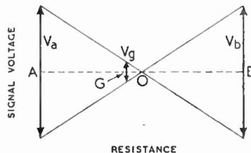
Fig. 2. Diagram showing signal voltage amplitude, as the vertical distance between the sloping lines, at all points between A and B along  $R_5$  and  $R_6$ . As  $V_a$  and  $V_b$  are assumed equal, O, the point of zero voltage, is at the centre point, with equal resistance each side. The required grid voltage is obtained at G, so AG represents the resistance of  $R_5$  and GB that of  $R_6$ . (For clarity,  $V_g$  is exaggerated, here and in Fig. 3.)
