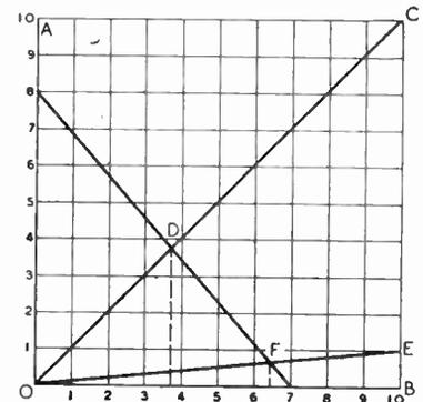
OE at F. Dropping vertically from F to OB we find that the reading is a little under 650 ohms—say 645. Work it out and you will find that the graphical solution is not so very far wrong.
