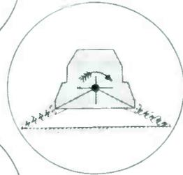
which, translated in a modern practical manner, utilizes "FLEXILANT" rubber-bonded-to-metal mountings, scientifically designed to give absorption of vibration.
