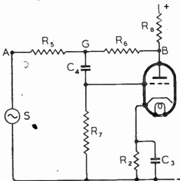
Fig. 1. The see-saw circuit in its simplest form.
