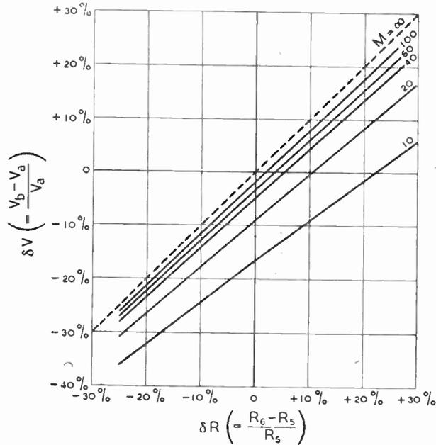
Fig. 5. Diagram showing the percentage departure from voltage balance ( $\delta V$ ) in terms of the percentage difference between  $R_6$  and  $R_5$  ( $\delta R$ ), for several values of amplification,  $M$ .
