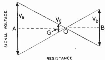
Fig. 3. Here  $R_5$  and  $R_6$  are assumed equal, so G is the centre point, and O is displaced.  $V_b$  is therefore less than  $V_a$ ; but the difference is small if  $V_g$  is very small compared with  $V_b$ .
