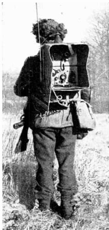
SUCCESSOR of the well-known infantry set No. 18. This short-range transmitter-receiver, the 68P, operates in the 1.75 to 2.9 Mc/s band with crystal control for sending. It has facilities for 'phone and CW operation.
