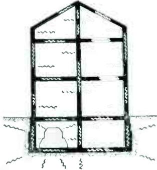
. . . the IDEAL way to prevent this transmission is to suspend the machine with springs converging on the centre of gravity thus . . . . .
