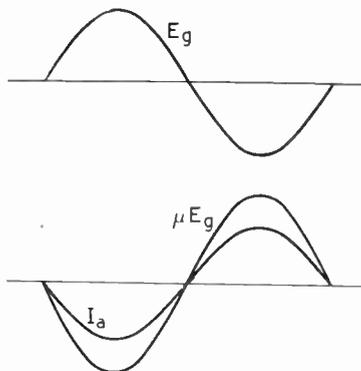
Fig. 1. Grid-voltage anode-current relationship.
