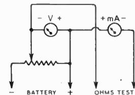
Method of using a voltmeter and milliammeter for resistance measurements.
