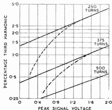
Fig. 2. Third harmonic distortion at various input levels produced by iron-cored coils bridged across 500-ohm line. Frequency of fundamental 50 c/s.
