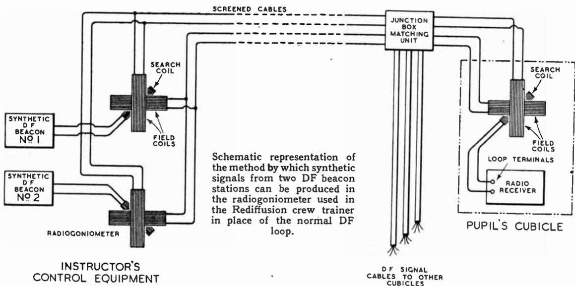
Several modifications have had to be made to the standard radio equipment in order to reproduce artificially the actual conditions obtaining in the air. Normally DF bearings are taken with a rotatable loop aerial, but as space-wave radio signals are not used in this trainer the loop is replaced by a radiogonio-
