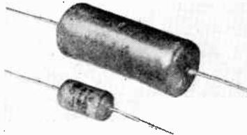
Hunt's metallised paper capacitors; showing one of  $0.1\ \mu\text{F}$  and one of  $0.5\ \mu\text{F}$  capacity. As the larger is comparable in dimensions to a standard pattern paper tubular of  $0.1\ \mu\text{F}$  it serves as a basis for comparing the size of the smaller 150-volt type. The larger is for 350 volts DC working.
