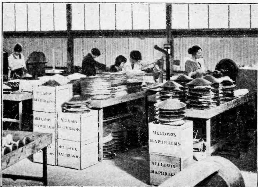
**LOUD-SPEAKERS IN THE MAKING.** An interesting corner of the Sterling Works, Dagenham, showing the processes of shaping and assembling Mellovox loud-speaker diaphragms.
