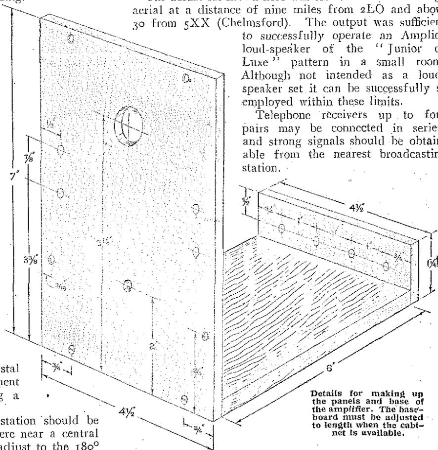
Details for making up the panels and base of the amplifier. The base-board must be adjusted to length when the cabinet is available.
