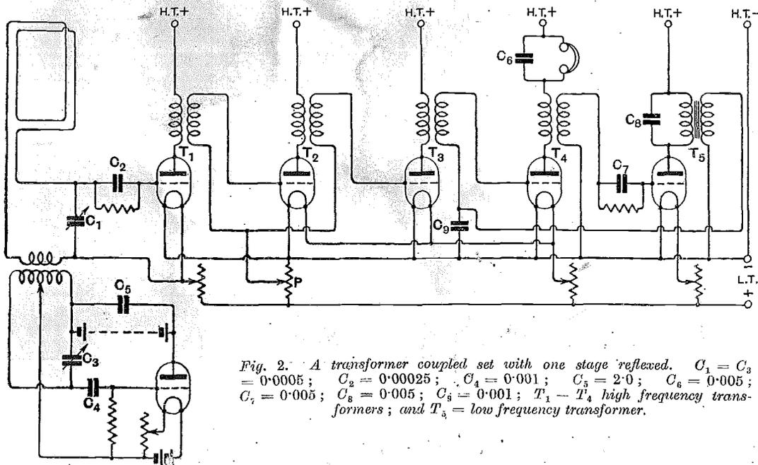
Fig. 2. A transformer coupled set with one stage reflexed.  $C_1 = C_3 = 0.0005$ ;  $C_2 = 0.00025$ ;  $C_4 = 0.001$ ;  $C_5 = 2.0$ ;  $C_6 = 0.005$ ;  $C_7 = 0.005$ ;  $C_8 = 0.005$ ;  $C_9 = 0.001$ ;  $T_1 - T_4$  high frequency transformers; and  $T_5 =$  low frequency transformer.
