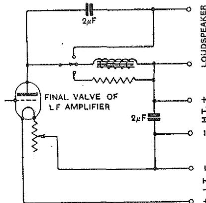
An experimental filter circuit.
