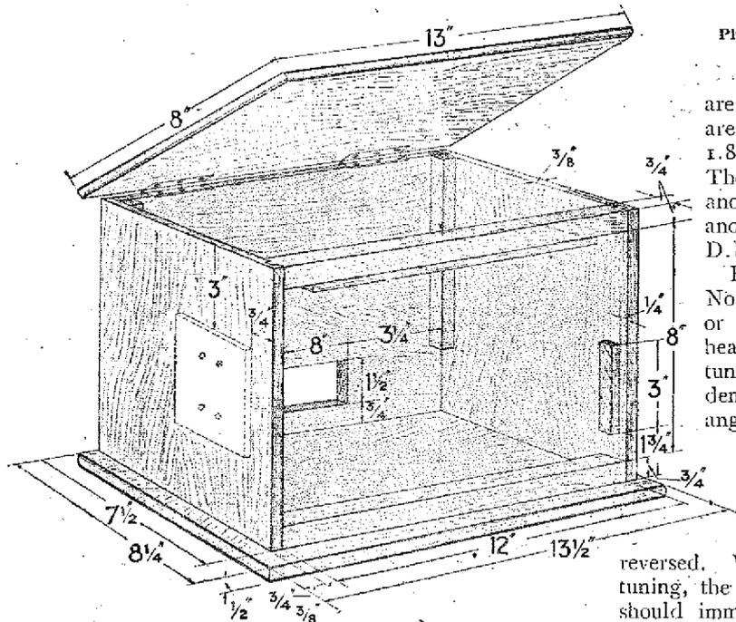
Fig. 5.—Sketch of cabinet, showing dimensions, position of slot in back for the terminal strip, and position of two-coil holder.
