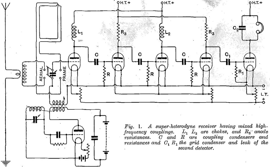
Fig. 1. A super-heterodyne receiver having mixed high-frequency couplings.  $L_1$   $L_2$  are chokes, and  $R_3$  anode resistances.  $C$  and  $R$  are coupling condensers and resistances and  $C_1$   $R_1$  the grid condenser and leak of the second detector.
