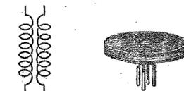
A high-frequency transformer with a fixed coupling. May be of the pin type shown, or consist of two coils fixed together, or a coil with a double winding.
