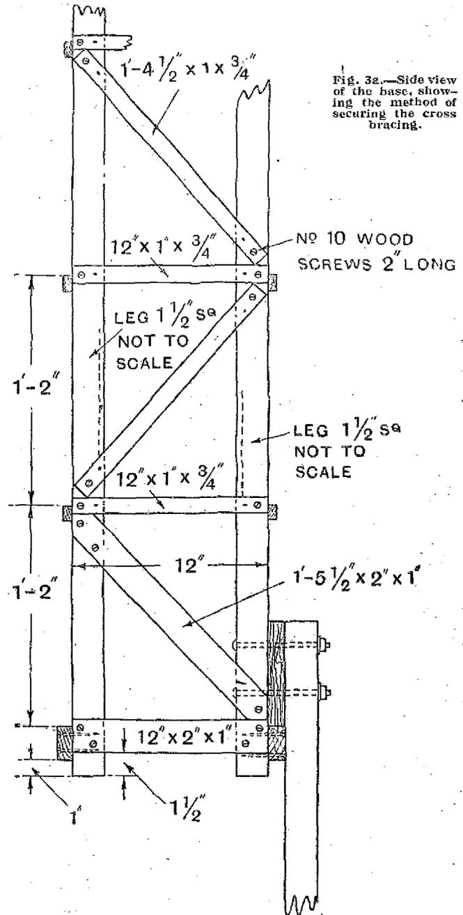
Fig. 3a.—Side view of the base, showing the method of securing the cross bracing.
