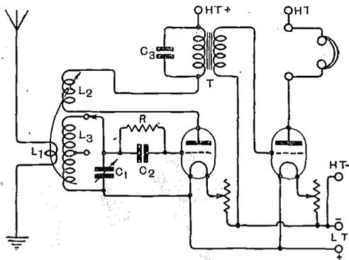
Fig. 1. Connections of the receiver.  $L_1$  is the loosely coupled aerial coil;  $L_2$ , the reaction coil;  $L_3$ , the tapped secondary coil;  $C_1$ , the tuning condenser;  $RC_2$  the grid leak and condenser;  $C_3$ , the by-pass condenser, and  $T$  the intervalve transformer.
