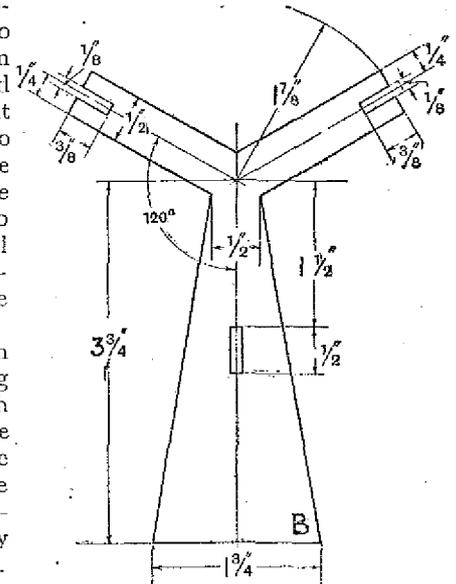
Fig. 3.—Details of the pieces marked B in fig. 2. These are of hardwood, 1/8th in. thick.
