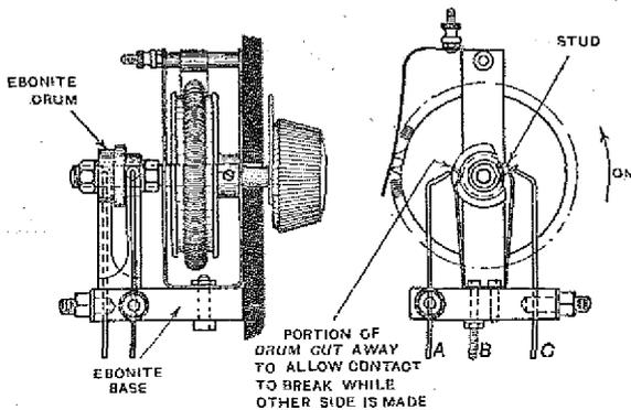
A switch is fitted to the filament rheostat so as to disconnect an amplifying stage when the knob is turned to the "off" position.
