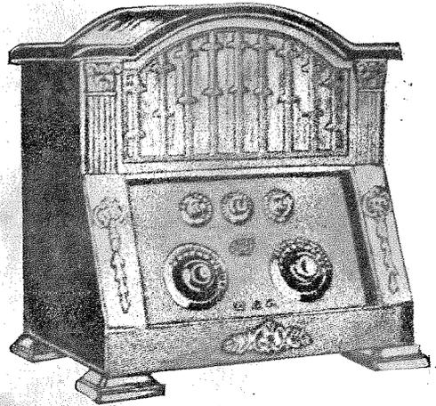
*The Bestone 5-valve receiver with built-in loud speaker and battery compartment.*
