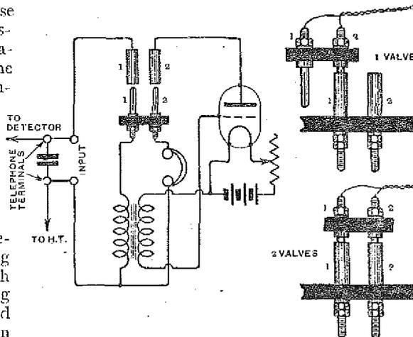
An L.F. valve switch constructed from valve pins.
