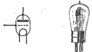
A three-electrode valve; that is, a receiving or transmitting valve having a filament, grid and anode.
