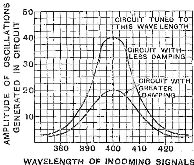
Fig. 3.—Resonance curves of two circuits, one having greater damping than the other.
