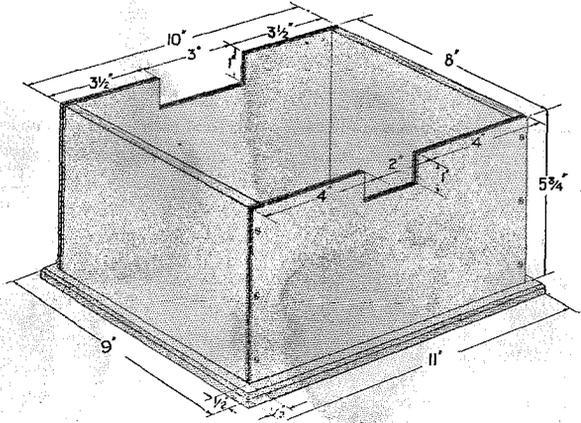
Fig. 7. A sketch of the box of the instrument, which is of simple construction.
