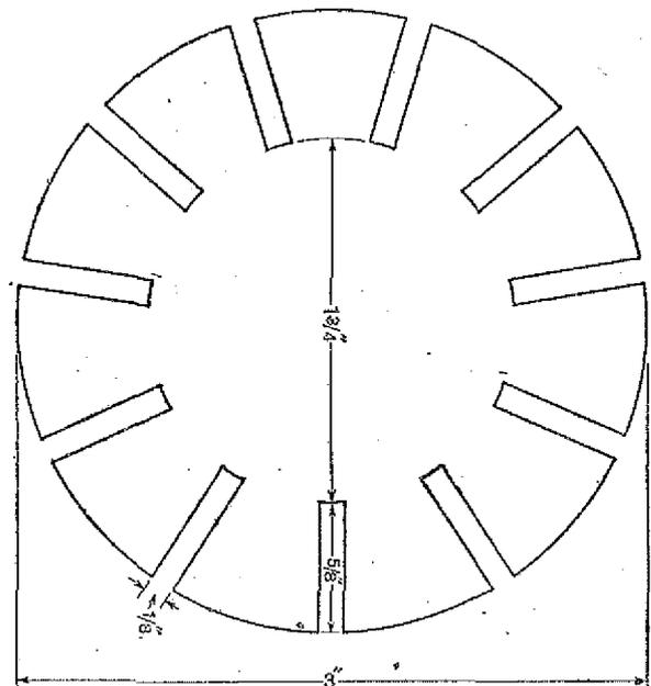
Fig. 2.—Dimensions of the former for a basket coil.
