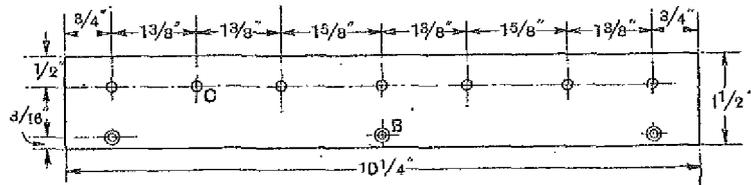
Fig. 11.—Details of the terminal strip.
