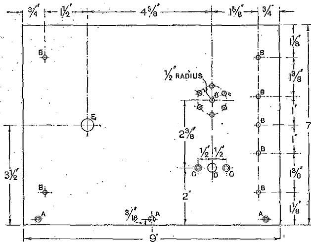
Fig. 2.—Drawing of the ebonite panel, showing the position and size of the holes. A =  $\frac{1}{8}$ " dia. and countersunk for No. 4 wood screws; B =  $\frac{3}{16}$ " dia.; C =  $\frac{3}{16}$ " dia., and countersunk for No. 4 E.A. screws; D =  $\frac{3}{16}$ " dia.; E =  $\frac{3}{16}$ " dia.
