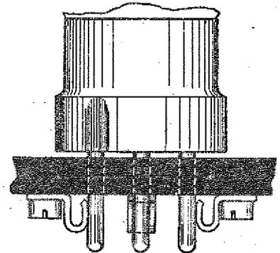
Design for a valve holder with contacts beneath the panel, and presenting very little stray capacity.
