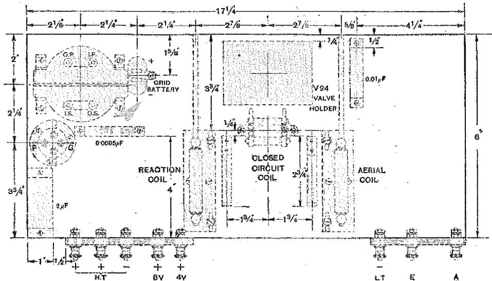
Fig. 2.—Details of the base, showing the position of the components.
