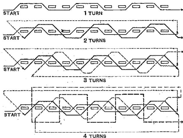
Fig. 2.—Method of winding the basket coil.
