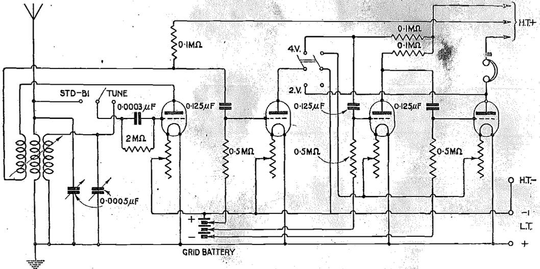
*A four-valve receiver having a valve detector and three stages of resistance-coupled low-frequency amplification.*
