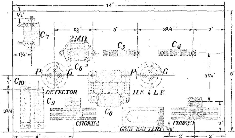
Fig. 4.—Arrangement of parts on the base.
