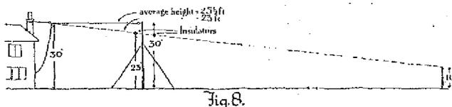
wire is recommended. Such a wire is flexible, inconspicuous and of ample strength. As regards insulation, very small porcelain insulators are the best. So long as they offer a clear inch of surface between the aerial wire and any support, the insulation is ample. Larger insulators are unnecessarily clumsy. A single insulator should be used at each point of support.
