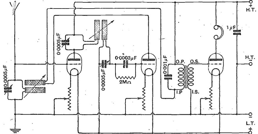
A receiver with one stage of loose coupled tuned transformer H.F. amplification, valve detector and note magnifier.
