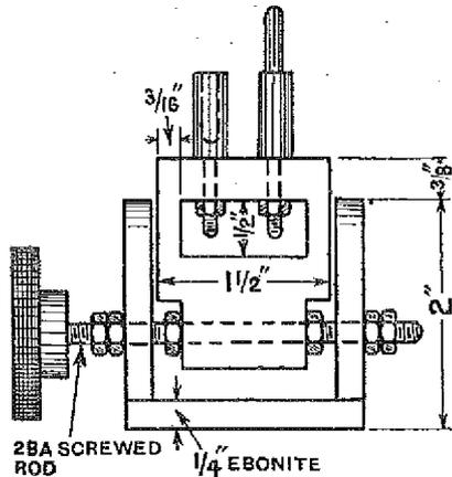
An easily constructed two-coil holder.
