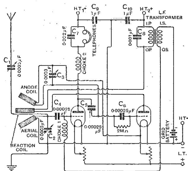
Fig. 2.—Theoretical diagram of connections.
