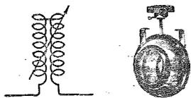
A variometer. The windings may be connected in series or parallel.
