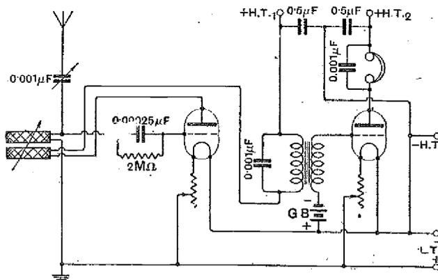
Fig. 1.—The theoretical connections of the set
