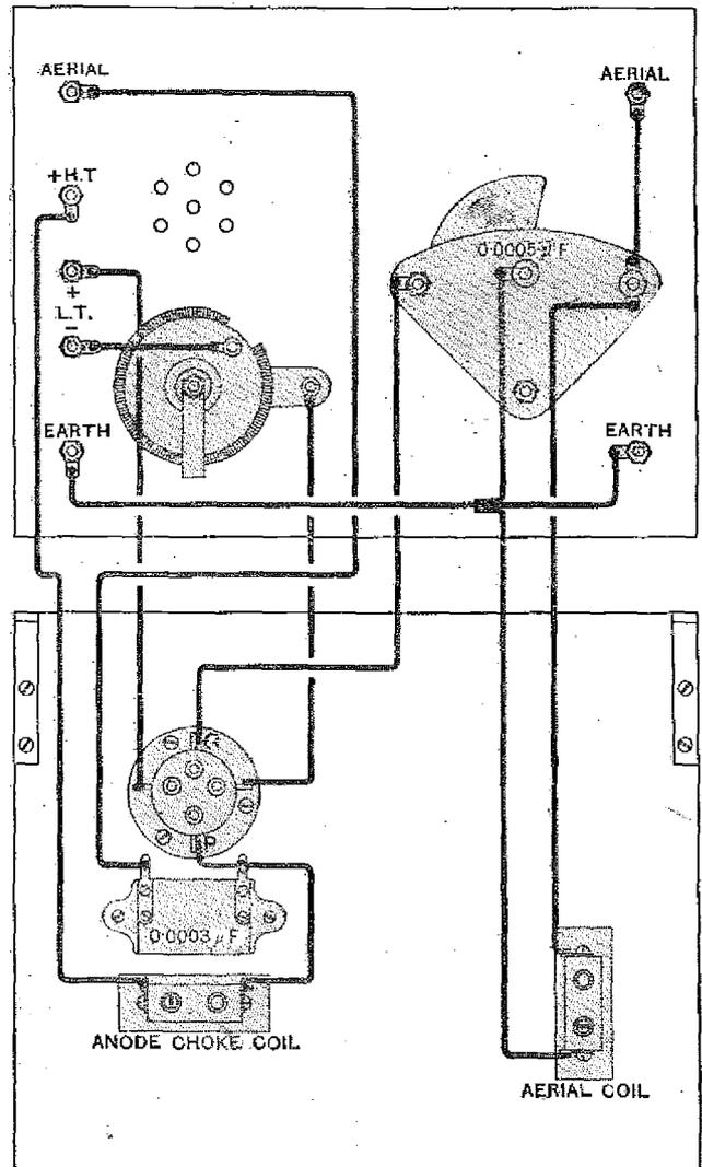
Fig. 4.—The wiring connections of the unit.
