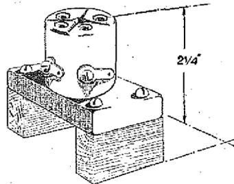
Microphonic valve noises are avoided by supporting the valve holder on an indiarubber platform.
