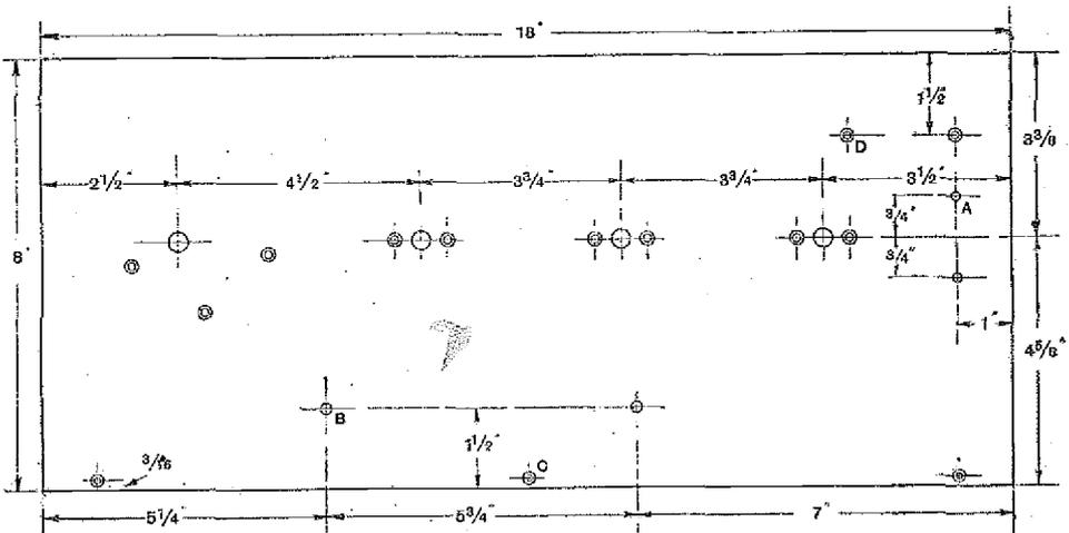
Fig. 1.—Details of the ebonite front panel. A = drill 5/16 in. B = drill 1/2 in. C = drill 1/4 in. and countersink. D = drill 3/8 in. for 4 B.A. countersunk screws.
