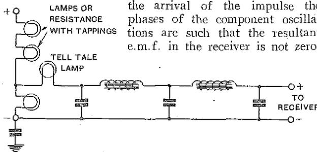
Fig. 5.—When the direct current mains are used as a source of H.T. for a receiver, the circuit shown here may be used. A high-resistance potentiometer may be used instead of the lamps.
