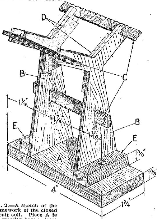
Fig. 2.—A sketch of the framework of the closed circuit coil. Piece A is the wooden base; pieces B are drawn in detail in fig. 3; pieces C are given in detail in fig. 5; pieces D are to strengthen the former, and pieces E are blocks of wood to which are screwed the upright pieces.
