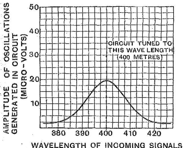
Fig. 2.—A resonance curve.
