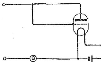
Fig. 1.—A valve rectifier and galvanometer.
