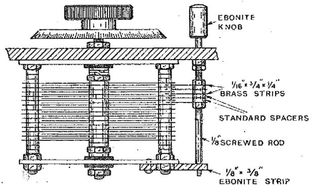
Fitting a vernier control to a variable condenser by means of a spindle carrying a few semi-circular plates, and engaging into the projections of the fixed plates.
