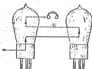
Fig. 1.—The reflex principle.
