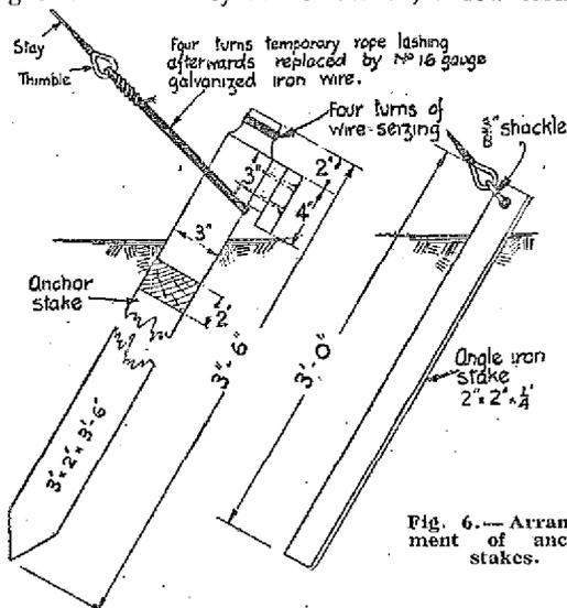
Fig. 6.—Arrangement of anchor stakes.
