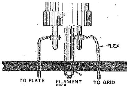
A good method of avoiding capacity and poor insulation troubles.
