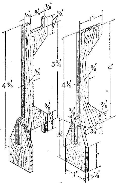
Fig. 6.—On the left is shown the wooden framework for supporting the reaction coil and on the right, the framework for the aerial coil. These pieces are secured to the movable portion of the coil-holders.
