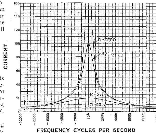
Fig. 1.—The value of the current flowing in the circuit over a range of frequencies when the circuit has resistances of 20, 5, 1, and zero ohms.
