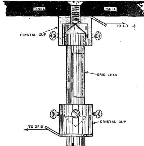
*Using crystal cups for making contact with a grid leak.*
