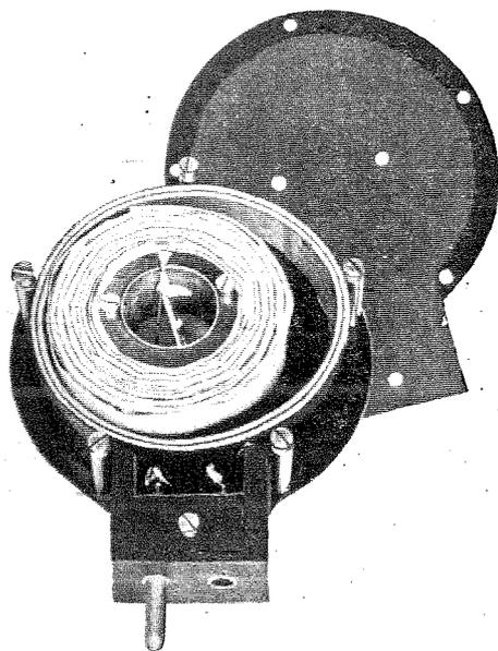
Interior of the "Cosmos" coil. The turns are paper supported, producing a very low dielectric loss.
