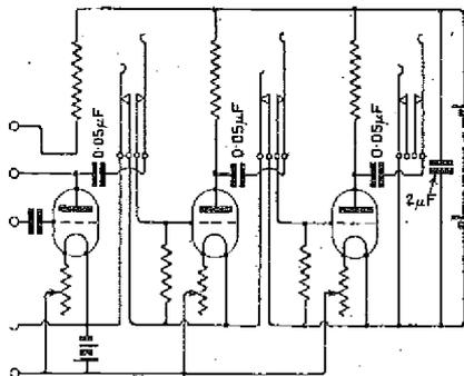
A useful method of switching a resistance coupled low frequency amplifier.
