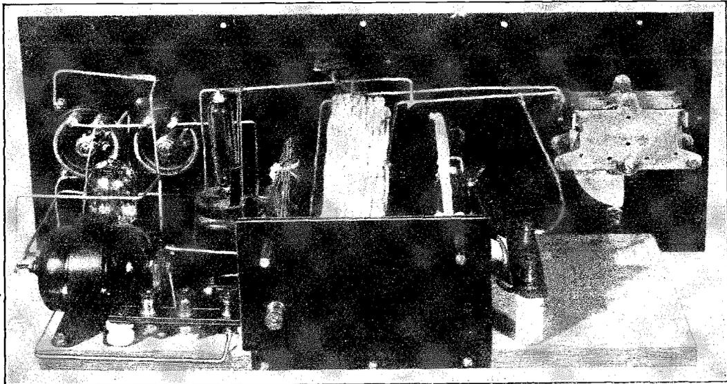
A view showing the arrangement of the set. Looking from right to left we have the tuning condenser, aerial coil, closed circuit coil and reaction coil. Then the detector valve and the transformer and valve for the I.F. stage.
