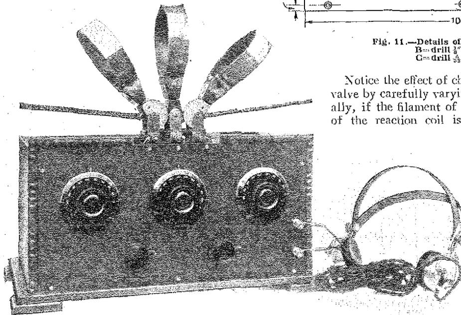
View of the complete Two Valve Reflex Receiver. In the coil holder, from left to right, are the aerial, reaction and anode coils. The first tuning condenser is in series with the aerial, the second across the aerial coil and the third across the anode coil.
