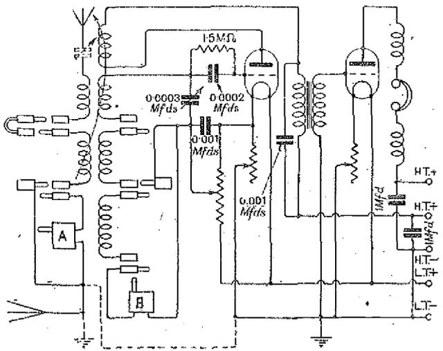
Fig. 1.—The circuit is a detector valve with reaction followed by a note magnifier. The short wave tuning inductances are shown while loading coils may be added at A and B or inserted into the plug and socket connectors in place of the "U" links.
