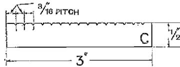
Fig. 5.—Details of the pieces marked C in fig. 2. These are of hardwood 1/8 in. thick, but may be of ebonite.
