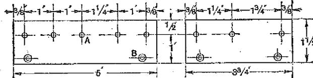
Fig. 3.—The ebonite terminal strips. A = drill  $\frac{1}{2}$  in. B = drill  $\frac{3}{8}$  in. and countersink.
