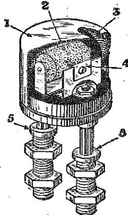
The internal construction of the Harlie detector
