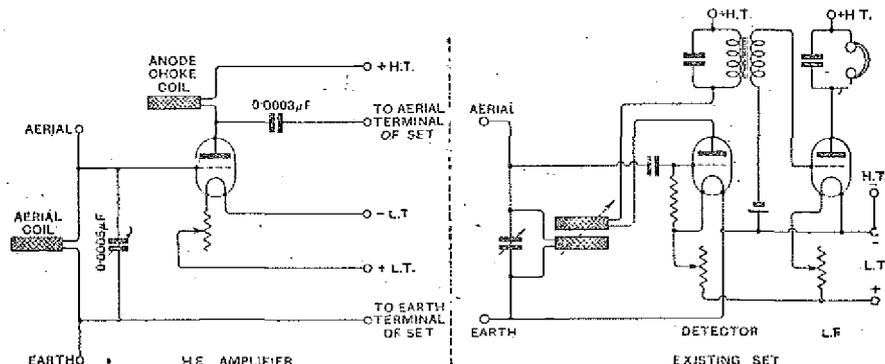
Fig. 1.—The connections of the H.F. unit, and those of a typical set having a detector and note magnifier. To connect the H.F. unit to the set connect the terminals marked "To aerial terminal of set" and "aerial"; "To earth terminal of set" and "earth"; H.T.+, to the H.T. battery, and connect the L.T. terminals to the filament battery. The aerial and earth should be joined to the respective terminals of the H.F. unit.
