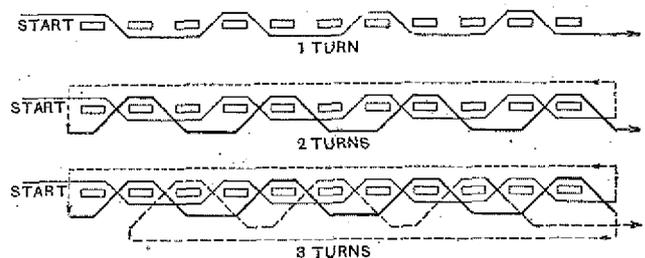
Fig. 3.—Method of winding a basket coil having a mixed pitch of two and four.
