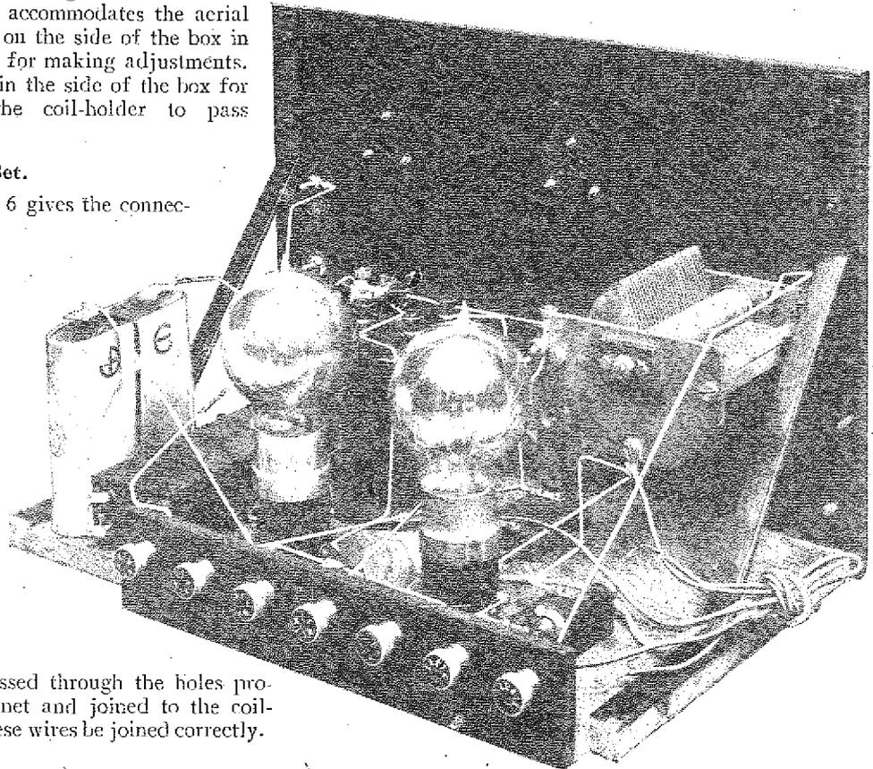
Photograph of the back of the set. The four flexible wires on the right connect to the coil-holder.
