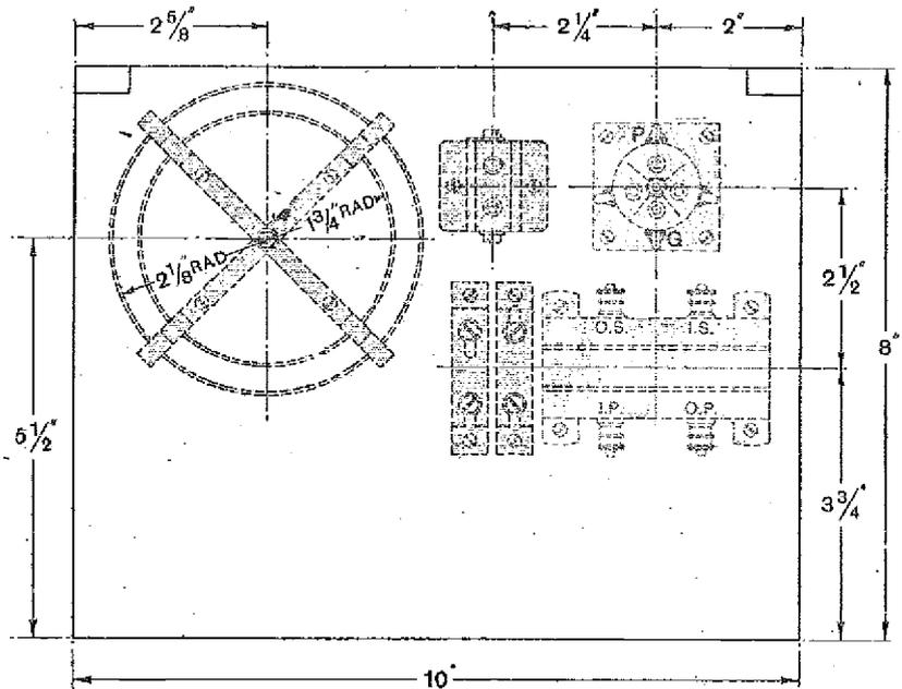
Fig. 4.—The layout of the components on the base board.
