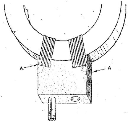
A good way of securing a home-made tuning coil to a plug and socket mount.
