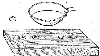
Casting up small pieces of crystal into pellets of Woods metal.
