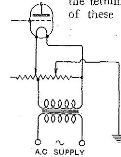
Fig. 6.—A method of reducing hum when the filaments are heated with alternating current.
