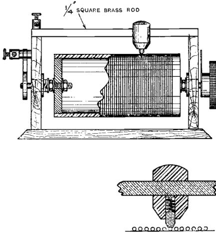
be required when using an inductance of large value, but for tuning the short wavelengths when the turns may be spaced, it will be found very helpful to set up the coil so that it can be rotated, causing the sliding contact to connect upon the turns of the wire and advance as the former revolves.
