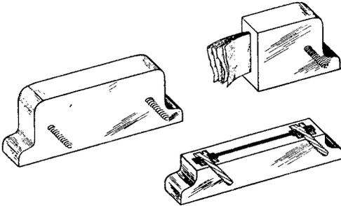
*The completed condenser and a sectional view showing the appearance of the clamped plates.*
