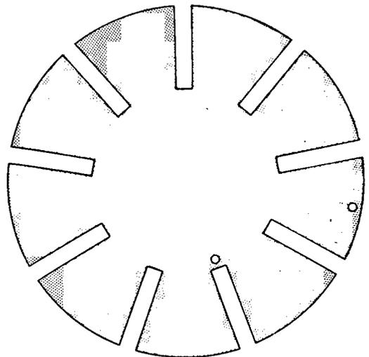
Fig. 5. Card for winding the inductances (exact size).
