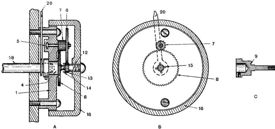
Fig. 1. The construction of a tuning device which provides a quick and a slow movement.
