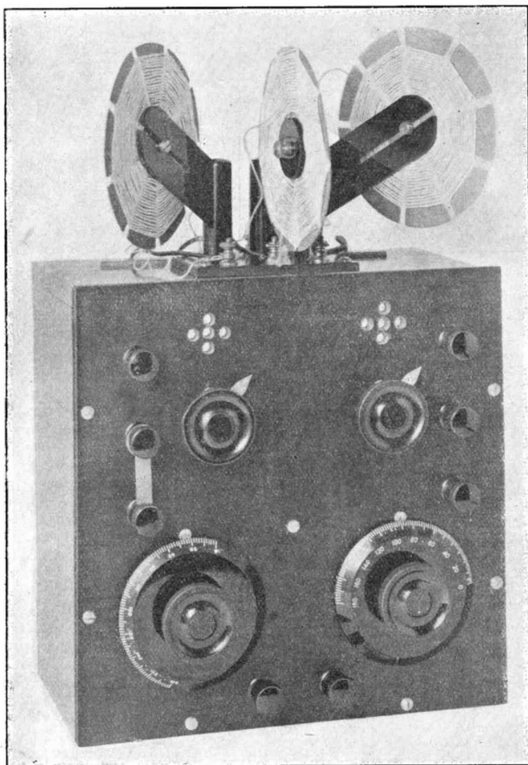
*Front view of the two-valve receiver.*
