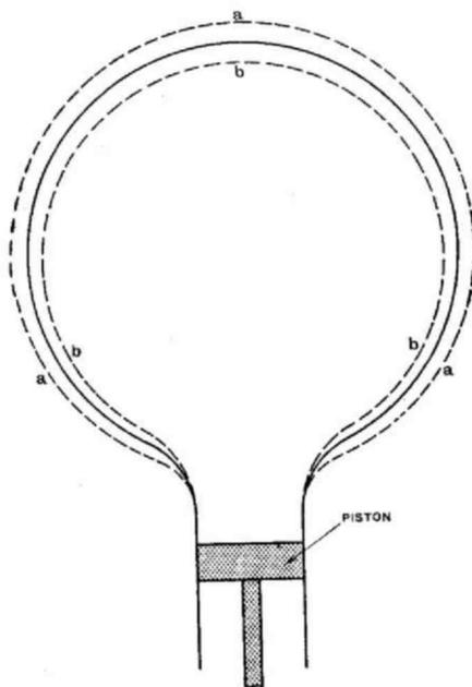
Fig. 1. Section of a toy balloon used in illustration of the production of sound waves.
