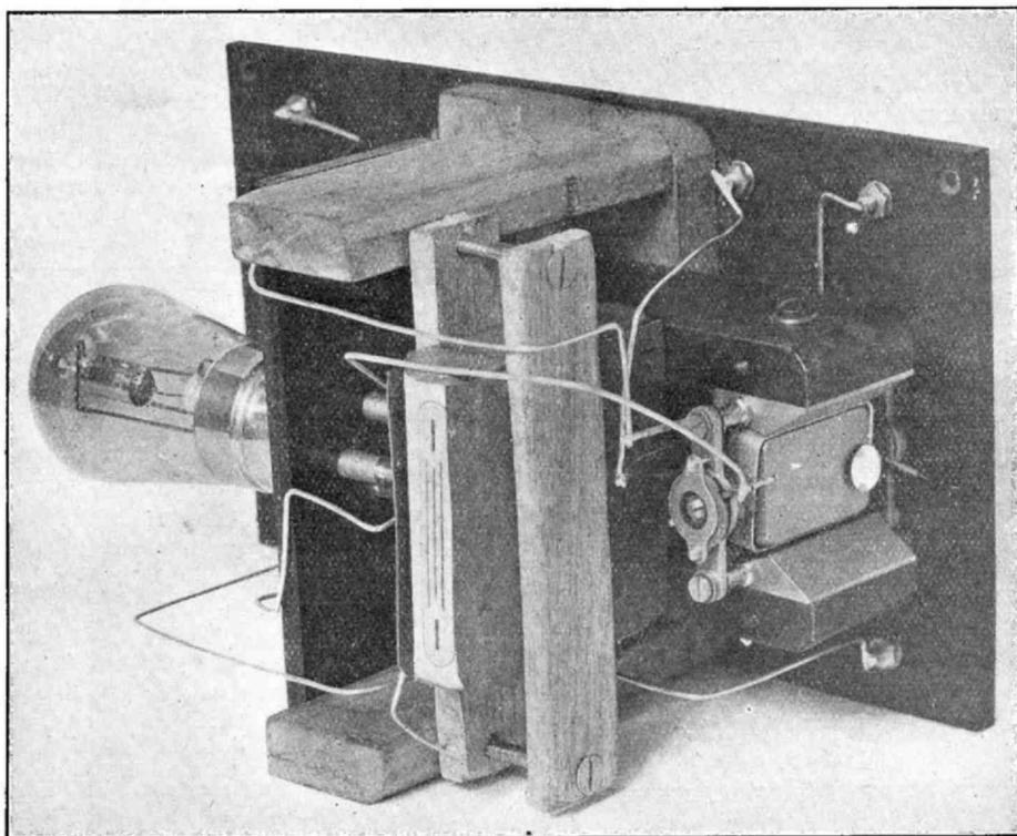
*View of the interior of the instrument. The small concave mirror is attached to the moving coil by means of an aluminium foil bracket.*
