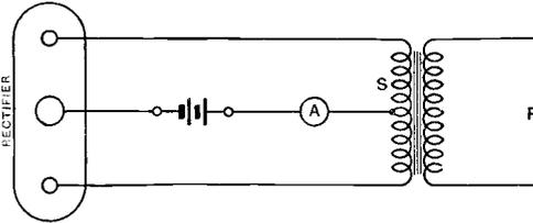
Fig. 2. Connections of a step-down transformer to a chemical rectifier for accumulator charging.
