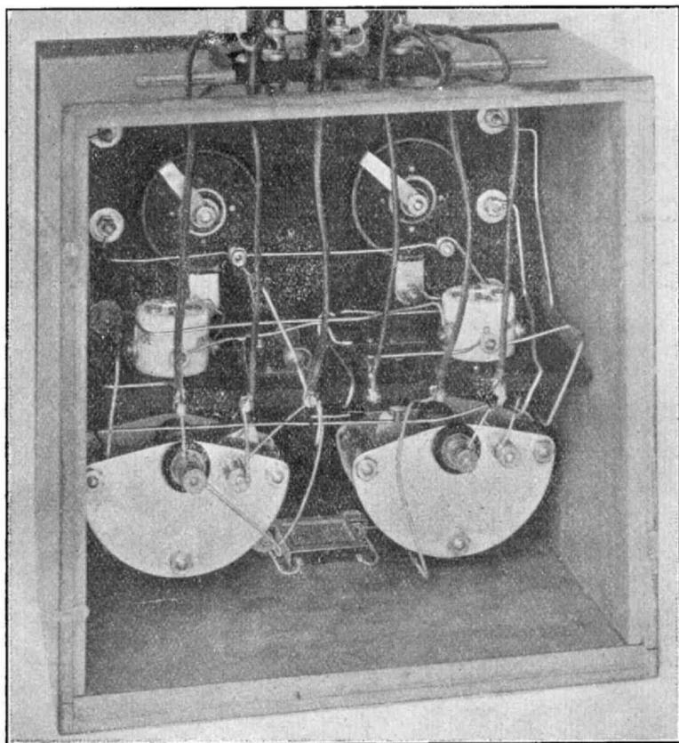
*A view of the receiver with the back removed to show the wiring.*
