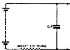
Method of connecting safety resistance to protect H.T. battery.
