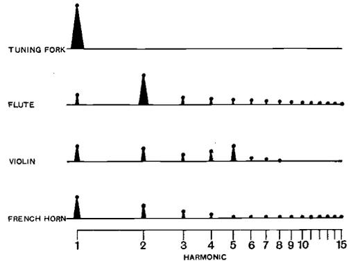
Fig. 14. Illustrating the frequency richness of various instruments.
