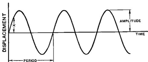
Fig. 4. Displacements of a sounding body producing a pure tone.
