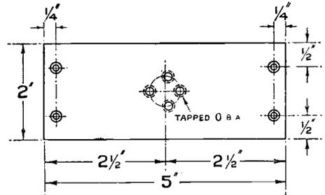
Fig. 5. The valve platform.
