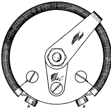
insulated covering. A suitable winding is No. 36 Eureka wire.
