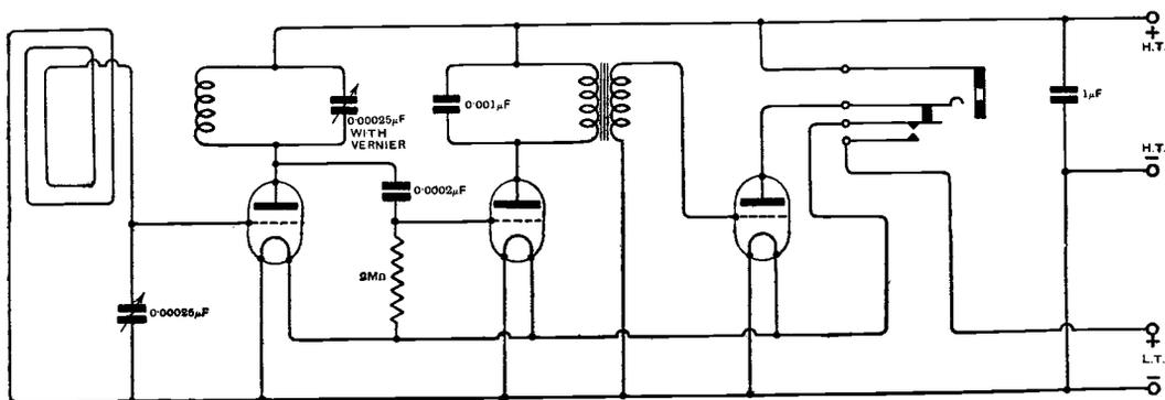
Fig. 1. Circuit of frame aerial receiver, with tuned anode high frequency amplifier, valve detector, and note magnifier. Reaction coupling is unnecessary owing to the low degree of damping possessed by the frame aerial.
