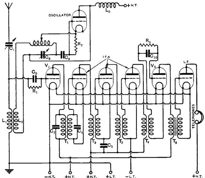
Fig. 2. Connections of the receiver.
