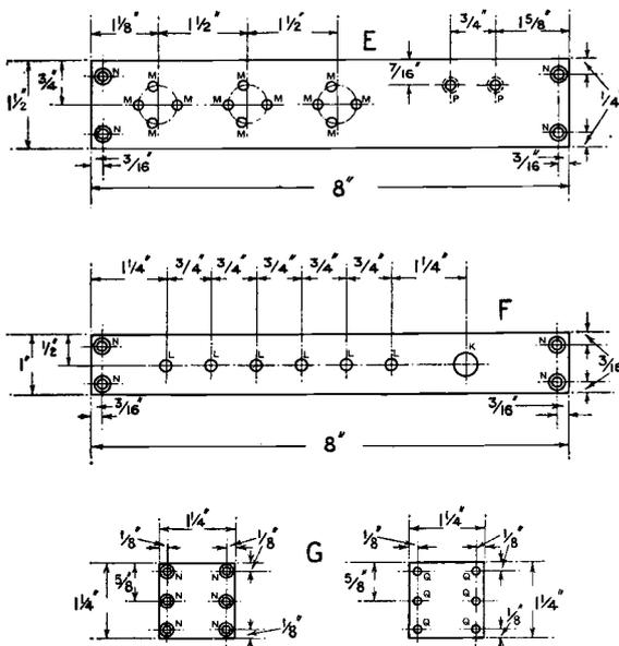
Fig. 3. The ebonite pieces, for valve holder platform, terminal strip and condensers. Size of holes; K  $\frac{3}{8}$ ", L  $\frac{7}{32}$ ", M  $\frac{5}{32}$ ", N  $\frac{3}{8}$ " countersunk on top side for No. 4 wood screws, P  $\frac{3}{8}$ " countersunk for No. 4 wood screws, Q  $\frac{1}{8}$ ".
