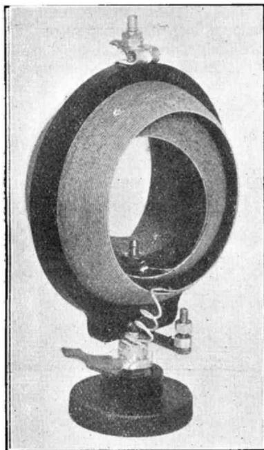
A variometer which appears to have desirable electrical properties is shown in the accompanying illustration. It will be
