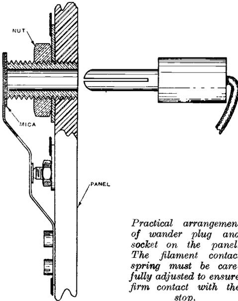
*Practical arrangement of wander plug and socket on the panel. The filament contact spring must be carefully adjusted to ensure firm contact with the stop.*
