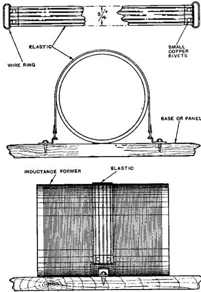
Coil fixing with elastic band.
