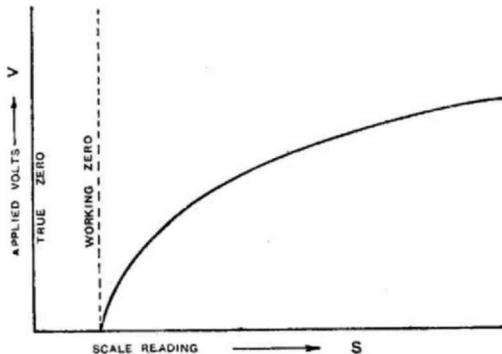
Fig. 7. Relationship between the applied voltage and scale deflection.
