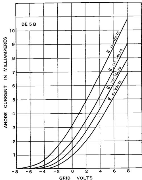
The valve takes a filament current of 0.22 ampere at 5 volts, which is similar to that taken by the D.E. 5 valve.
