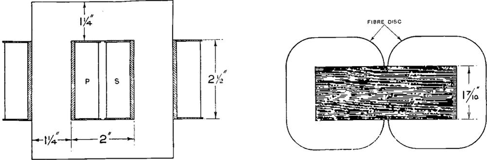
Fig. 3. Scale drawing of the transformer.
