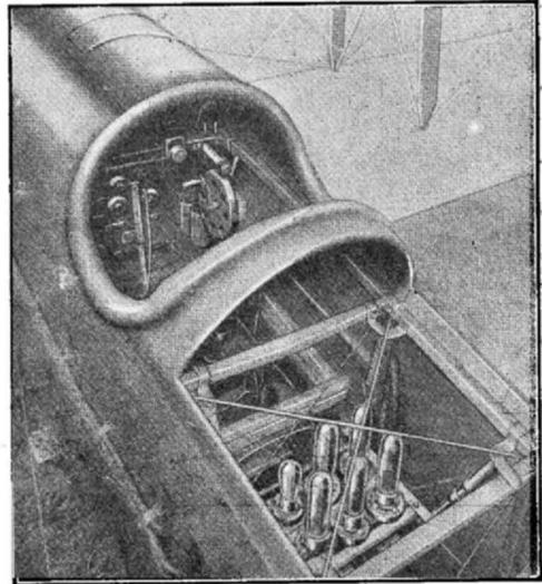
*The wireless equipment installed in an aeroplane.*
