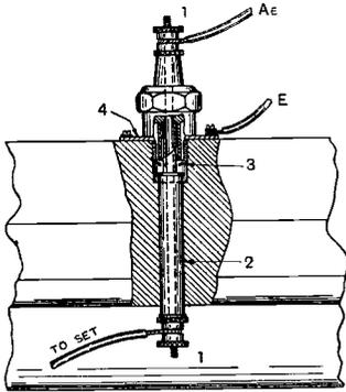
Fig. 1. A lead-in tube.
