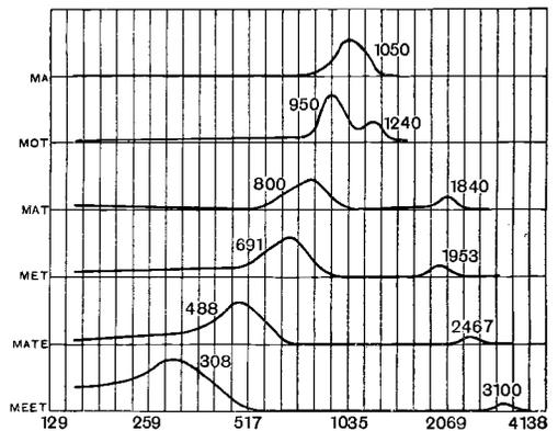
Figs. 17 and 18. Showing the energy distribution at different frequencies for various vowel sounds.
