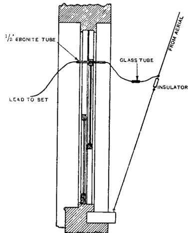
*By fixing your lead-in in this way opening and closing the window is not interfered with.*
