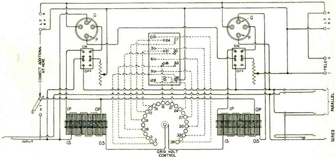
Fig. 5. Circuit diagram of two-valve power amplifier.
