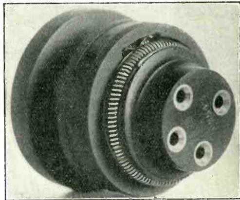
Another view showing arrangement of adjusting ring, resistance and valve socket.
