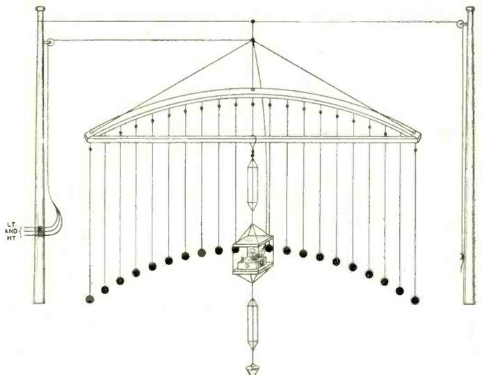
Fig. 3. Practical details of the reflector and suspension of transmitting apparatus and aerial.
