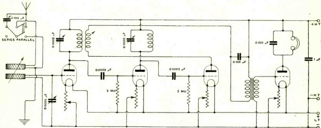
Fig. 4. "B.G.A." (Guernsey). Diagram of a four-valve broadcast receiver with two H.F. (tuned anode), rectifier and one stage of note magnification.
