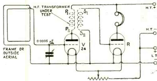
Fig. 12. Circuit with frame aerial for testing the H.F. Transformers.
