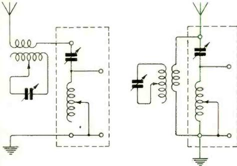
Figs. 5 and 6. Here the filter circuits are coupled with the aerial circuit. The coupling coil in the aerial circuit (Fig. 5) may have 5 to 10 turns. The coil across aerial and earth (Fig. 6) should be 3 ins. in diameter with 50 turns of No. 22 D.C.C. with a few taps.
