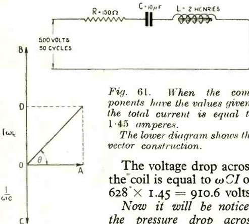
Fig. 61. When the components have the values given, the total current is equal to 1.45 amperes. The lower diagram shows the vector construction.
