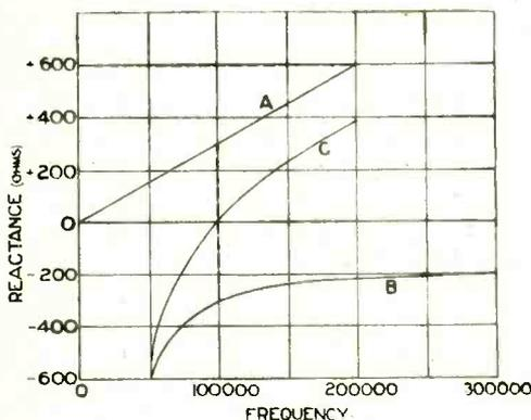
Fig. 63. Curves A and B represent the reactances of a coil and condenser at various frequencies. When both are connected together in a series circuit, the resultant reactance is given by curve C. The point where C crosses the zero reactance line is the resonant frequency of the circuit.
