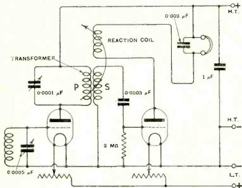
Fig. 3. Method of connecting an H.F. transformer and reaction to provide H.F. amplification.
