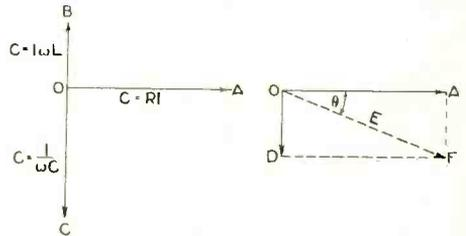
Fig. 60. Vector diagram showing phase relationship in a circuit such as Fig. 59.
