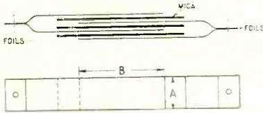
*It will be seen that the area of overlap is equal to  $A \times B$  where  $A$  is the width of one foil and  $B$  is the length of foil covered by a plate of opposite polarity.*
