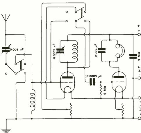
Fig. 3. "G.H." (Canterbury). Diagram of a two-valve receiver with H.F. and rectifier. A switch is connected to cut out the H.F. valve when required.
