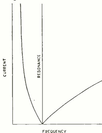
The curve shows the variation in current taken from the supply when the applied frequency is varied. At resonance the current is negligible, that is the circuit has a high impedance. To the left of the resonance point a larger portion of current flows through the inductance; to the right the condenser carries a larger current.
