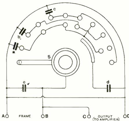
Fig. 1. Circuit arrangement for providing a wide range variable condenser.
