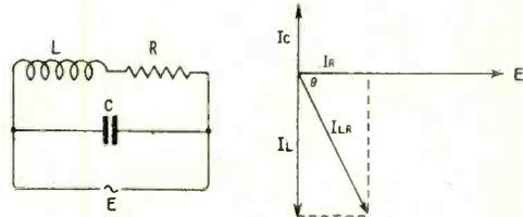
Fig. 67. A coil with inductance  $L$  henries and resistance  $R$  ohms in parallel with a condenser. The vector diagram shows the phases of the currents. The current  $I_{LR}$  is the current which flows through the resistance and inductance in series. The current from the mains is obtained by the method of Fig. 66.
