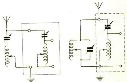
Figs. 3 and 4. Simple filter circuits joined with the receiver. The condenser may have a maximum value of 0.0005 mfd.
