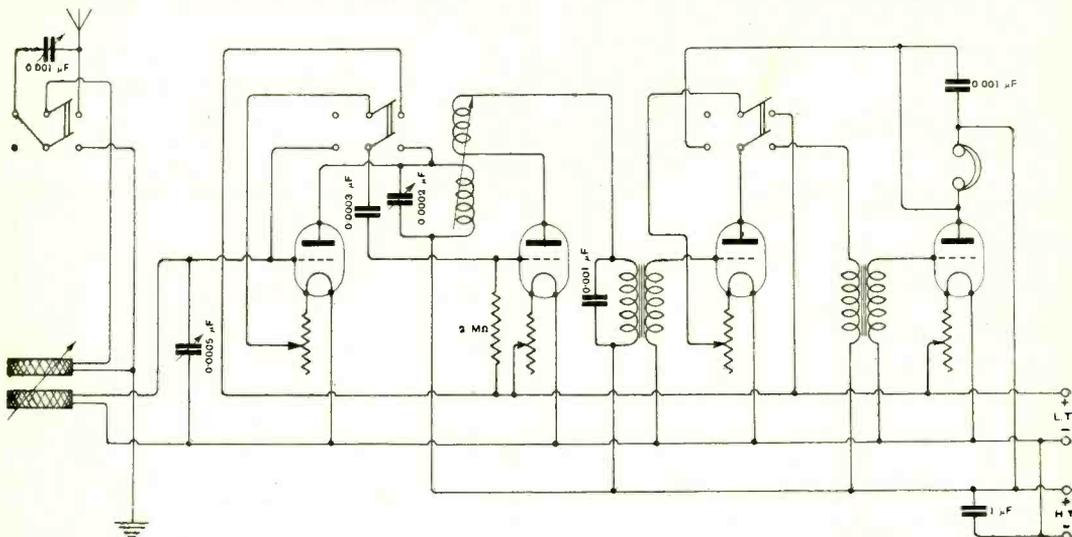
Fig. 4. "T.A.W." (Chingford). This is a diagram of a four-valve receiver with H.F., detector and two stages of note magnification. The H.F. and the last note magnifier may be switched out of circuit when desired. The tuned anode method of H.F. amplification is used and the reaction coil is coupled with this circuit. The circuit is suitable for broadcast reception.
