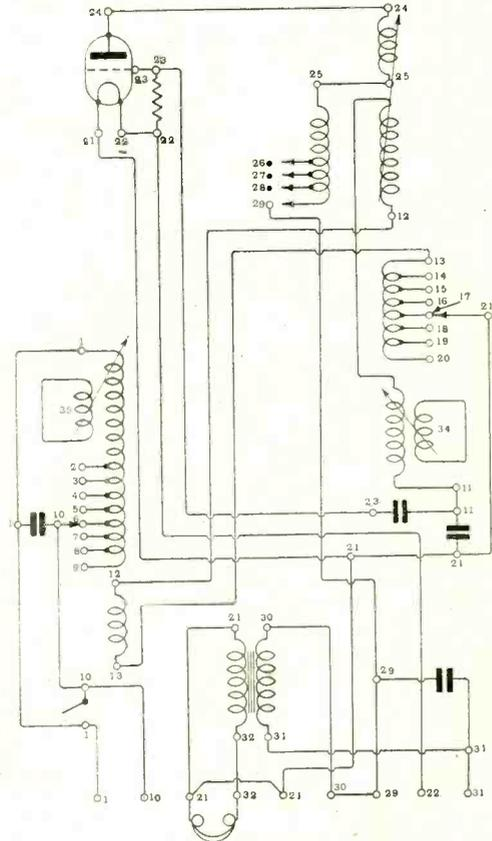
Fig. 4. Circuit of the tuner unit.
