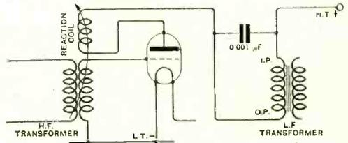
Fig. 6. "F.E.C." (Herts). Method of connecting a reaction coil.
