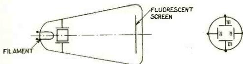
Fig. 3. The production of the Cathode beam used in the Cathode ray oscillograph.
