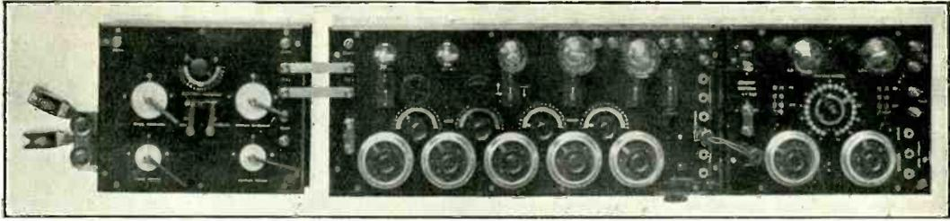
Fig. 2. The tuner, detector and amplifying units.
