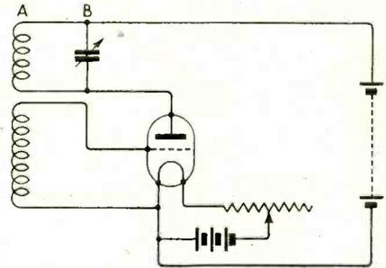
Fig. 11. Reacting valve for reducing the effective resistance of the grid circuit.
