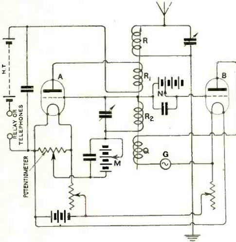
An abbreviated diagram of Capt. Bolitho's circuit.
