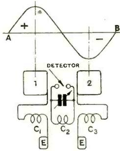
Fig. 7. Principle of the Weagant arrangement.
