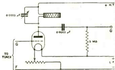
Fig. 2. "J.W." (Somerset). Method of connecting one stage of H.F. amplification with a receiver.
