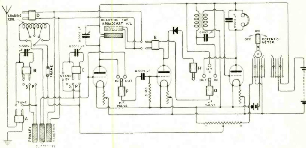
Fig. 2. Circuit showing how plug and socket connectors are provided for giving a variety of tuning systems.
