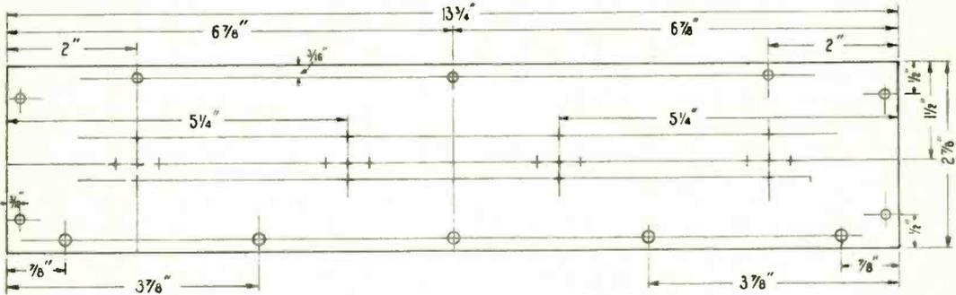
*Dimensional drawing of panel for four valve holders.*
