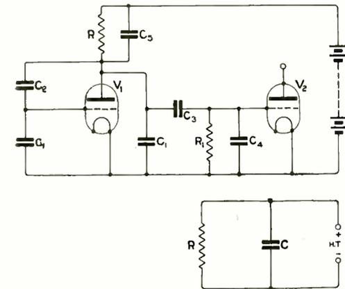
Fig. 56. Diagrammatic arrangement to show the capacities which shunt a resistance used in the anode circuit of a valve.
