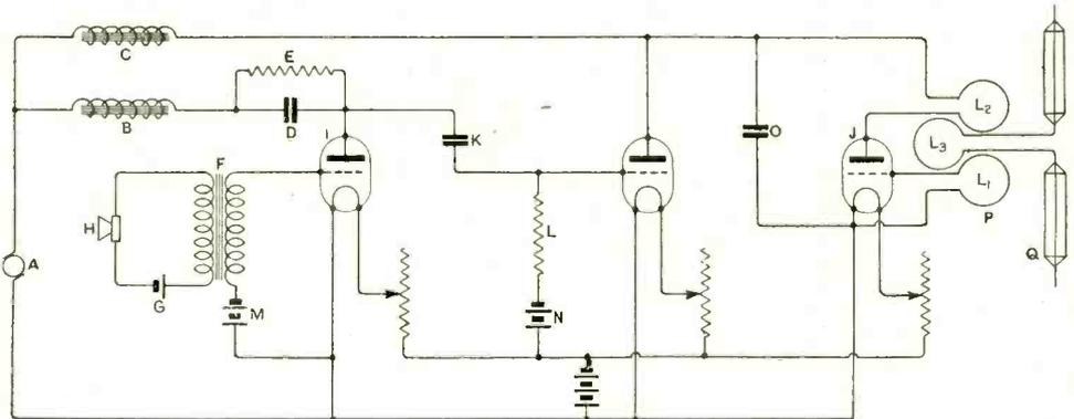
Fig. 9. Circuit of modulator for telephony for use with 10-metre wavelength directional transmitter.
