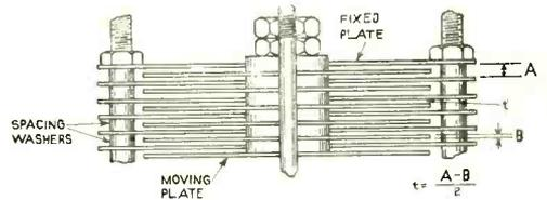
The figure illustrates a portion of a variable condenser. The distance between the fixed and moving plates,  $t$ , is obviously given by  $\frac{A - B}{2}$  where  $A$  is the thickness of a spacing washer and  $B$  is the thickness of a moving plate.
