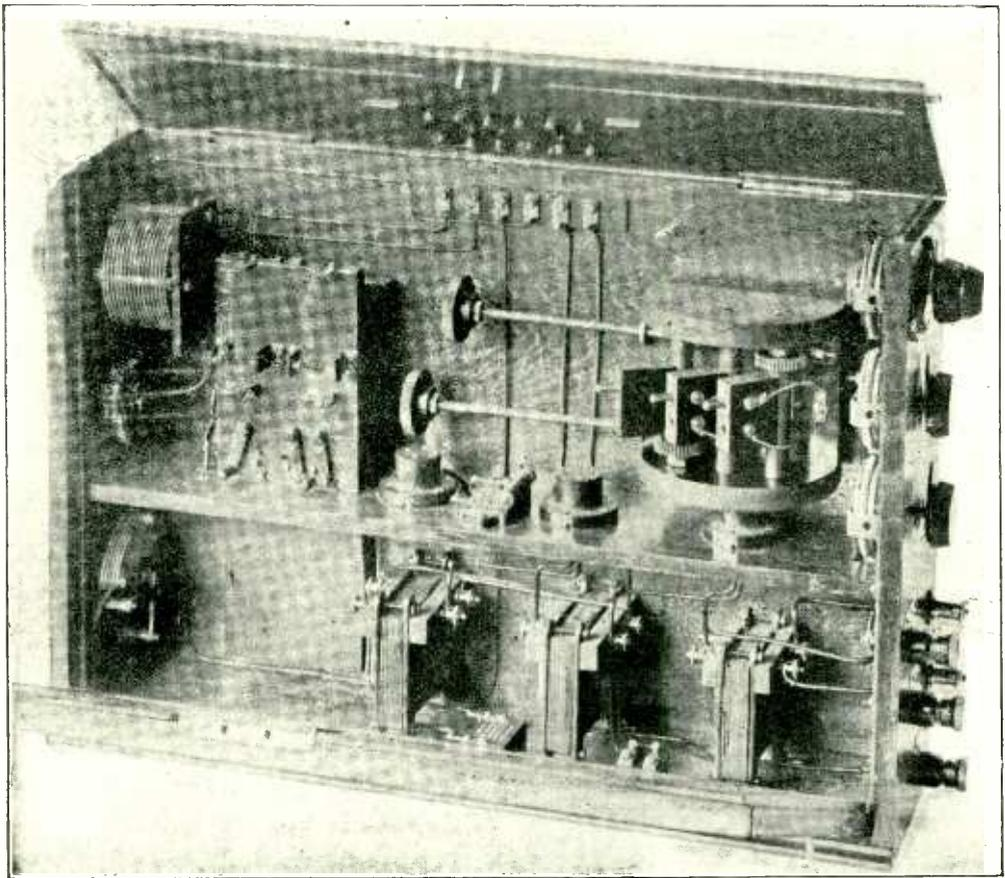
*Fig. 7. The Receiver with valves removed and coil holder transferred to the interior for portability.*
