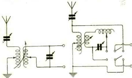
Fig. 2. A coupled circuit. Better selectivity is obtained by splitting the secondary coil. The coil which couples with the aerial circuit may be 3 ins. in diameter, with 10 turns. The other secondary coil may be 4 ins. in diameter and 3 ins. long of No. 22 D.C.C. with 10 taps.
