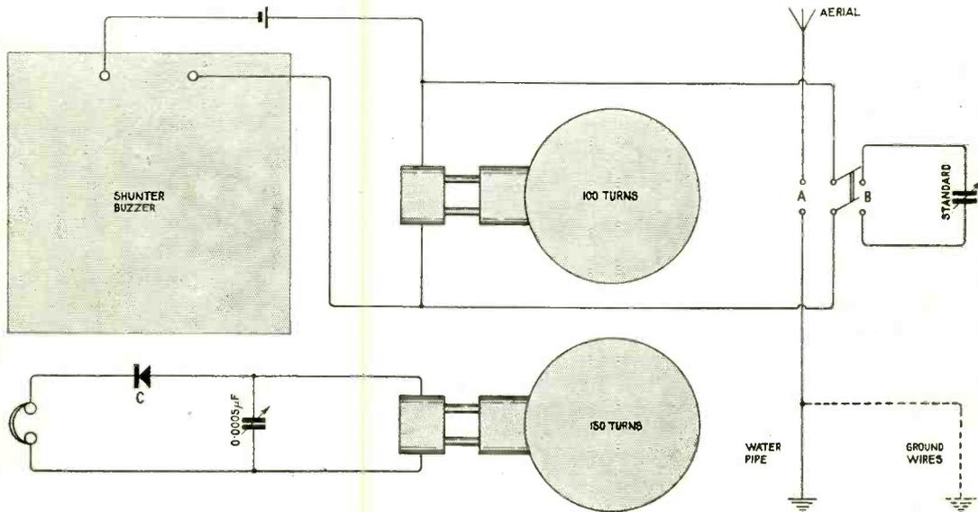
Fig. 14. Circuit arrangements necessary for determining the capacity of the aerial.
