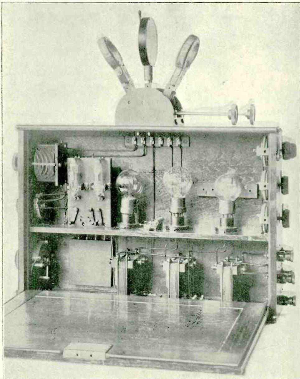
*Aerial circuit tuning is accomplished by variable condenser and plug-in coil. A closed circuit is arranged for selective tuning. The high frequency valves can be taken out of circuit by a switch and wander plug. Interchangeable transformers are used in the high frequency amplifying circuits. The low frequency valves are transformer coupled.*
