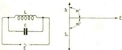
Fig. 65. A circuit with a condenser of capacity  $C$  farads in parallel with an inductance of  $L$  henries. The phase relationship is shown in the vector construction.
