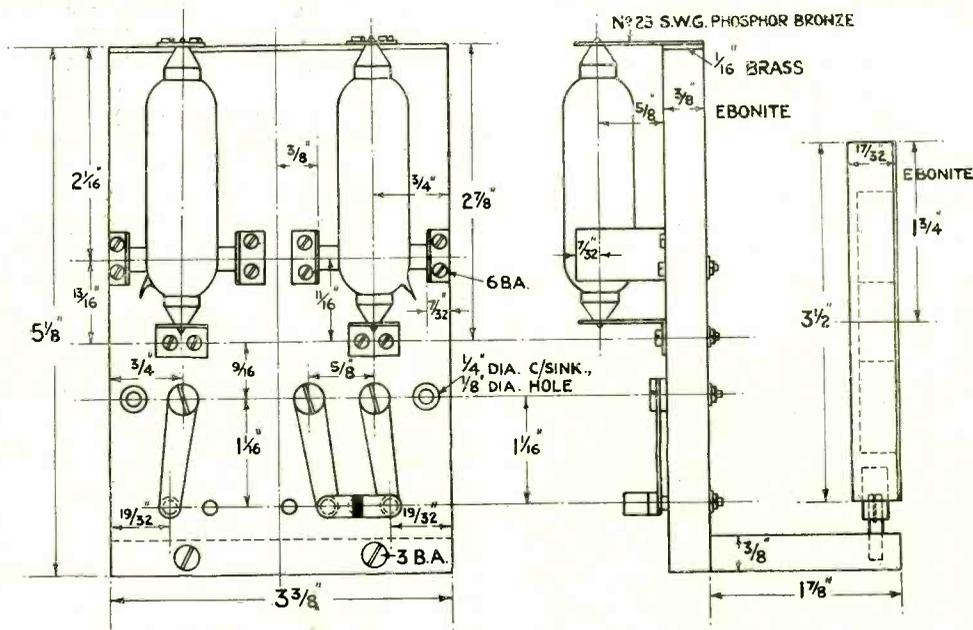
Fig. 10. Dimensions for setting out the H.F. valve panel.
