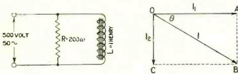
Fig. 54. The total current flowing in this parallel circuit is 2.96 amperes.
