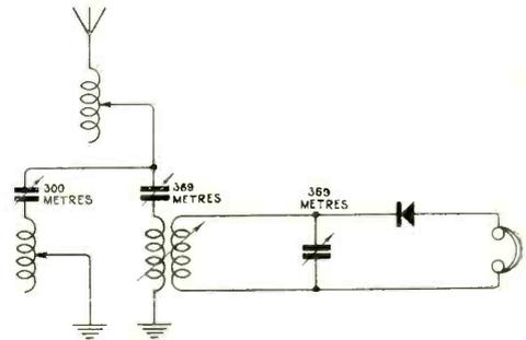
Fig. 5. A circuit arranged to eliminate interference by a particular transmitter.
