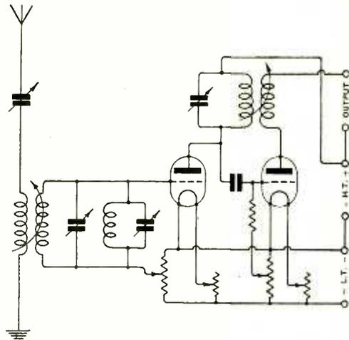
Fig. 13. Another circuit with rejector.
