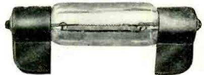
Fig. 13. Barretter tube of the type employed in receiving valve filament circuits for maintaining the current constant.
