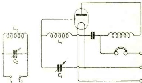
Fig. 1. Arrangement of test circuit for the measurement of the capacity of a condenser.
