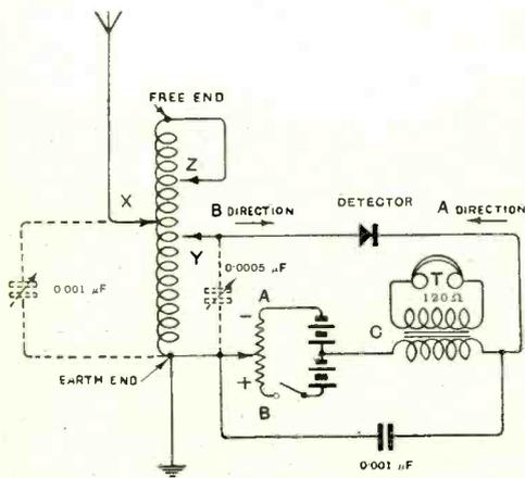
Fig. 15. Experimental Crystal Receiving Circuit.
