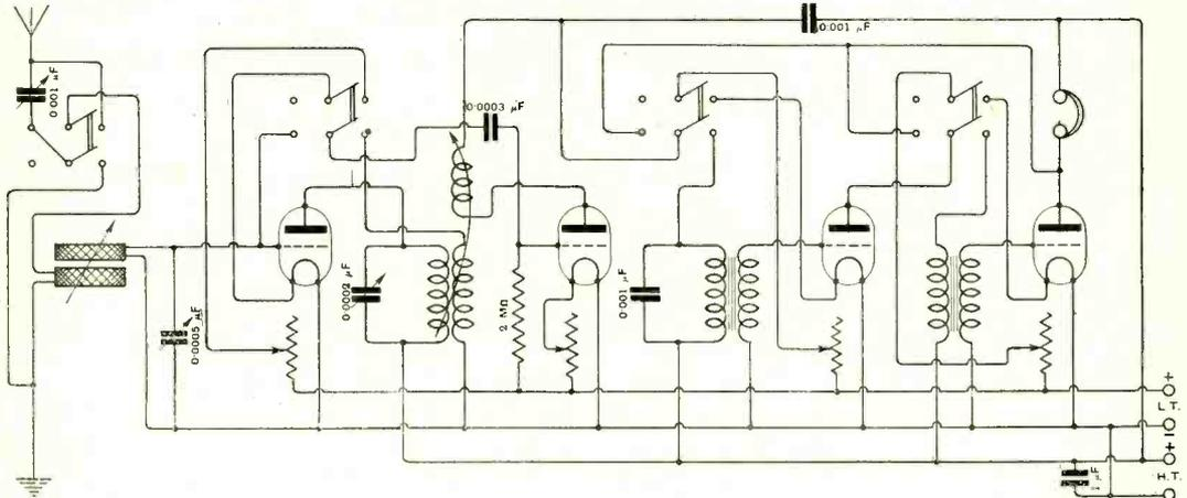
Fig. 5. "SIRKIT" (Lancs.). Connections of a four-valve receiver with H.F., rectifier and two note magnifiers. Switches are connected to cut out valves when required.
