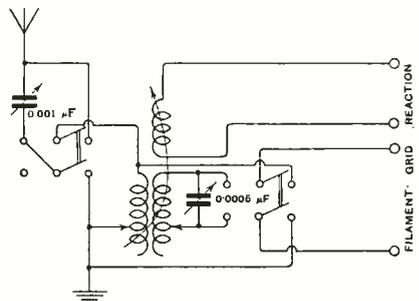
Fig. 4. "C.C." (Surrey). Showing the connections of a series-parallel, and a tune stand-by switch.
