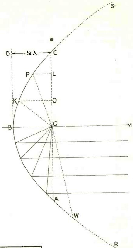
Fig. 5. The transmitter is located at the principal focus, which is arranged to be one quarter of the wavelength employed.
