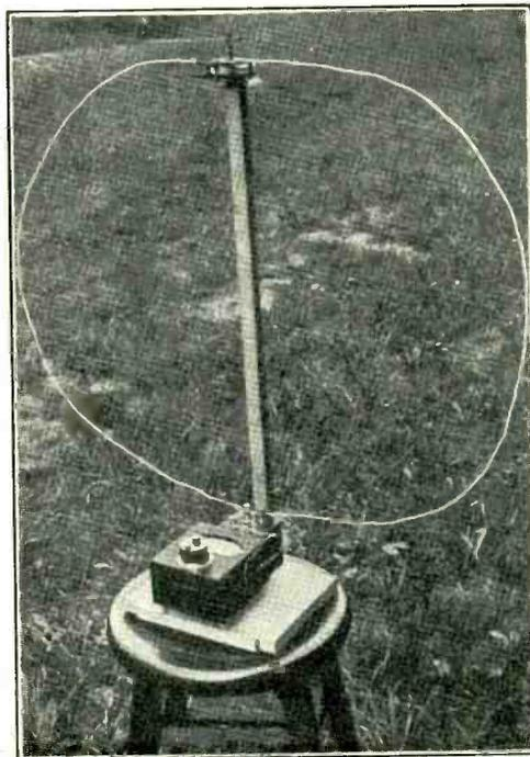
Fig. 6. Apparatus for determining radiation characteristic at short distances.
