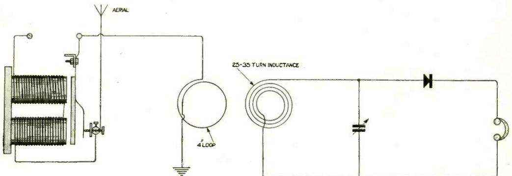
Fig. 13. Method of energising the aerial in order that the natural wavelength may be measured by the calibrated receiving circuit.
