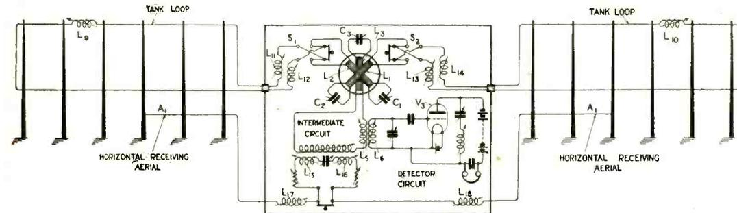
Fig. 9. Another and improved arrangement devised by Weagant.
