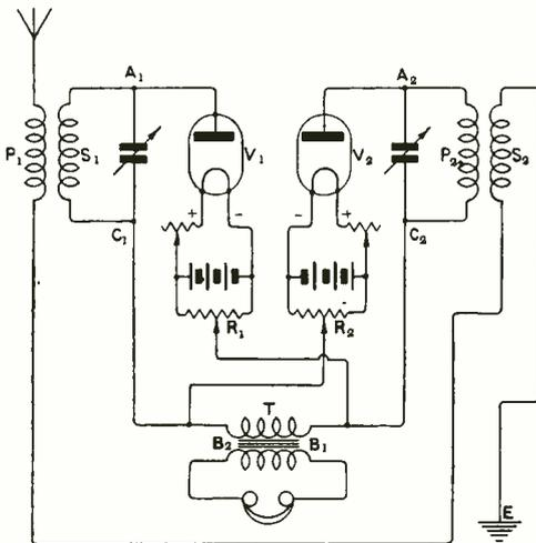
Fig. 5. Circuit arranged to eliminate interference.
