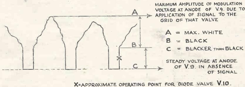
Fig. 3. Graph showing pictorially the voltage at the anode of the valve V.9 in the circuit diagram Fig. 1 shown on page 91 of last month's issue.
