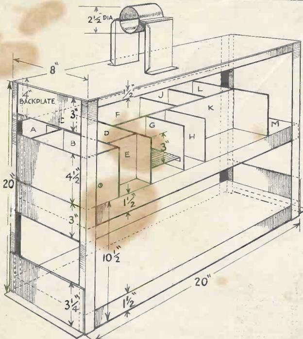
Dimensioned drawing of complete chassis.
