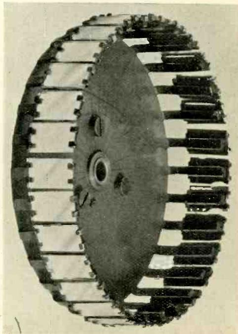
The completed drum with mirrors in position.
