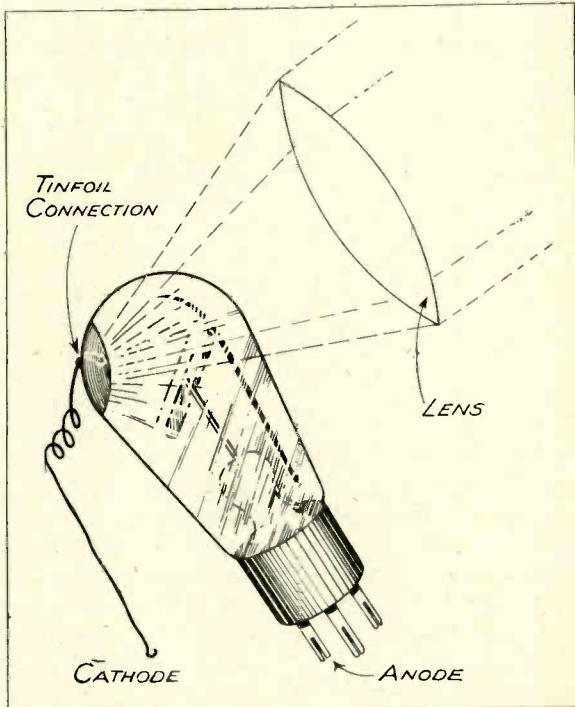
Diagram showing the light being directed from the lens to the valve.
