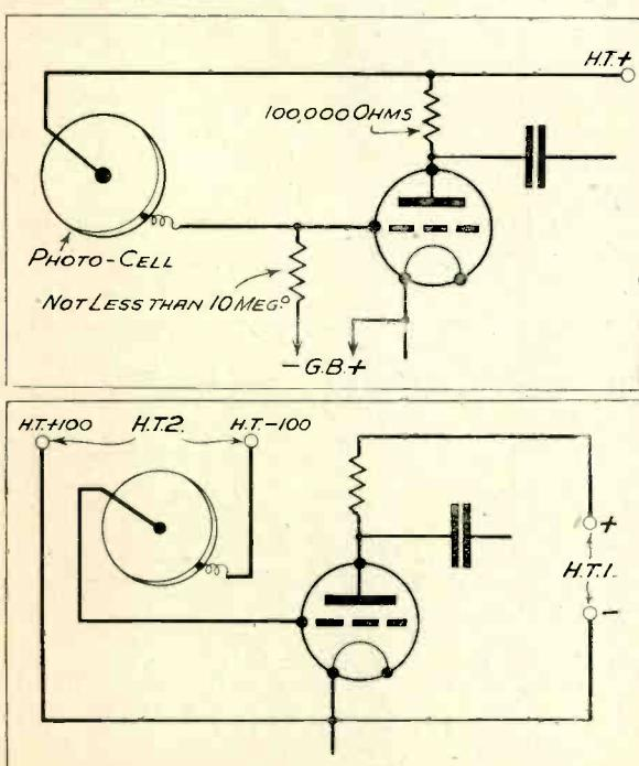
(Above) Method of coupling cell to first stage amplifier. (Below) An alternative method, which is more sensitive but requires two H.T. batteries; no grid leak is used.
