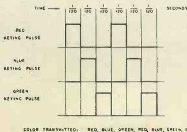
Fig. 8. Colour mixer pulse diagram.
