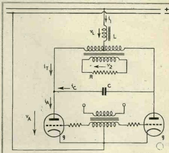
THE push-pull inverter with gas-filled triodes whose operation and mathematical theory have been described elsewhere† is a thermionic valve circuit for static conversion of direct current to alternating current. Current conversion is obtained at a high degree of efficiency owing to the relatively small power loss in the gas-filled valves.
