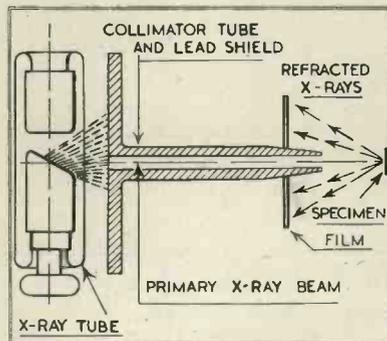
Fig. 1. Method of obtaining crystallograms by back reflexion.
