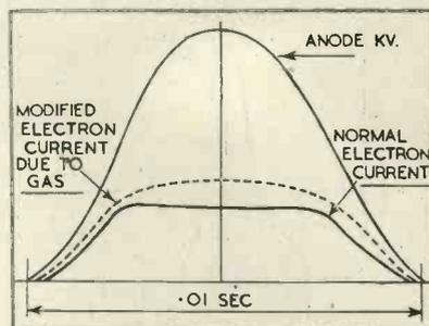
Fig. 3. Effect of gas in increasing emission over a half-cycle of anode voltage.
