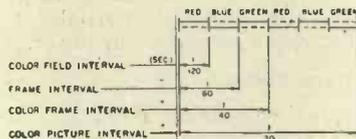
Fig. 1. Diagrammatic representation of CBS System 3.
