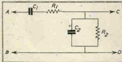
Fig. 5. Phase-shifting Network.
