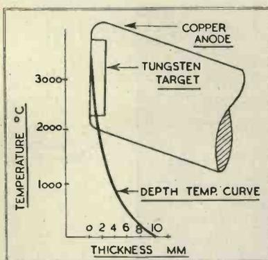
Figs. 6 (left) and 7 (right). Temperature curves of a tungsten-copper target showing variation across the surface and with target thickness.
