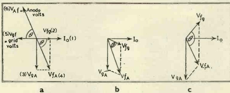
Fig. 4. Vector diagrams for the grid circuit of Fig. 3.
