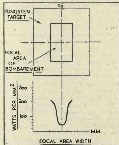
Fig. 11. Variation of power dissipation across the surface of the target.
