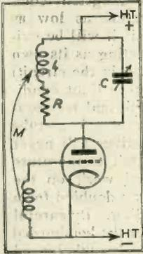
IN the case of low or medium frequency oscillators, an oscillatory current started in an L.C.R. circuit in the anode lead of a valve by attaching the H.T. + lead can be maintained by mutual coupling between the coil of the tuned circuit and a coil placed in the grid circuit, provided  $M$  in the figure above is of the correct sign and is equal to or greater than:
