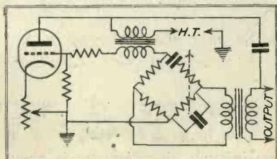
Fig. 3. Audio-frequency Oscillator using Wien Bridge.
