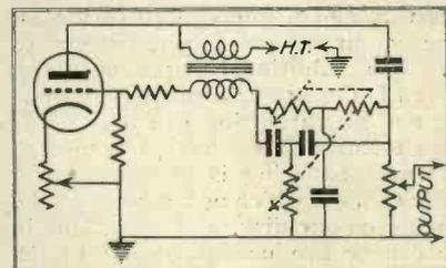
Fig. 4. Audio-frequency Oscillator using parallel-T network.
