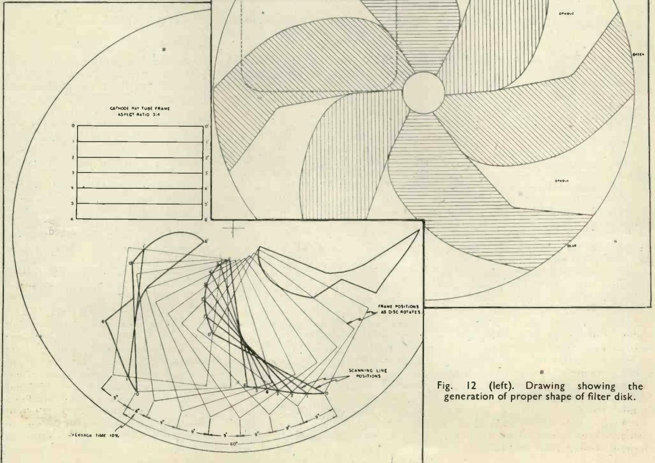
Fig. 12 (left). Drawing showing the generation of proper shape of filter disk.
