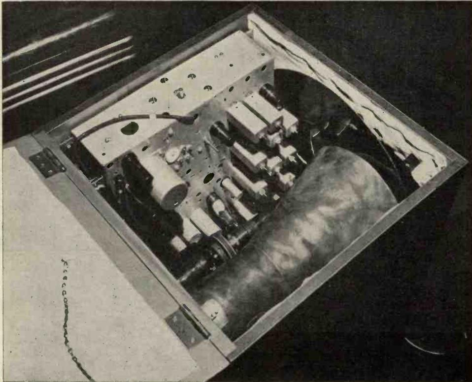
Fig. 11. The interior view of a 9" colour television receiver showing filter disk and cathode ray tube (lower right).
