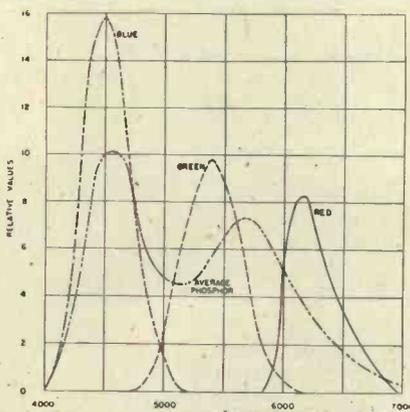
Fig. 2. Colour characteristics at the receiver: colour filters Nos. 47, 58 and 26 combined with the phosphor. The fourth curve represents an average phosphor.
