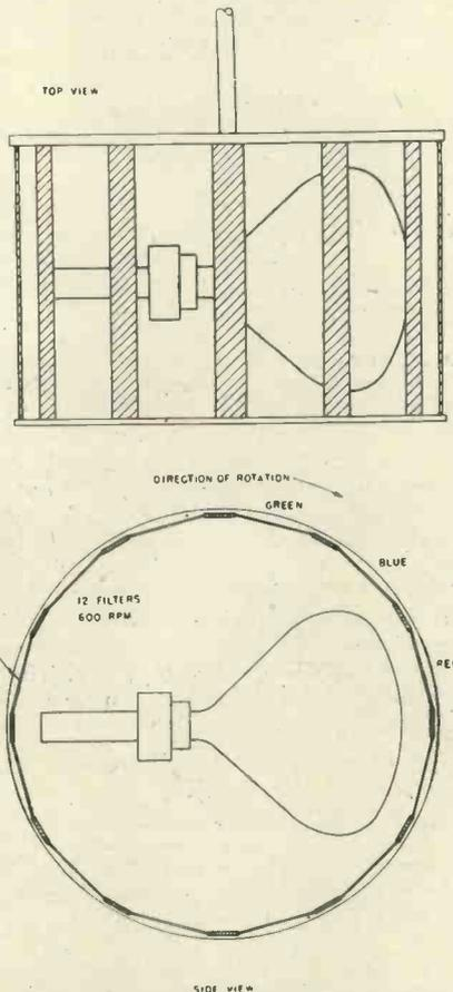
Fig. 14. Diagrammatic view of drum receiver for colour television.
