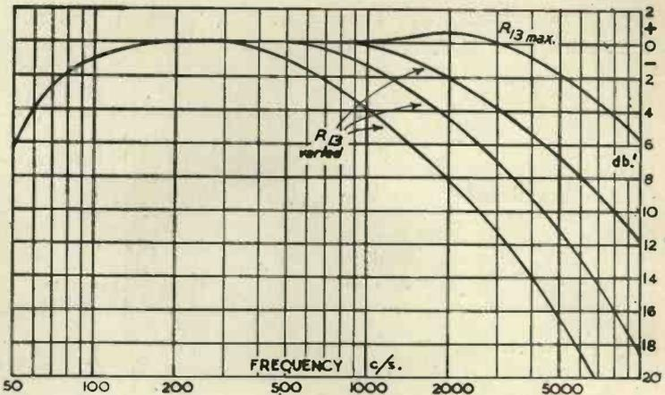
Fig. 35. Effect of tone control  $R_{13} C_{17}$  (Fig. 34) on audio frequency response.
