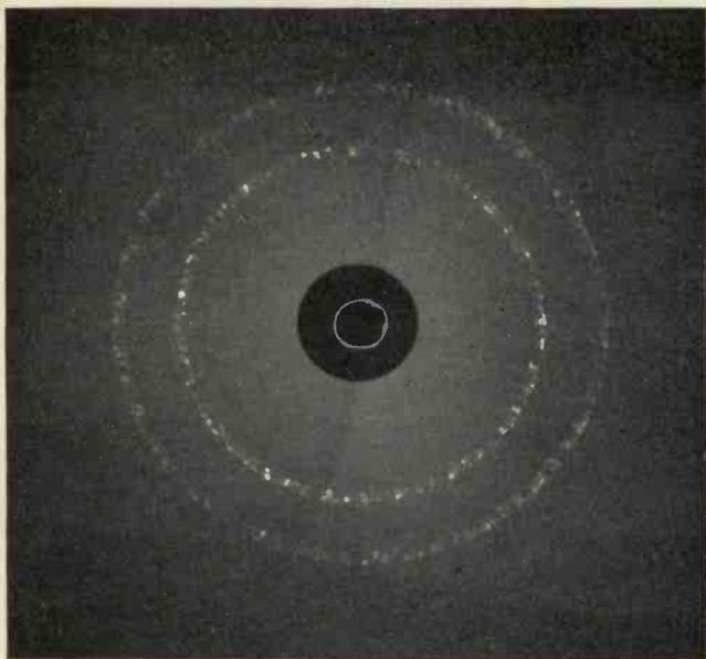
Fig. 2. Crystallogram obtained by the method of Fig. 1.
