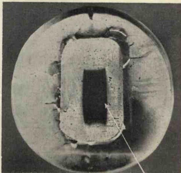
gives the almost true view. It will now be evident that the stresses produced by unequal thermal expansion are very severe.
