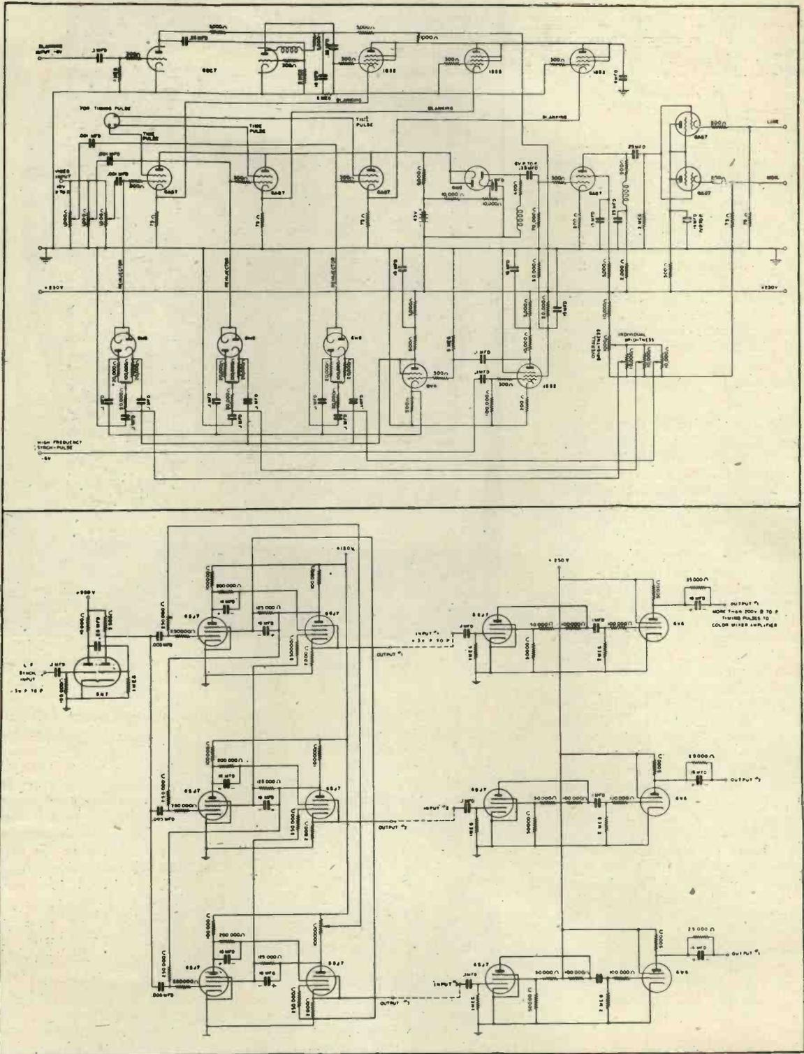
Fig. 7 (top). Circuit diagram of colour mixing amplifier.
