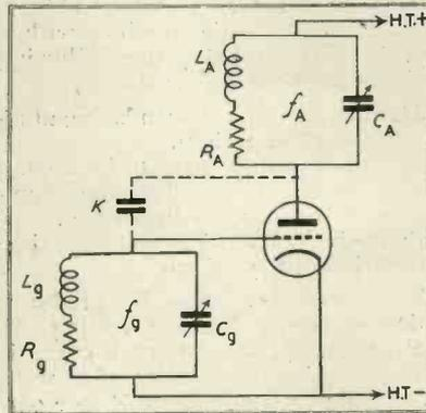
Fig. 2 (above), Circuit of tuned anode-tuned grid oscillator and Fig. 3 (right) the equivalent circuit.
