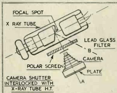
Fig. 8. Method of obtaining photograph of target.
