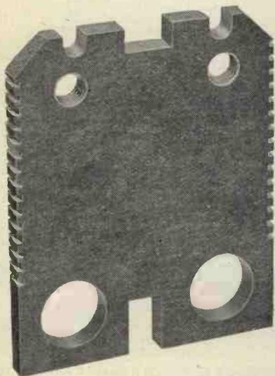
*(Left) MYCALEX sheet, cut, milled, trepanned, tapped, without fracture or crumbling and with all edges sharp and true.*
