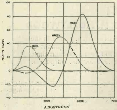
Fig. 3. Colour characteristics at the transmitter: calculated on the basis of receiver characteristics represented in Fig. 2.
