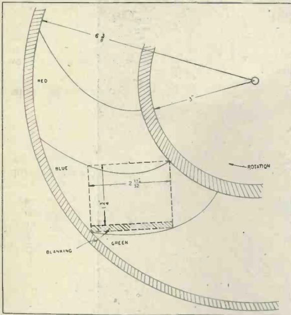
Fig. 10. Drawing showing portion of filter disk for orthicon camera.
