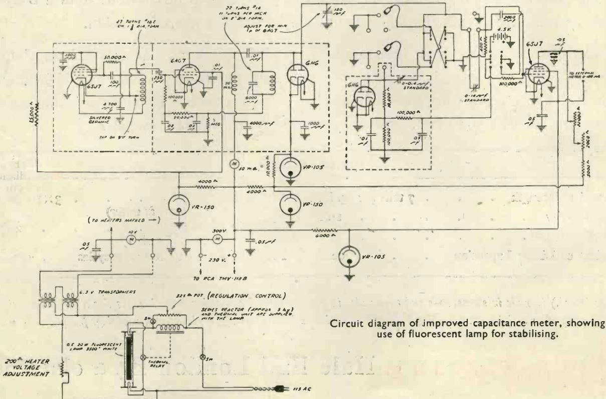
Circuit diagram of improved capacitance meter, showing use of fluorescent lamp for stabilising.
