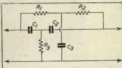
Fig. 2. Equivalent Parallel-T Network.
