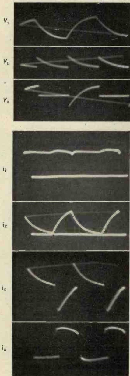
Fig. 4. Oscillograms of the voltages and currents at various points in the circuit. The lettering against each oscillogram corresponds to the lettering on the circuit diagram.
