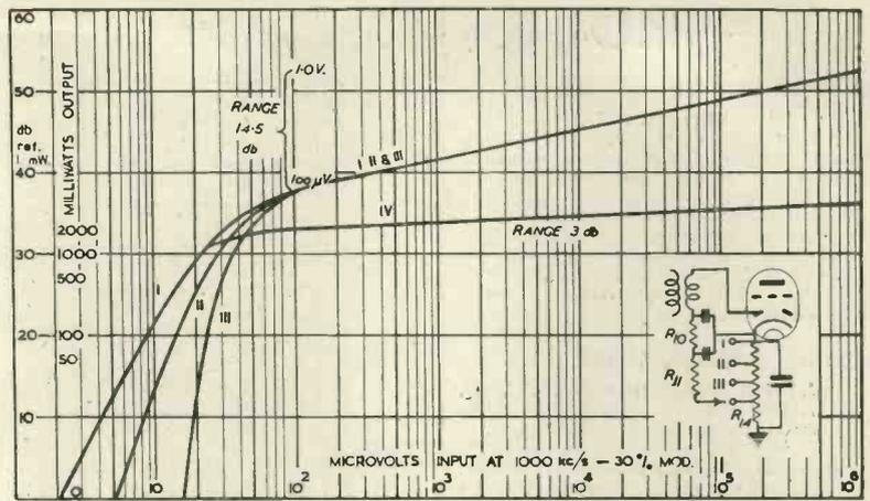
Fig. 33. A.V.C. characteristics. (i) For two controlled stages of conventional receiver with -3 v. delay. (ii) as (i) but with -1 v. at signal diode. (iii) With -1.5v. (iv) is the same as (i) but with A.V.C. also applied to the 1st A.F. stage.
