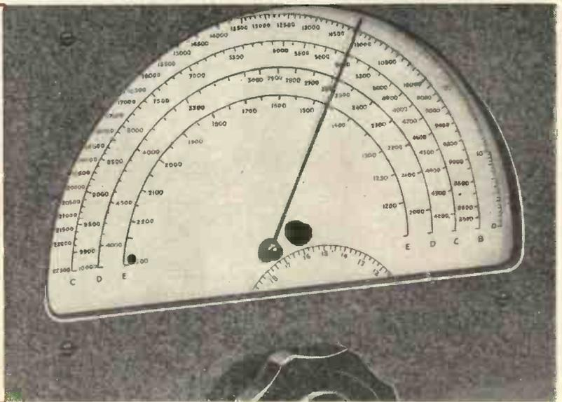
**EDDYSTONE "358" Communication Receiver.** *Specification:* The receiver employs one stage of R.F. amplification, frequency changer, two I.F. amplifiers, a separate beat frequency oscillator, octal base Mullard or Osram 6.3 volt valves. Frequency range is continuous from 22 M/cs to 1.25 M/cs using four fully screened interchangeable coil units. *Five additional coil units extend the range to 31 M/cs, and 90 K/cs.* Illuminated dial is accurately calibrated with
