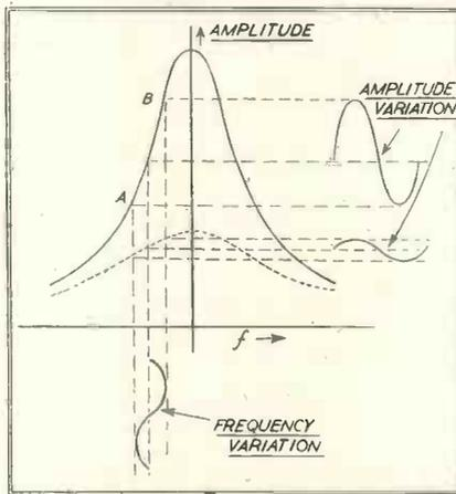
Fig. 1. Frequency Amplitude conversion of a detuned circuit.
