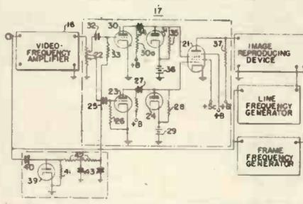
The video-frequency signal is supplied to the amplifier 17 from the output of the amplifier 16, and appears
