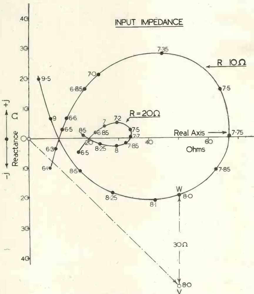
Fig. 5. Input Impedance diagram for two values of R.
