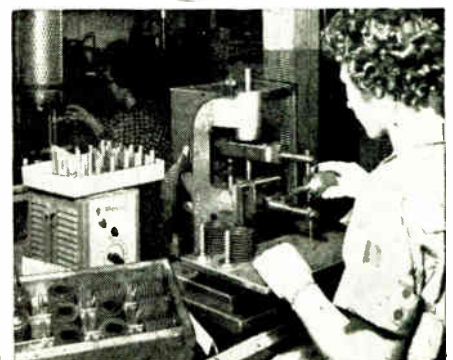
Below: An Eisler precision vertical Spot Welder designed exclusively for welding electronic components. Sizes from 1/2 to 7 1/2 KVA
