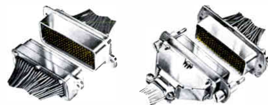
SERIES "A" —Meets electrical and environmental requirements of MIL-C-26518. Metallic shell—sealed or unsealed—50 and 100 positions. Rack and panel or bulkhead mounting. Screw-machine contacts exclusively. Center to center spacing of .150".
