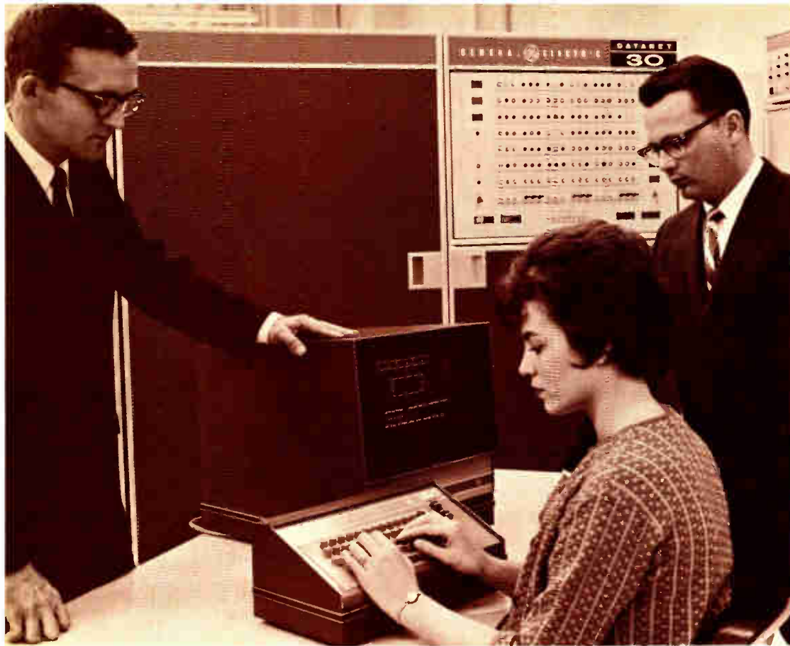
Fig. 1: Data communications secretary operates Datanet-760 keyboard display terminal. Datanet-30 data communications processor in background automatically schedules communications flow and monitors messages in and out of the computer center.
