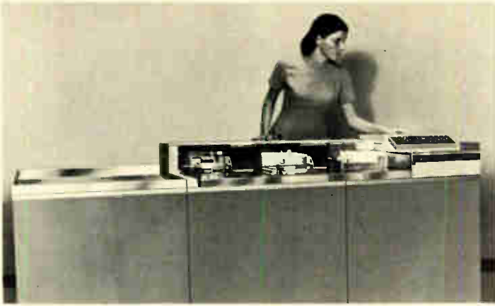
RCA Spectra 70/251 Videoscan Document Reader reads up to 1,800 documents/min. continuously and up to 1,300 documents/min. on demand.
