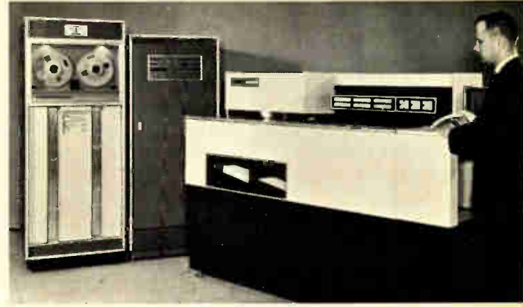
The Control Data Corp. 915 Page Reader is shown with the 8092 Teleprogrammer (center) and the 603 Tape Transport (at left).
