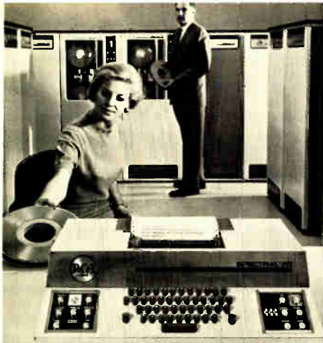
Fig. 2: Main control console and some of the operating equipment of RCA's Spectra 70 family are shown in this photo.
