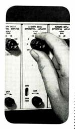
1000X Amplification, high common mode rejection
