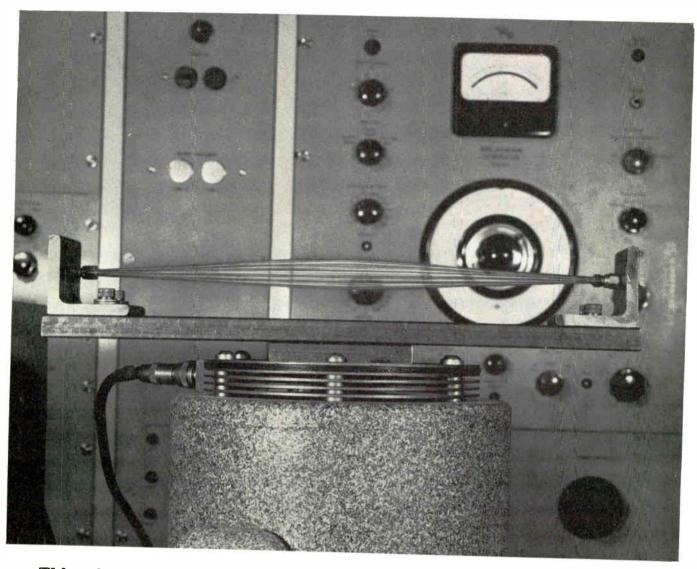
This miniature coaxial cable of ours was vibrated at resonance 7 hours before the sheath cracked. The best competitive cable lasted 55 minutes.
