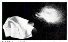
FIBER for ablative and radome applications. Comes in yarn, roving, wool and matt, readily fabricated into cloth or tape.
