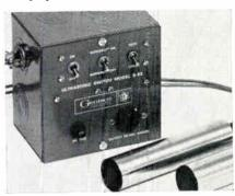
Model S-82 consists of a transmitter, receiver and control unit. The transmitter contains an 82kc piezoelectric trans-ducer. Transmitter power is supplied by the control unit or by battery if separation of the 2 units is desired. The control unit converts 60 cps, 110v. to low voltages for the transistorized transmitter, receiver, relay driver and switching circuits. Electronic Components Div., Genisco Technology Corp., 6320 W. Arizona Circle, Los Angeles, Calif.
