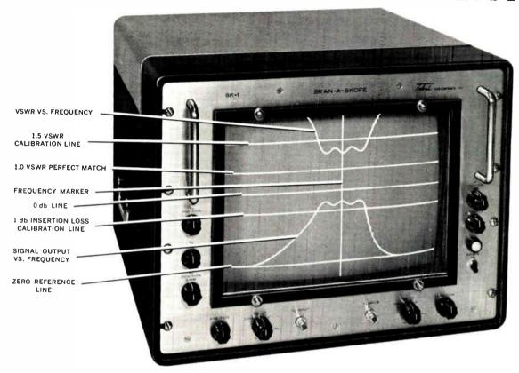
3 TRACES plus 2 REFERENCE LINES or 2 TRACES plus 3 REFERENCE LINES or 1 TRACE plus 4 REFERENCE LINES
