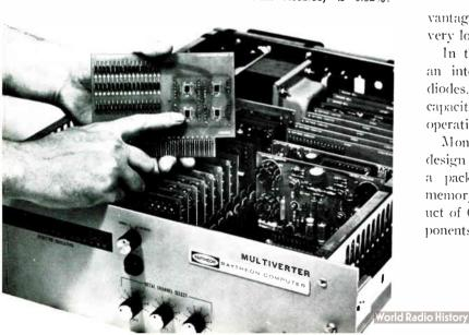
system. To simplify connector wiring, the device uses an integrated diode selection matrix (indexing circuits), which reduces the number of peripheral components.
