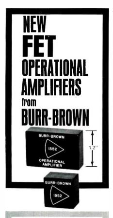
These new general purpose dc operational amplifiers employ matched junction FETs in the balanced input stage to achieve high input resistance and unusually low drift. Designed for ±10 volt service, units have an operating temperature range of -40 to +85°C. Model 1552 is supplied in a modular 1.8" x 1.2" x 0.6" package. Model 1952, designed for high density applications, is 1.0" x 1.0" x 0.7". Units are priced at \$145 and \$165.
