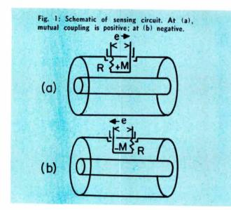
The output voltage,  $e_r$  is the sum of two samples:  $e_R$  from the division of E by R and C,
