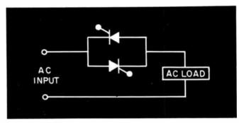
Fig. 9: A basic inverse parallel connection-ac output.
