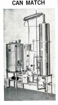
This NEW Still produces better quality distilled water than any other Still including triple distillation types. Special patented high purity features insures water of 0.1 ppm or less — ten times purer than ordinary distilled water.
