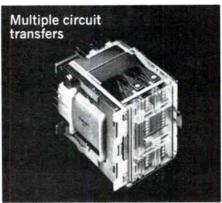
CLASS W RELAY. 17, 34 or 51 form C contact-spring combinations. Features low loss insulation, high insulation resistance. Extremely low inter-spring capacitance. Life in excess of one billion operations. Gold contacts available for low-level switching.
