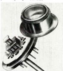
Model 094447 is a 2-stage cascade thermoelectric unit. It is capable of achieving a zero load temp. differential of 85°C. Carrying a 15mw heat load, this cooler will maintain the cold plate junction at -58°C in a vacuum of 10-6 Torr with a +27°C heat sink temp. Cooler performance including vacuum level is guaranteed for 1 year. A 4w. heat sink is required, while input power is 3.5a. @ 1.1vdc. Borg-Warner Thermoelectrics, Wolf & Algonquin Rds., Des Plaines, Ill. 60018.
