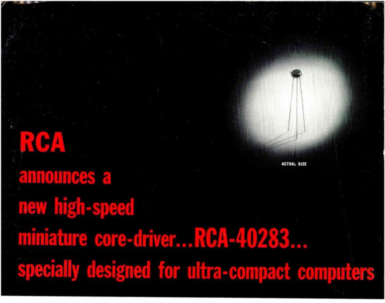
Now-commercially available, this tiny new RCA-40283 N-P-N silicon core-and-line driver packs substantially all the performance of TO-5 core drivers into a tiny TO-46 case.
