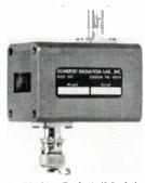
Model X430 Switch/Modulator/Voltage-Controlled Attenuator has its switching diodes connected in series, instead of the usual parallel. This allows a choice of either polarity grounded biasing or straight through bias drive in an ungrounded system. Min. attenuation of 3db or less is realized from 8.5 to 9.5gc with a total diode current of 150ma. Modulation freq. are dc to 500mc. Modulation is 99% from 8.2 to 10.5gc. Somerset Radiation Laboratory, Inc., Box 201, Edison, Pa. 18919.
