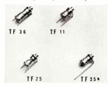
The TF series is sealed and features a non-rotating piston construction. The "O" ring seal provides protection during user assembly, soldering, cleaning, encapsulation and in the field. The unique design offers long life, low inductance, low resistance, high "Q" and no self-resonance below 1200 mc. Operating working voltage is 750 and 1000dc; min. "Q" is 700 to 11100 @ 1 mc and 500 to 1000 @ 20 mc. Linearity is ±1% with no capacitance reversals. Voltronics Corp., 296 Route 10, Hanover, N. J.
