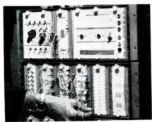
The MBK2 silicon module breadboard kit provides a simple and convenient method of developing and testing circuits. A basic kit can accommodate up to 10 modules. The kit contains a power supply, a 1 pps to 1 mc signal generator for static or dynamic circuit analysis, and an indicator panel with lights for visual observation of circuit operation. Circuit wiring is then done with external patchcords. Raytheon Computer, 2700 So. Fairview St., Santa Ana, Calif. 92704.
