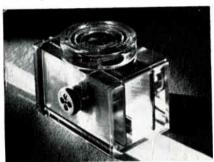
In this Kerr cell the windows are flat to a quarter wavelength and are low-reflection coated for 6943Å. The device is hermetically sealed and filled with hyper pure nitrobenzene. This eliminates space charge effects, produces an extremely uniform electric field, and creates a uniform and complete closure. Electrode separation or aperture width is 0.8 in. and aperture height is 1.5 in. Kappa Scientific Corp., 5785 Thornwood Ave., Goleta, Calif.
