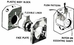
A rotor, mounted on an eccentric shaft in this plastic pump, rotates within a liner to create a progressive squeezing action on fluid trapped between the liner and the body block. All metal parts and mechanical action takes place inside the liner where fluid never reaches. This completely eliminates the need for stuffing boxes or shaft seals, guaranteeing no leakage.
