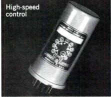
CLASS V MERCURY-WETTED RELAY. For computers, data processing and control equipment. Up to 200 operations per second. No contact erosion, no bounce. Over 1 billion operations without change, maintenance or adjustment. Can be operated within 30° of vertical. Polarized and nonpolarized versions. 1 pole to 4 pole double throw contact forms.
