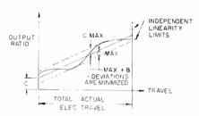
Independent linearity limits are shown with the output ratio vs. total elec. travel.
