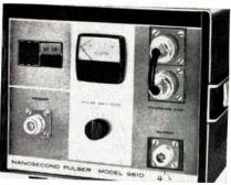
Model 961 provides high-voltage nsec. pulses for R&D, engineering and calibration uses. Amplitudes are adjustable from 0 to 3kv. Repetition rate is at 1 cps, line freq., or pushbutton actuated. The primary use is for simulation of scintillations from nuclear events by driving nsec. light sources. Other uses include photosynthesis timing, impedance measurements, multiplier phototube testing. Huggins Laboratories, 999 E. Arques Ave., Sunnyvale, Calif.
