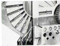
The Librafile 4800 mass memories are available in a basic 6-disc configuration. Storage capacity is 400 million bits, and data transfer rate is up to 150 million bits/sec. By combining 16 files on a single trunk line, an on-line storage capacity of 6.4 billion bits can be achieved. The memories have a fixed-head/track, two methods of search and retrieval, and retractable head plates. Retractable mounting plates permit easy maintenance. General Precision, Inc., Librascope Group, Glenside, Calif.
