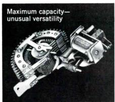
TYPE 45 ROTARY STEPPING SWITCH. Larger capacity: up to twelve 25-point levels, eight 50-point levels. For any DC voltage up to 110, or 115 volts AC with rectifier. Can be impulse-controlled or self-interrupted. Available with normally open or normally closed circuits (Type 45NC). Also available as prewired, hermetically sealed units.
