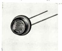
Type NSL-364C cadmium selenide photoconductive cells have chopping freqs. up to 2kc. Very low applied voltage operation is possible since the photocells have a linear voltage-current characteristic. Illuminated by a neon lamp, typical photocell resistance is 5KΩ, and dark resistance is 50 megohms minimum. Higher resistance types are also available. National Semiconductors Ltd., 2150 Ward St., Montreal 9, Canada.
