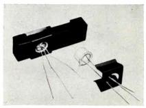
Aluminum transistor heat dissipators, numbers 10054-1 and 2, are for TO-5 transistor case sizes. The -1 unit is noninsulated, has a body finish of black anodized aluminum, and clips of Ebonal "C". The -2 unit is an insulated unit with a hard anodized black aluminum body and clips of Delcoat "B". The breakdown voltage is 350v. minimum dc on the -2 unit. The transistor is clipped into place, with no screws or bolts. Atlee Corp., 2 Lowell Ave., Winchester, Mass.
