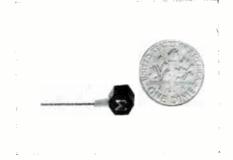
Model 2222 piezoelectric accelerometer is 0.25 in. hex x 0.20 in. high. Its light weight, 0.5 gram, permits measurement of the motion of circuit boards, components, airframe skin and other lightweight structures with negligible loading effects from its own mass. This transducer is adhesive mounted and it is optimized for operation with both charge and voltage amplifiers. Endevco Corp., 801 S. Arroyo Pkwy., Pasadena, Calif.
