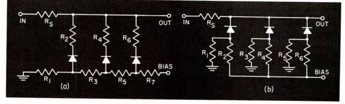
Fig. 6: Shaper circuits are used to take care of tracking across band. Circuit on left is common, while other circuit offers advantages.
