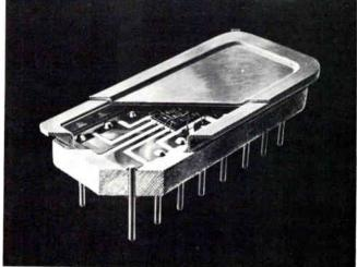
A flange tab is provided as a means of indexing. As an option, customers may specify a missing pin for positive indexing. The packages are adaptable to lowcost assembly techniques, including high-volume manual or automatic insertion, flow and wave soldering, and the use of less-expensive circuit boards with 100mil grid spacings.
