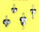
Discoidal design eliminates all parallel resonance effects at 1000 Mcps and less. Insulation resistance exceeds 100,000 megohms. Standard values: 470 mmf  $\pm$  20% and 1000 mmf GMV. Special values from 6.8 mmf to 1500 mmf. Rated to 500 v DC maximum.
