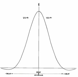
Fig. 3: Correlator output vs delay between incoming signals.
