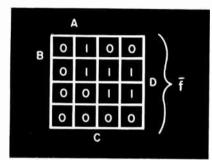
Fig. 5: Veitch diagram function plot for inverse of  $\overline{AC}$  +  $\overline{AB}$  +  $\overline{AD}$ .
