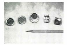
The subminiature DSM's meet and exceed the electrical and environmental performance requirements of the latest applicable Mil specs. They are available in 5 shell sizes : 3, 7, 12, 19, and 27, containing 7, 19, 37, 61, and 91 #22 contacts respectively. They have a wide range of clocking positions, and are available in sq. flange, single hole, and solder mount type mounting configurations. Pin contacts rated at 2a. Deutsch Co., Electronic Components Div., Municipal Airport, Banning, Calif.
