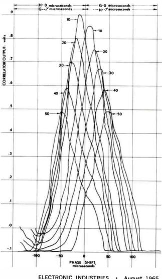
Fig. 4: Correlator output with delay au vs delay between signals in.
