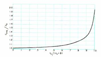
Fig. 5: Curve shows the detuning effects due to signal.
