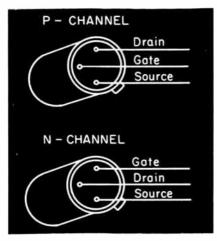
Manufacturers should adopt a standard for N-channel and P-channel configurations which are identical. I would, from a practical standpoint, like to see a center-lead location of the GATE in order to be analogous to the more common bipolar transistor types. However, I have heard arguments that "collector-to-case" headers are easier to obtain, which would then put the gate in the "collector" position. Whichever method decided upon is fine provided it will be standard for N-channel and P- channels.
