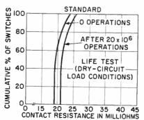
For maintaining extremely low contact resistance during prolonged life under "low level," or "dry circuit" conditions. Typical applications include low-level audio switching and
