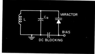
Fig. 1: A typical varactor tuned circuit that is used.
