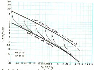
Fig. 4: Tuning range as a function of signal level limitations.
