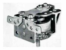
The KR3-H series relay has heavy copper-alloy movable contact arms with twin  $\frac{1}{4}$  in. dia. silver-cadmium-oxide contacts. They are rated at 20a. at 115vac 60 cycles resistive, or 28vdc; 1 HP 115/230v. 60 cycles. Its contact arrangement is 1 Form X (SPST-NO-DB). Its small size and rugged construction makes it particularly desirable for use in automation controls, communications circuits and many other uses where limited space is a factor. Potter & Brumfield, Princeton, Ind.
