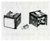
The Tec-Lite Rectangular Switch Lite, RSL Series, provide a choice of 14 different lens colors. Lenses can be hot stamped with legends in 4 different type sizes. Three available options include: Model 1. SPST normally open switch and indicator; Model 2, 2 normally open switches, DPST, and no indicator; and Model 3, an indicator only. The switch is rated 100ma at 120vac, non-inductive. Transistor Electronics Corp., Box 6191, Minneapolis, Minn.
