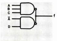
Fig. 6: Mechanization of  $f = \overline{AC} + \overline{AB} + \overline{AD}$ .
