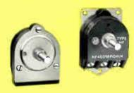
Provides higher voltage and wattage ratings for industrial and commercial electronic equipment. Quiet, stepless control. Life exceeds 100,000 com. plete cycles of operation on accelerated tests with less than 10% resist-ance change. Rated 5 watts at 40°C and 3 watts at 70°C, with a maximum of 750 volts.
