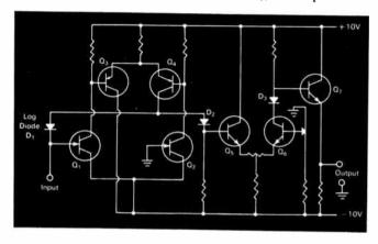
rent variation is achieved by using 2 n-channel fieldeffect transistors,  $Q_1$  and  $Q_2$  for the first differential amplifier stage. Because of the very high input impedance of these transistors, they are also sensitive to very small current.
