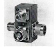
Cable faults which cause objectionable ghosts and reflection noise in TV reception are reliably detected, before cable installation, by the Model 701 Reflectometer. A bridge device, it may be used to distinguish between critical and relatively unimportant reflections caused by minor variations in impedance uniformity in the cable. Impedance is  $75\Omega$ ; balance is greater than 35db. Spencer-Kennedy Laboratories, Inc., 1320 Soldiers Field Rd., Boston, Mass.
