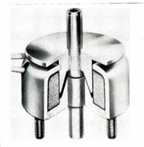
This solenoid responds in less than 10msec. at intermittent duty, and is available with conical or flat-face plungers. It is precalculated to deliver optimum performance. It uses a precision-wound coil for max. copper in minimum space. Operating voltage are 28vdc and 115vac rectified, continuous and intermittent duty. Ledex Inc., 123 Webster St., Dayton, Ohio.
