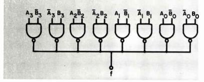
Fig. 7: Mechanization of A = B (above).
