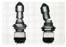
These miniature military switches feature a variety of lever lock configurations. They are available in 2- and 3-position circuit arrangements, for maintained or momentary operation, in SP-DP. The line meets all general requirements of Mil-S-8834 (Type 1). Inductive ratings are 1a. @ 28vdc and 115vac. Minimum rating for dry circuit use is 25µa @ 5mv. Other standard features include positive makebreak operation and gold-plated contacts. Cutler-Hammer, 436 N. 12th St., Milwaukee, Wisc.
