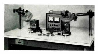
Weltek's new Model 750 can be set up in minutes to do microminiature welding, controlled soldering or "nail head" bonding. With this one piece of equipment you can solder or weld flat packs to p.c. boards, do module welding, pointto-point microsoldering or bond a wire to a transistor chip! The possibilities are unlimited. The 750 can do *all* of your miniature joining work...in the lab or in production. And it is reasonably priced.
