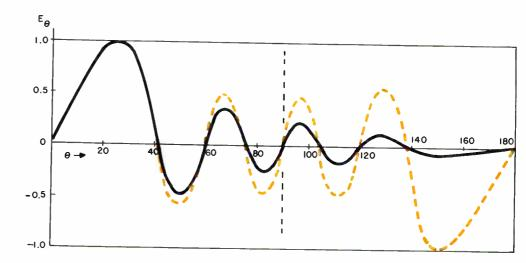
Fig. 1: Free-space normalized field-strength distributions at constant great distance from an ideal 4  $\lambda$  linear radiator with traveling-wave (--) and stand-ing-wave (+) current distributions, where  $\Theta$  is angle to wire.
