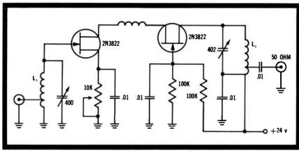
Figure 1. 200 mc cascode RF amplifier uses new T1 N-channel FET's
