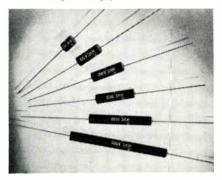
These high voltage cartridge type silicon rectifiers have avalanche characteristics which provide built-in protection against transient overvoltages. Dc ma range from 250 to 50, depending on the voltage. Max. forward voltage drop at rated current ranges from 4v. for the smaller units to 50vdc for the largest type. Sarkes Tarzian Inc., Semiconductor Div., 415 College Ave., Bloomington, Ind.
