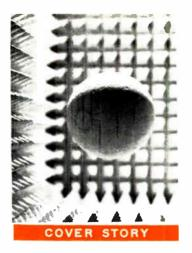
THE SPHERICALLY-SYMMETRIC LUNEBERG LENS has been applied in systems ranging from large-aperture receiving antennas to small-diameter passive reflectors (see cover photo).
