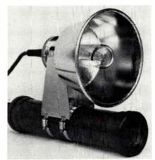
A complete underwater TV system workable down to 1300 ft. in fresh or salt water developed by Cohu Electronics, Inc., includes Cohu 2000 series miniature TV camera (above), 12" long, 3" wide, with special underwater housing. Camera has fixed-focus half-inch lens with remote focus control, plus standard vidicon. Attached is mercury vapor lamp (400w.) that can stand 5000 psi.
