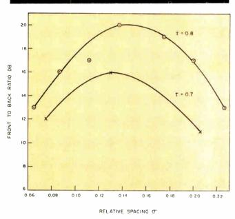
Fig. 5: Computed LP pattern front-to-back ratio vs.  $\tau$  and  $\sigma$ .
