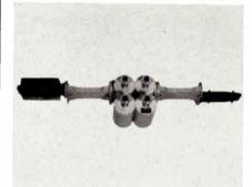
Model S4798B high-power band-pass filter is suited for radar uses where r-f interference is a problem. By preventing unwanted spurious emissions, it effectively eliminates any possible interference with neighboring radar systems. The filter displays a bandwidth ratio of less than 6 to 1 @ 60db. Freq. range is 2700-2900 MC and ripple is 0.3db max. Power capability is 1.2 megawatts peak, 4.2kw average. vswR is 1.4:1 max. Aircraft Armaments, Inc., Cockeysville, Md.
