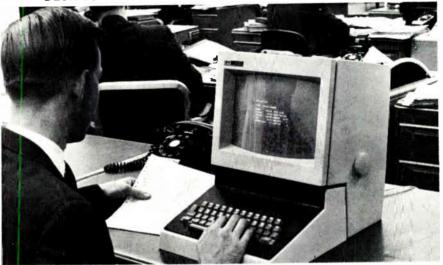
New IBM table - top device provides visual image of computer - stored information, and can help management of small and large firms maintain tight control over business activity. The 2260 can display insurance records, logs of customer calls, inventory - shipping data.
