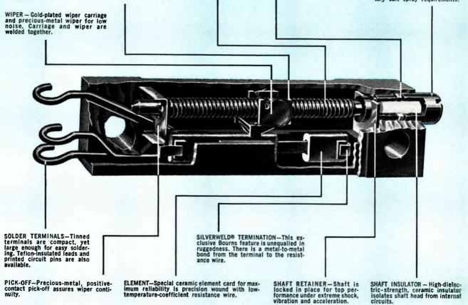
This cutaway of Model 224 shows the typical high quality to be found in all Bourns TRIMPOT potentiometers, although some features may vary from model to model.
