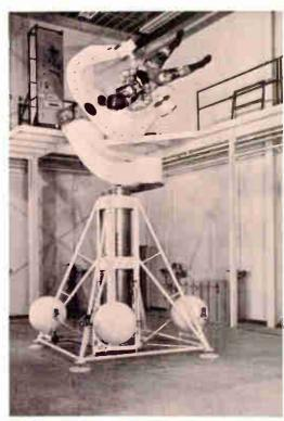
▲ FIRST MANNED TEST Manned test of "first" weightlessness simulator designed by Convair, General Dynamics. Vehicle will be used to study design needs of astronauts, orbital labs and spacecraft.
