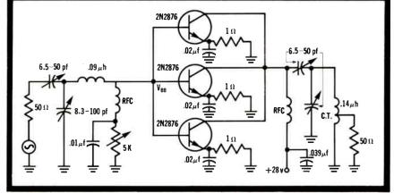
Figure 4. 30w, 50 mc amplifier uses three 2N2876 transistors (See Figure 3)
