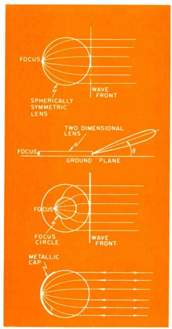
Fig. 7: Luneberg lens is a spherical lens of dielectric material.
