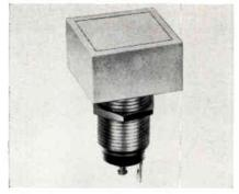
The Contempo 300 Series Square Lens indicator lights are two terminal devices. Series 301 features a 3/4 in. sq. lens, and mounts in a 7/16 in. dia. hole. It is 1-11/32 in. long. Unique feature of this series is its "push-pull" lens. The lens is "pulled" to remove, and "pushed" to install. Lens colors available are red, white, blue, green, and amber. The Sloan Co., P. O. Box 367, Sun Valley, Calif. Circle 222 on Inquiry Card
