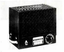
The Change-A-Cycle device uses a principle entirely different from conventional motor-generator devices. The ac input (from 25 to 400 cPs) is first rectified to dc. It is then filtered and fed to a rotary dc to ac converter which, in turn, produces either 50 or 60 cPs current. Standard units operate from single phase input and deliver single phase output. Units are available with up to 2kw outputs. Carter Motor Co., 2760A W. George St., Chicago, Ill.
