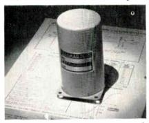
The Ultamag® 100 solid state magnetic amplifiers have high resistance to radiation. Available in either 50 or 60 CPs. They can be used in almost any application where vacuum tubes or transistors are required. Life is 10 yrs. The units provide up to 43db polarity reversible gain with 0 stability better than 1%. Power requirements are 115vac ±10%, 50 or 60 CPS. Military & Computer Electronics Corp., 900 N.E. 13th St., Ft. Lauderdale, Fla.
