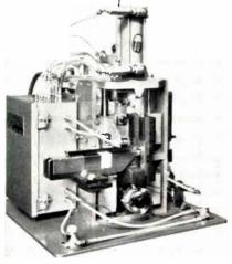
Model PCR-20 Automatic Coil Retainer Inserting Machine allows 1 operator to insert the coil retainer, stamp identifying numbers, secure the leads, and perform the final forming of the end turns at rates of up to 400 fields/hr. Designed for both machine wound and hand inserted fields, it handles stack dia. up to 6 in. and stack heights up to  $3\frac{1}{2}$ in. The standard machine uses preformed coil retainer material. Possis Machine Corp., 825 Rhode Island Ave. So., Minneapolis, Minn.
