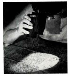
Can see objects clearly in pitch darkness. Unit, developed by ITT, is self - contained device that converts infrared to visible light with a special tube — a high - resolution converter. Will be used by military, for law enforcement, and in industry, such as in dark-room inspection of processing film.
