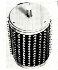
Model 205S contains 13 pot gangs. This film potentiometer functions as a precision voltage divider with multi-increment fixed voltage taps. The same pot can also be used to custom shape nonlinear functions (experimentally) until the precise, desired function is obtained. With excitation applied to the wiper, it provides multiple gating signals. Terminal resistance is  $120K\Omega$ . Computer Instruments Corp., 92 Madison Ave., Hempstead, L. I., N. Y.
