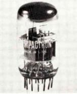
The 9BJ11 Compactron offers sensitivity equal to some 3-stage amplifiers. It can lower costs, improve performance levels, and conserve space in the manufacture of monochrome TV receivers. Construction features of the input section eliminate the need for a gain-robbing unbypassed cathode resistor. It provides high transductance and low capacitance in each section. High-input impedance unloads the mixer stage for improved tuner gain. General Electric Co., 3800 N. Milwaukee Ave., Chicago, Ill.
