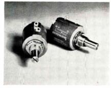
Model 3500 is  $\frac{7}{6}$  in. dia., bushing mount 10-turn unit. All-sealed construction ensures Mil-spec resistance to humidity. Silverweld® terminations, a fused bond between the terminal and resistance wire, eliminates fragile, single-wire termination. Resistance tolerance is  $\pm 3\%$ ; linearity is  $\pm 0.20\%$ . Withstands vibration of 20G and shock of 100G. Bourns, Inc., 1200 Columbia Ave., Riverside, Calif.
