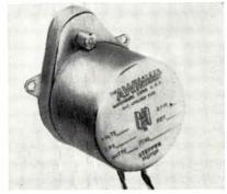
Series 44600 rotation is unidirectional, either clockwise or counterclockwise, as required. The rotor shaft rotates in discrete 15° steps, and at rates up to 4800 steps/min. Positive magnetic detenting occurs at each of 24 angular rotor positions. Stepping action is obtained by applying dc pulses alternately to 2 stator coils. Operating voltage is 27vdc  $\pm 10^{\circ}$ in standard models. The A. W. Haydon Co., 232 N. Elm St., Waterbury, Conn. Circle 242 on Inquiry Card
