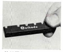
Model TB-809 WS is a 9-contact bussing connector. It is expected to be used in communications, data acquisition and transmission equipment. The connector mounts through 0.051 dia. holes. Jumper bars are available for bussing between any pair of contacts. Insulation is glassfilled diallyl phthalate. Connector measures  $2\frac{3}{8} \times 0.340 \times 7/16$  in., not including terminals. Methode Electronics, Inc., 7447 W. Wilson Ave., Chicago, Ill.
