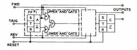
Fig. 2: Equivalent circuit for on-off condition. Fig. 3: The 3-stage reversible counter logic diagram.
