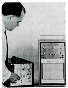
Full - floating, 500  $\mu$ v. level, high - voltage dc preamplifier that accepts microvolt level signals up to 1000v off - ground on low - level channel, or a potential difference up to 1000v dc. on high level has been developed by Brush Instruments, Clevite Corp. Amplifier, recorder and system monitored are all protected by current limiters and over - voltage devices. Unit insures noise-free operation.
