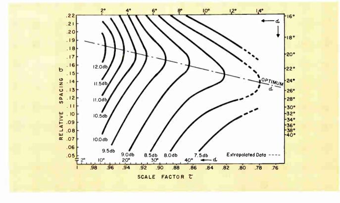
Fig. 4: Computed log-periodic contours of constant directivity (D) vs  $\tau$ ,  $\sigma$ , and  $\alpha$ .
