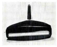
The SC-3800 is designed for grounded anode voltage circuit uses only. The fiber optics strip has an approx. active area  $8\frac{1}{2}$  in. long x 5/16 in. wide. The electron optical system and fine grain screen achieve a very fine trace width using conventional focusing and deflection units. Electronic Tube Div., Sylvania Electric Products Inc., Seneca Falls, N. Y.
