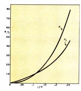
Fig. 3 (left): R and X<sub>1</sub> of a linear antenna.
