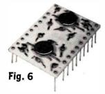
The most recent chapter of the CERMET story has been written by a family of CTS CERMET hybrid integrated circuits which provide the basic building blocks for digital logic functions. The dual flip-flop. (Fig. 6) has 14 diodes and 4 transistors on the upper side and 20 CERMET resistors, 4 CERMET capacitors, a CERMET lead crossover, and a CERMET conductive network on the under surface. A dual nand gate, a bistable flip-flop, a one shot multi-
