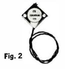
The reliability and the stability of CERMET films has been confirmed by the use of CTS CERMET trimmers, (Fig. 2) in electronic pacemakers inserted into the bodies of heart disease patients.
