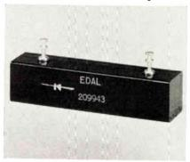
The Series N cold case silicon packages eliminate soldering many diodes to achieve equivalent circuitry. Available in full-wave, half-wave, doubler, center tap, open bridge and 3 phase types. Units consist of matched, pre-tested, pre-selected, double diffused avalanche rectifiers, self-protected against voltage transients. Standard types offer voltage ratings from 1500 to 30Kv PIV, with currents from 20ma to 6a. Edal Industries, Inc., 4 Short Beach Rd., East Haven, Conn.
