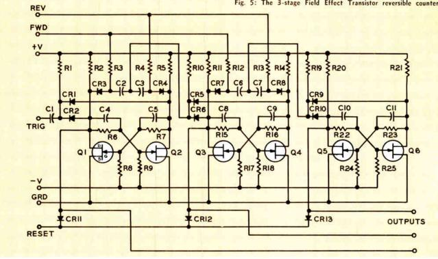
Fig. 5: The 3-stage Field Effect Transistor reversible counter.
