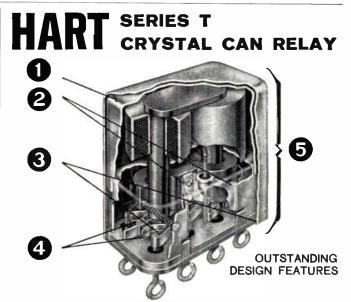
Hermetically Sealed Coil prevents contact contamination; seals organic coil material from switch section. 2 Unique Hinge Design—no pivot or bearing problems; free from wear particles. 3 Welded Construction increases reliability of joints; further reduces contamination. 4 Bifurcated Contacts increase low level switching reliability. 5 Improved Sensitivity —100 MW or less at pull-in.
