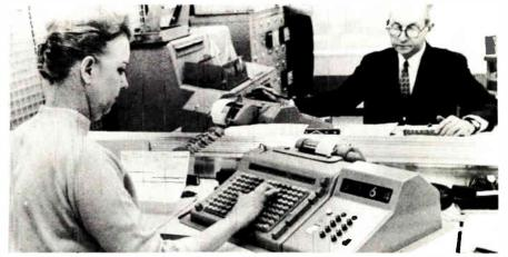
Desk digital computer, developed by Digital Electronics, Inc., instantly checks authenticity of messages in inter - bank activity, now in use at Chase Manhattan Bank, New York. Each computer can index up to 999 identity numbers for member or corresponding banks.
