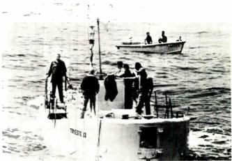
Bathyscaph TRIESTE II for underwater search. Electronic equipment aboard includes: cameras, Xenon strobe flash, side-looking sonar.
