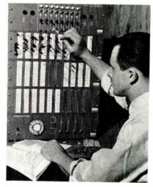
Desk - top Digital Laboratory System introduced by Digital Equipment Corp., is described as versatile digital - logic training device and design tool. It allows student or designer to build an operating system, complete with logic elements, power supply, controls, indicators and mounting hardware.
