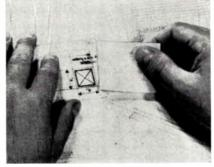
This backing sheet will be used on all Stanpat preprinted repetitive symbols and drawing details. The backing sheet lays flat regardless of atmospheric conditions. It is transparent, allowing draftsmen to position the Stanpat before application to drawing. Without any change to the adhesive, both sides of the sheet are now sealed to prevent any absorption of moisture. Stanpat Products Inc., Whitestone, N. Y.
