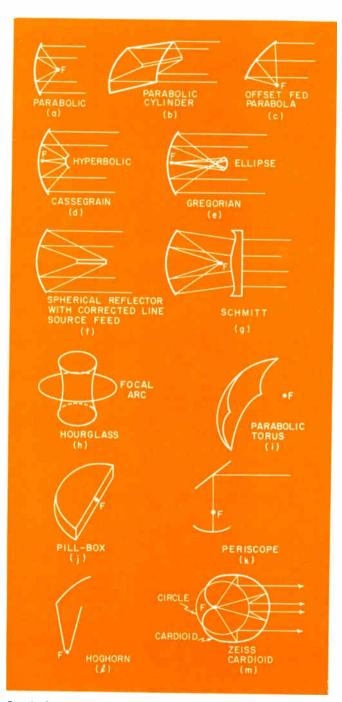
Fig. 1: Some of the possible antenna reflector forms.
