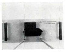
The EECO 5000 Photoblock Readers can control any automated punched tape programmed system. Typical uses include automatic test equipment, ground support systems, machine tool control, and manufacturing process control. Each signal output is capable of switching up to 100ma from either plus or minus logic levels, or from relay loads depending upon output option selected. The unit has no clutch, brake or pinch rollers. Electronic Engincering Co. of Calif., 1601 W. Chestnut Ave., Santa Ana, Calif.
