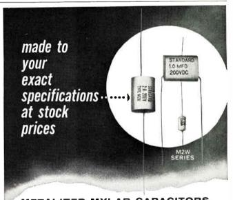
**METALIZED MYLAR CAPACITORS** Unique, self-healing units that remain in circuit during voltage surges with little or no loss of electrical properties. Use the M2W's where size and weight are limiting factors and long life and dependability are required. The units utilize metalized Mylar\* Dielectric with film wrap and custom formulated epoxy resin end fill. Available in round and flat styles.
