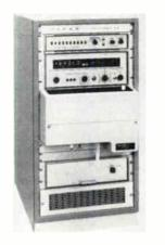
The Vidar 5100 offers microvolt sensitivity on the lowest range. It makes lowlevel measurements directly without further amplification. The system is floated and guarded from power-line ground with a common mode rejection of 160db at all freqs. The system integrates digital voltmeter, high-speed paper-tape printer, and a system coupler. Channel identification, polarity, 5 digits of data, and range are printed at a max. rate of 600 channels/ min. Vidar Corp., Mountain View, Calif.
