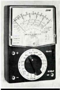
Handy, pocket size providing a meter movement of 35 microamperes in sensitivity.
