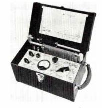
The type A Groundometer features a transistor operated 1-f bridge power source. It uses a synchronous meter detector to eliminate stray ac and dc ground currents. Full scale ranges are 1-10-100-1K and  $10K\Omega$ . It is used for measuring the resistance path of grounding electrodes for lightning arrestors, transformers, relays, transmission line towers, telephone and telegraph equipment, etc. Industrial Instruments Inc., Borden Engineering Div., 89 Commerce Rd., Cedar Grove, N. J.
