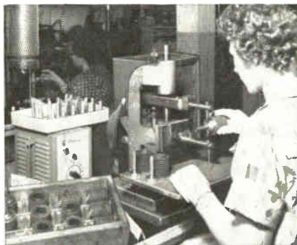
Below: An Eisler precision vertical Spot Welder designed exclusively for welding electronic components. Sizes from 1/2 to 7 1/2 KVA
