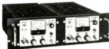
Two Trygon HR20-1.5's, rack-mounted side by side.
