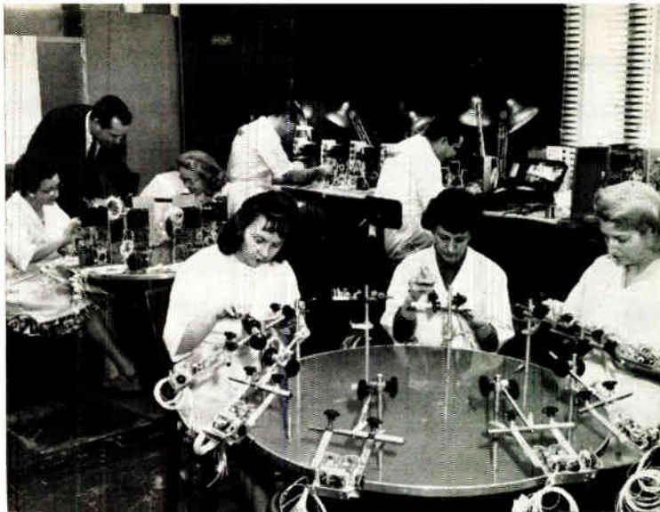
To insure reliability for orbiting spacecraft, Aerojet-General Corp. developed its Microwelder to link micro-size components after discovery that standard bonding devices would not produce needed reliability. Workers here are producing Microwelder components.
